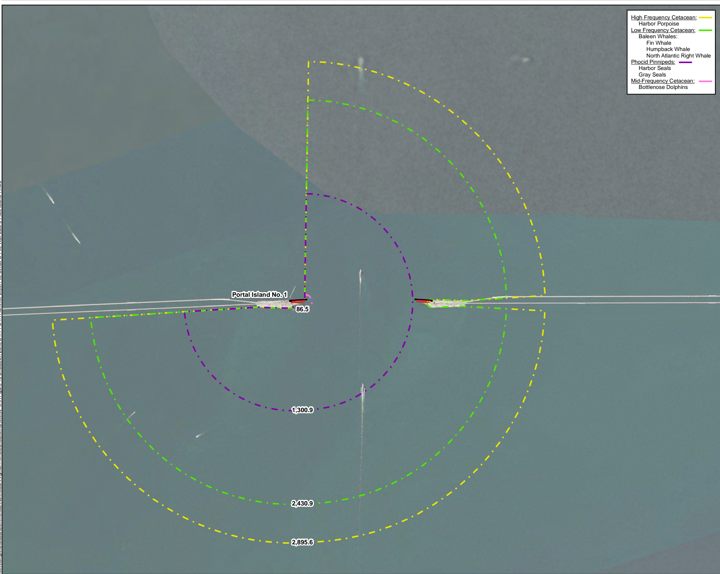
Figure 6 Distance (meters) to Shutdown Zone Using Two Down-the-Hole Hammers for Simultaneous 36- and 42-in Steel Pile Driving for the East O-Pile Wall – 6 Piles per Day at Portal Island No. 1 Marine Mammal Protection Act Parallel Thimble Shoal Tunnel
