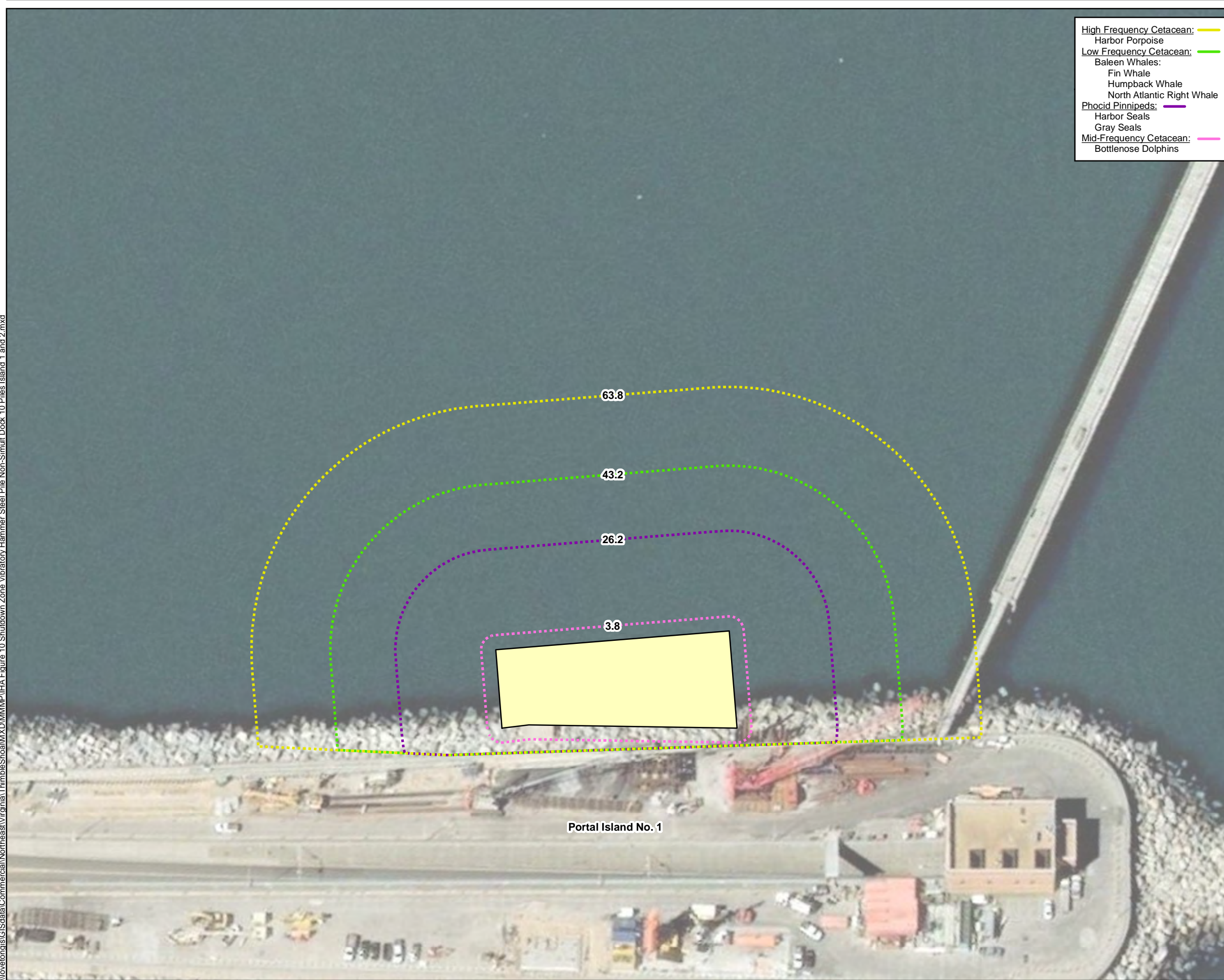
Figure 3 Distance (meters) to Shutdown Zone Using a Vibratory Hammer for Non-Simultaneous 36- and 42-in Steel Pile Driving for the Temporary Dock – 10 Piles per Day at Portal Island No. 1 Marine Mammal Protection Act Parallel Thimble Shoal Tunnel
