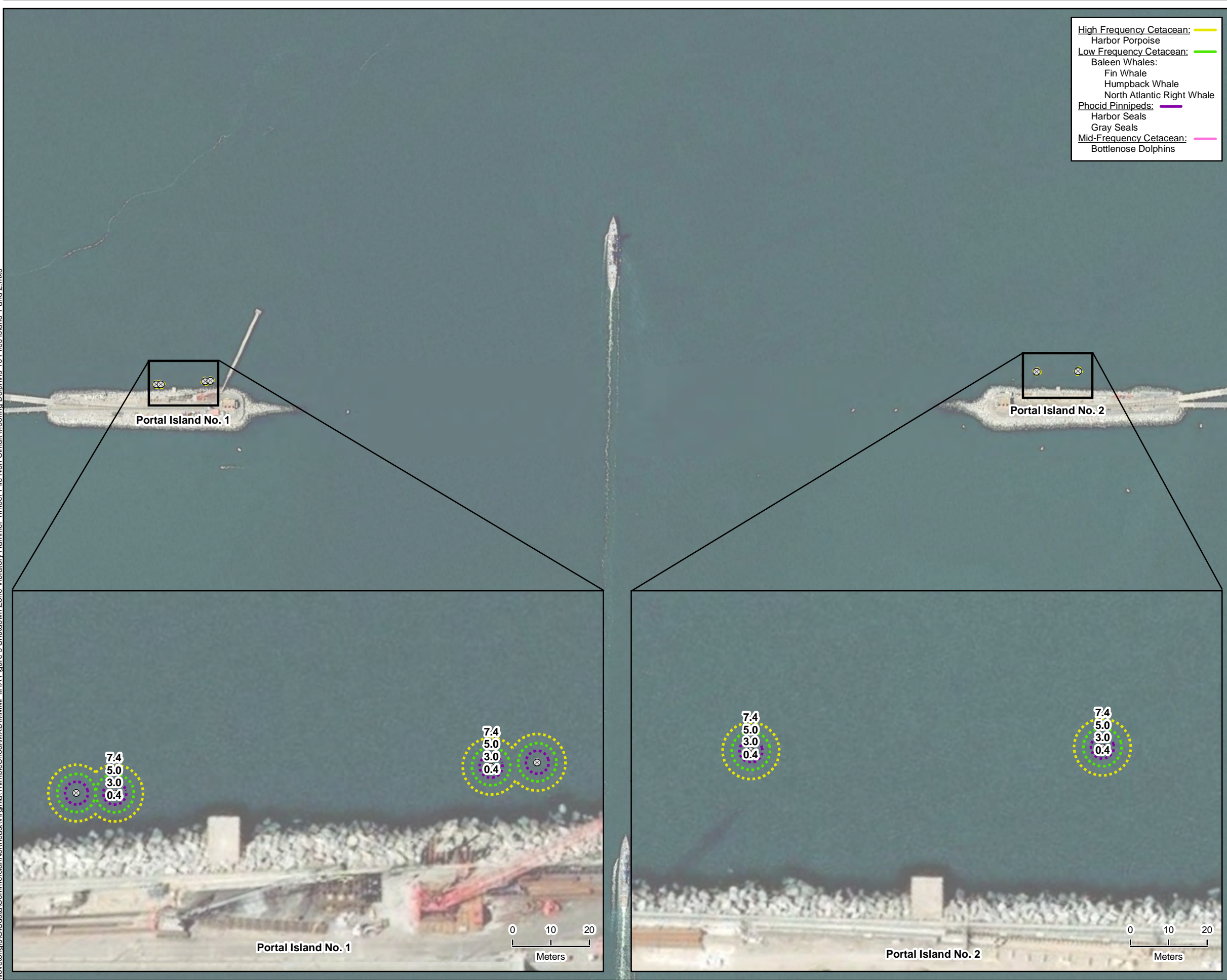
Figure 2 Distance (meters) to Shutdown Zone Using a Vibratory Hammer for Non-Simultaneous Timber Pile Driving for the Mooring Dolphins – 10 Piles per Day at Portal Island Nos. 1 and 2 Marine Mammal Protection Act Parallel Thimble Shoal Tunnel
