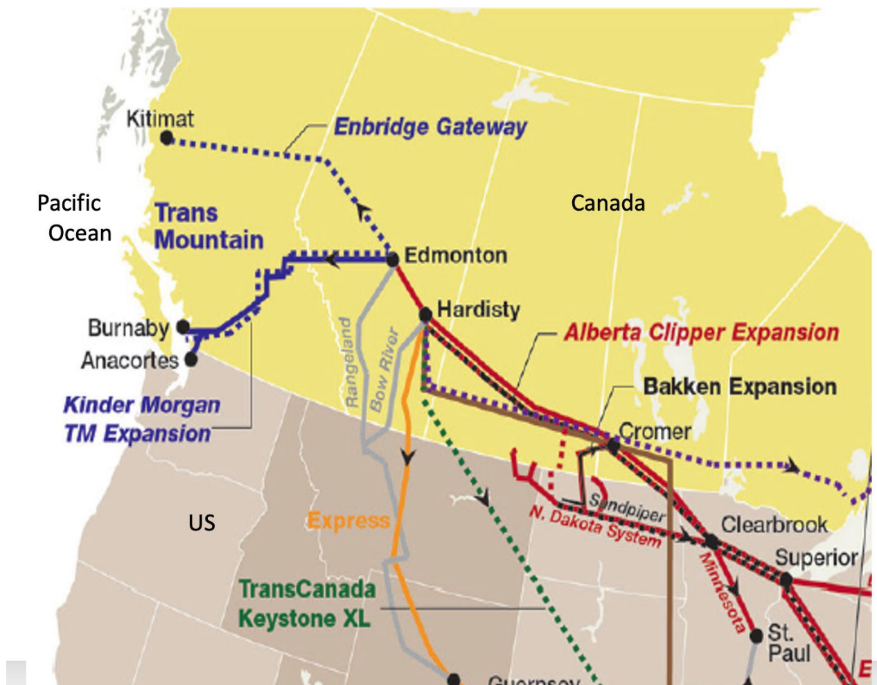
Figure 4. Map showing the pipeline distribution of for oil including dilbit. Two endpoints for Kinder Morgan expansion are at Burnaby, B.C., Canada and Anacortes, WA, USA with dilbit scheduled to be transported by ships through the tidal straits of the Central Salish Sea. Modified after NASEM (2016) .
