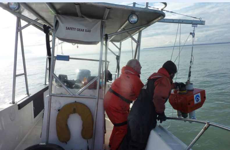
Marine Mammal Laboratory staff deploy acoustic recording equipment in Cook Inlet to detect belugas and measure anthropogenic noise levels. Credit: Verena Gill, NMFS
