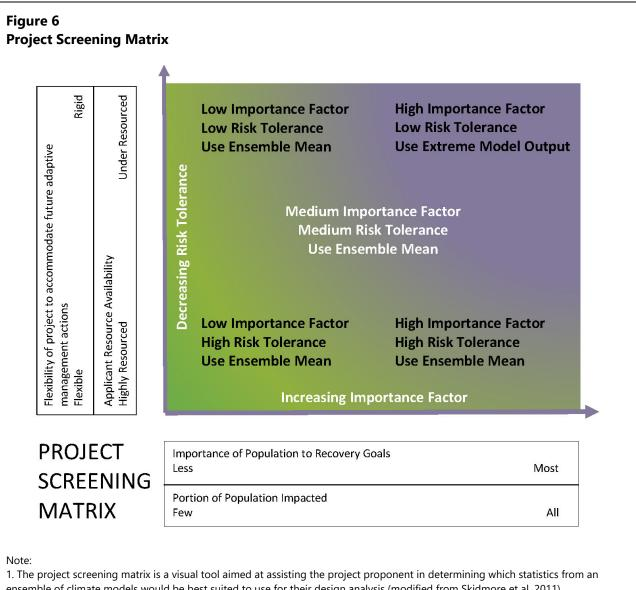
The project screening matrix is a visual tool aimed at assisting the project proponent in determining which statistics from an ensemble of climate models would be best suited to use for their design analysis (modified from Skidmore et al. 2011).
