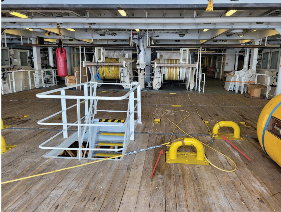
Figure 5: Second and third Chinese fingers connected to the pad eyes on the streamer deck and some loose cable on the deck for extra when moving the cable if needed.
