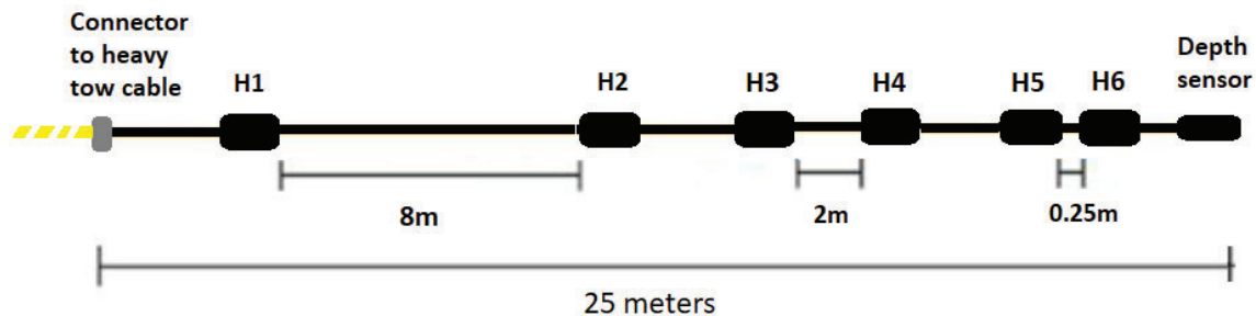
Figure 1: Schematic diagram of the hydrophone array cable indicating the position and separation of individual hydrophone elements and hydrophone pairs.
