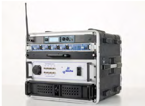
Figure 3: Electronic 8U base unit including PC and LF and HF monitors
