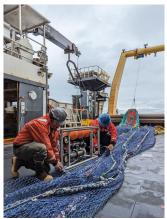
Top: Deployment of a trawl-resistant echosounder mooring to evaluate movement of pollock into, and out of, the U.S. EEZ.
