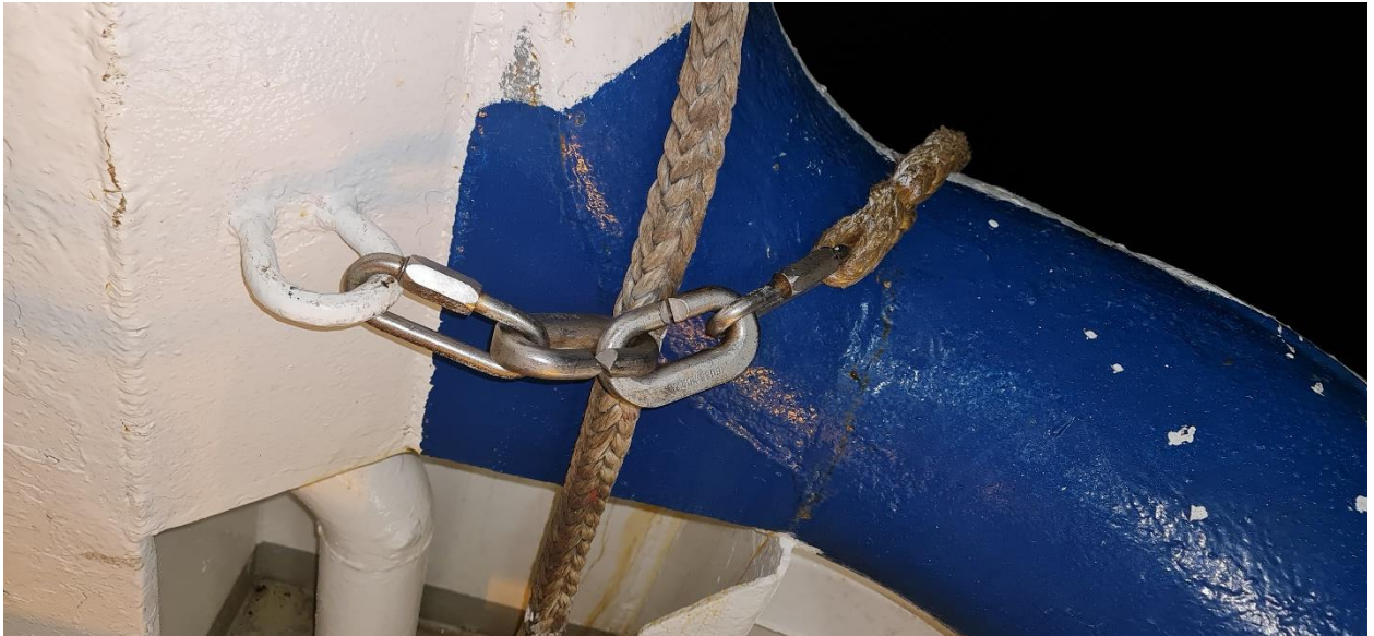
Figure 55. tension rope with G-link in stored position off Streamer deck.
