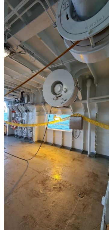
Figure 50. Starboard winch utilized for main PAM cable.
