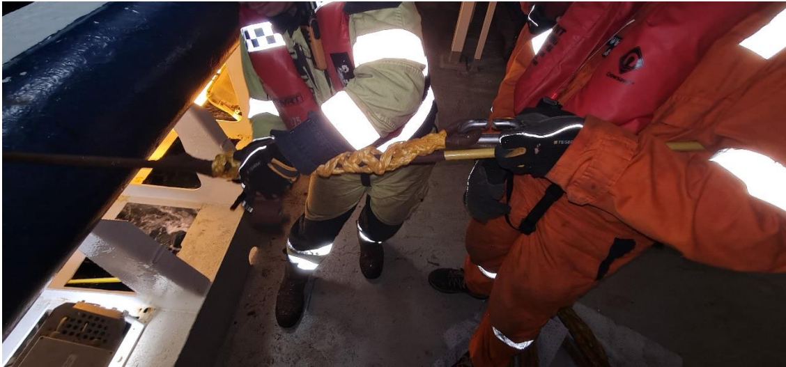
Figure 53. Chinese fingers being attached to tow cable.
