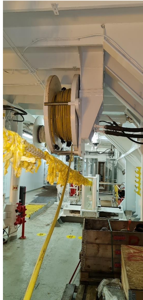
Figure 61. Incorrect cable deployment.
