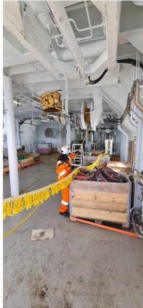
Figure 51. Starboard side main PAM cable being spooled onto winch.
