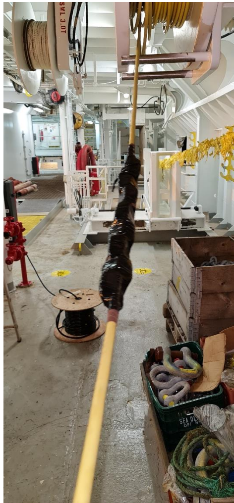
Figure 52. Starboard side main PAM cable being spooled onto winch.
