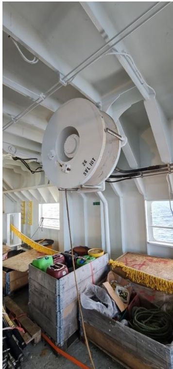
Figure 49. Port winch utilized for spare PAM cable
