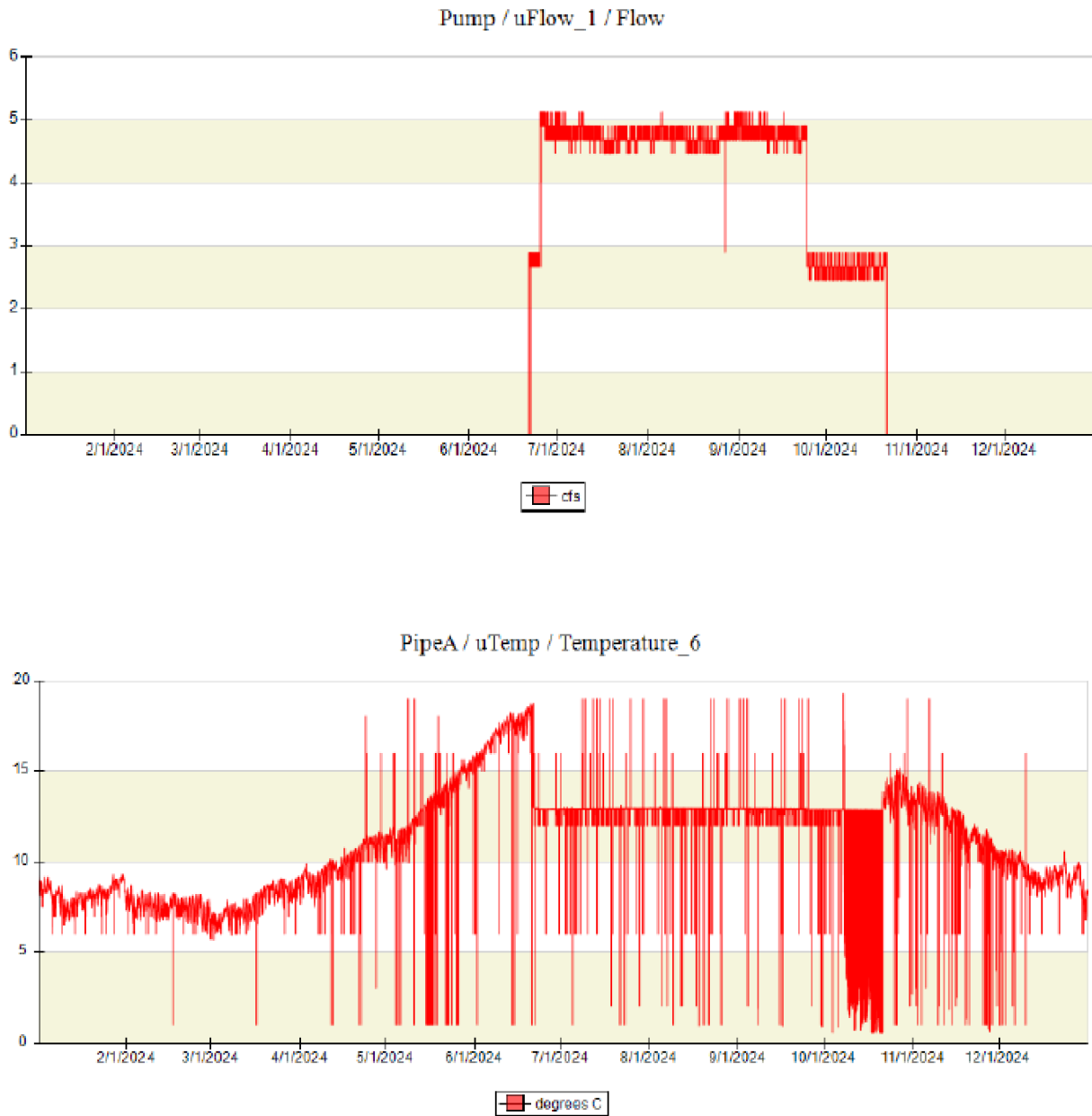
Figure 2 - Flying L Groundwater Contribution for 2024 in cfs in the first graph, showing pumping rates at 5 cfs between July through end of September, dropping to 3 cfs in October. The second graph shows temperature recorded from the pipeline delivering water from well to cold water habitat- Temperature of water released is generally a consistent 15 degrees C.
