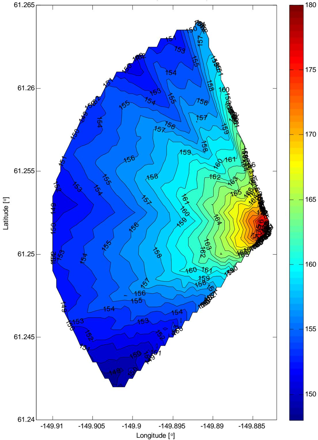
**Figure 52. Isopleths from Instantaneous Peak Pressure with Smoothing Window Size of 9 (Impact, Sheet Pile, Deep Hydrophone)**
