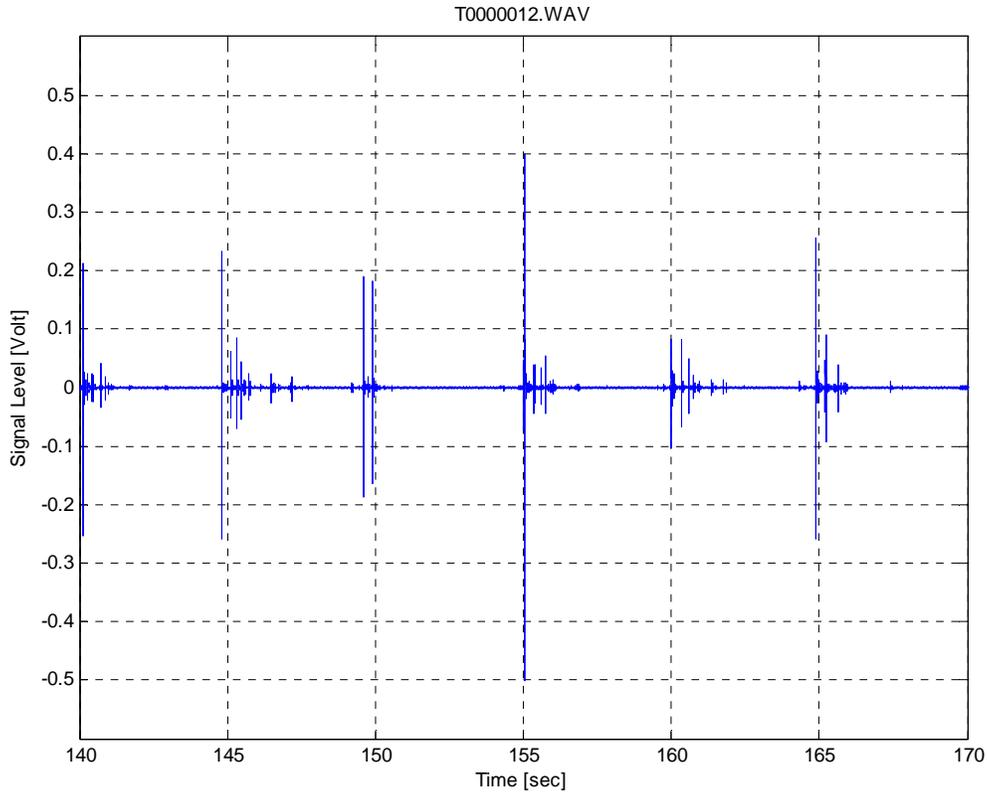
Figure 71. Raw Time Series of Worst Case Impact Pile Driving (Impact, Hairpin)
