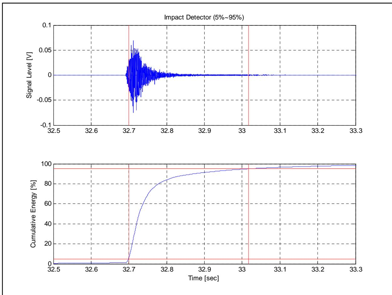
**Figure 3. An Example of Impact Detection and Pulse Duration**
