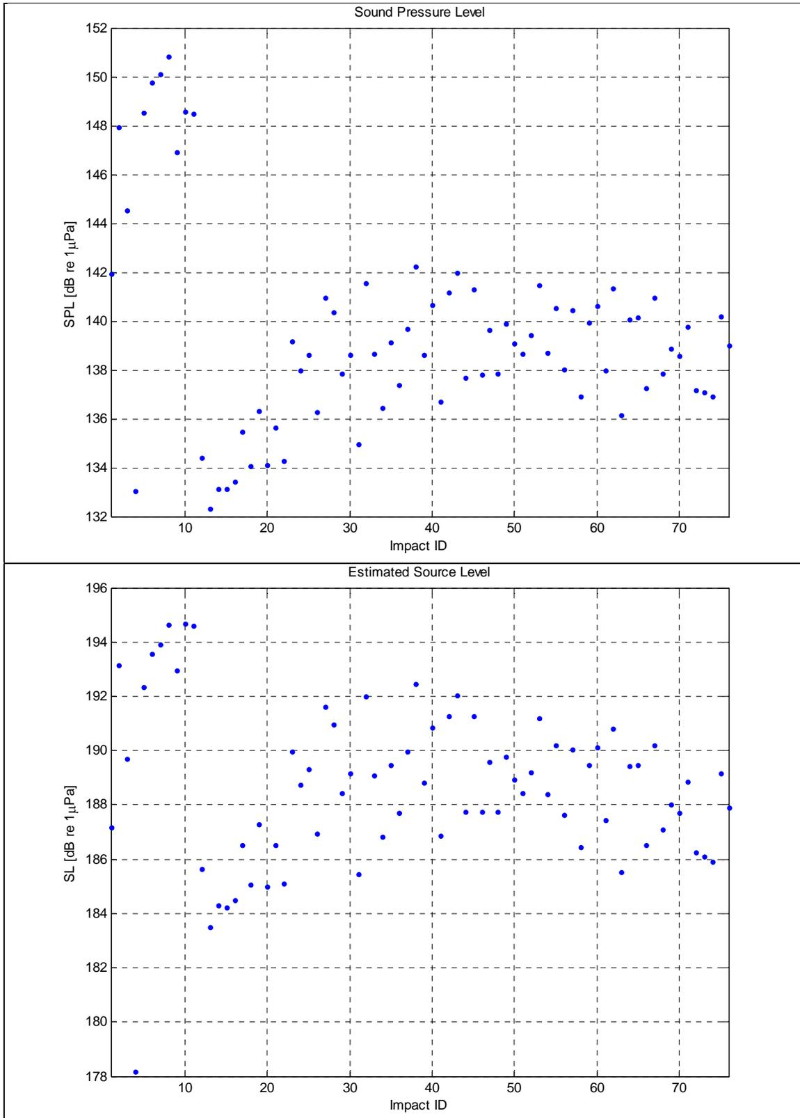
Figure 56. Sound Pressure Level and Estimated Source Level (Impact, Wye-Pile)
