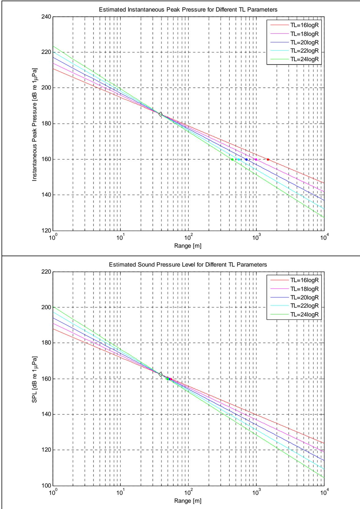
Figure 77 (e). Consideration of Different Transmission Loss Configuration for Impact ID 5
