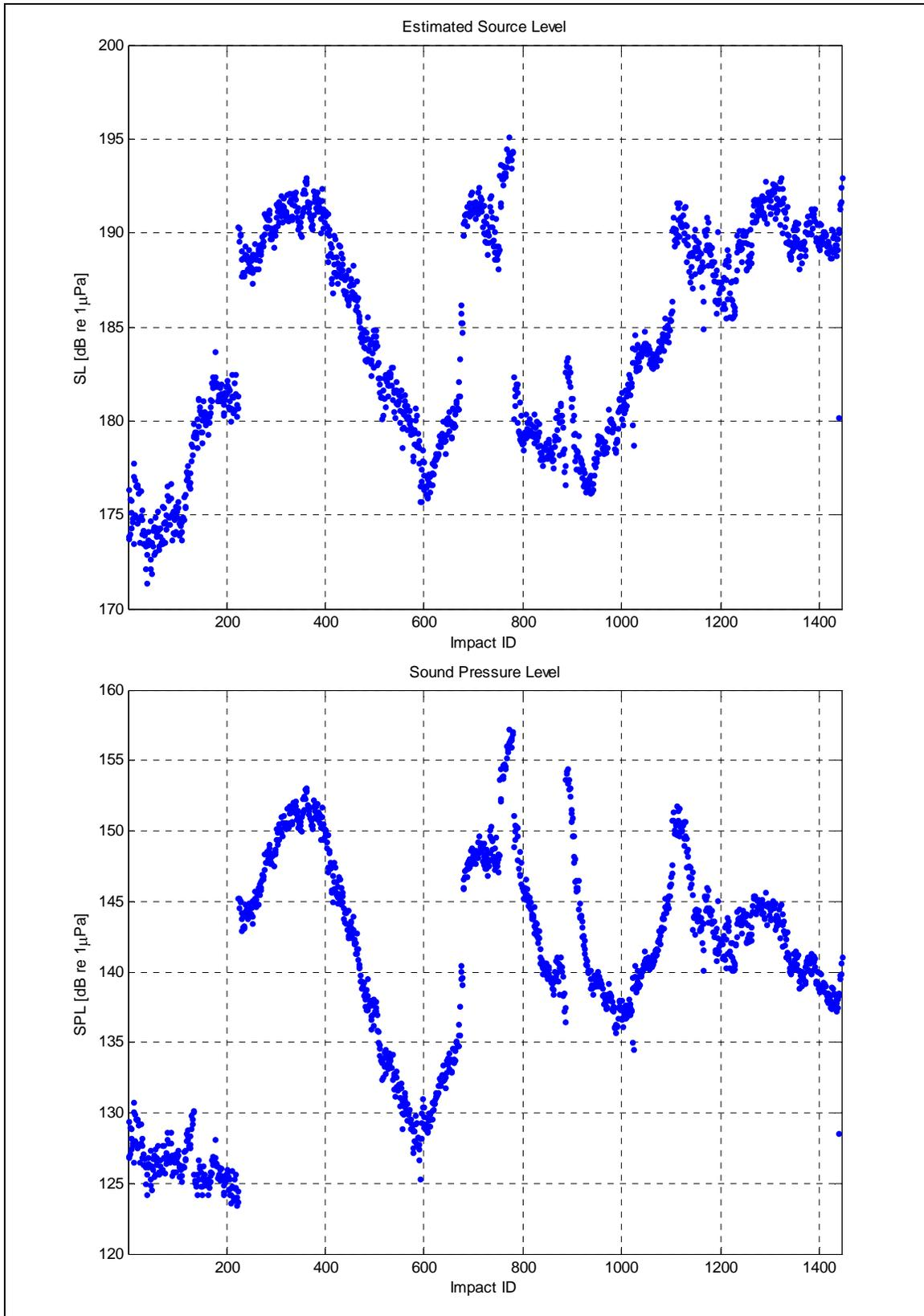
**Figure 32. Sound Pressure Level and Estimated Source Level (Impact, Sheet Pile, Shallow Hydrophone)**
