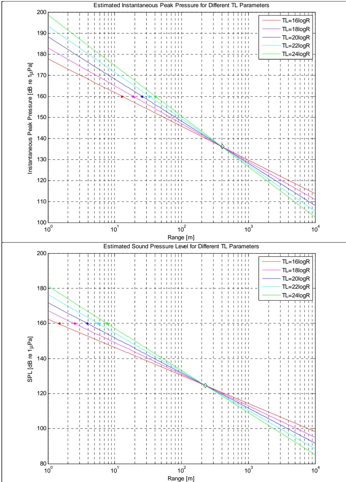
**Figure 94. Consideration of Different Transmission Loss Configuration (Hand Hammer)**
