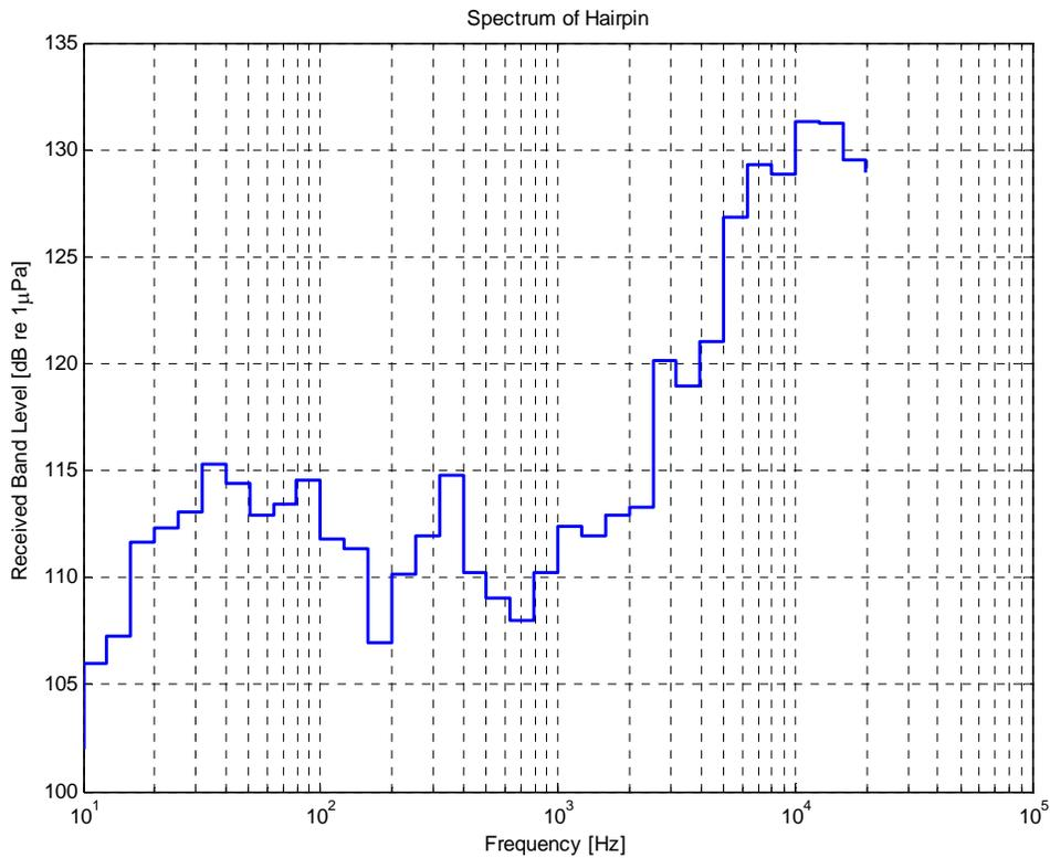
Figure 72. One-Third Octave Spectrum for Pile Driving (Impact, Hairpin)
