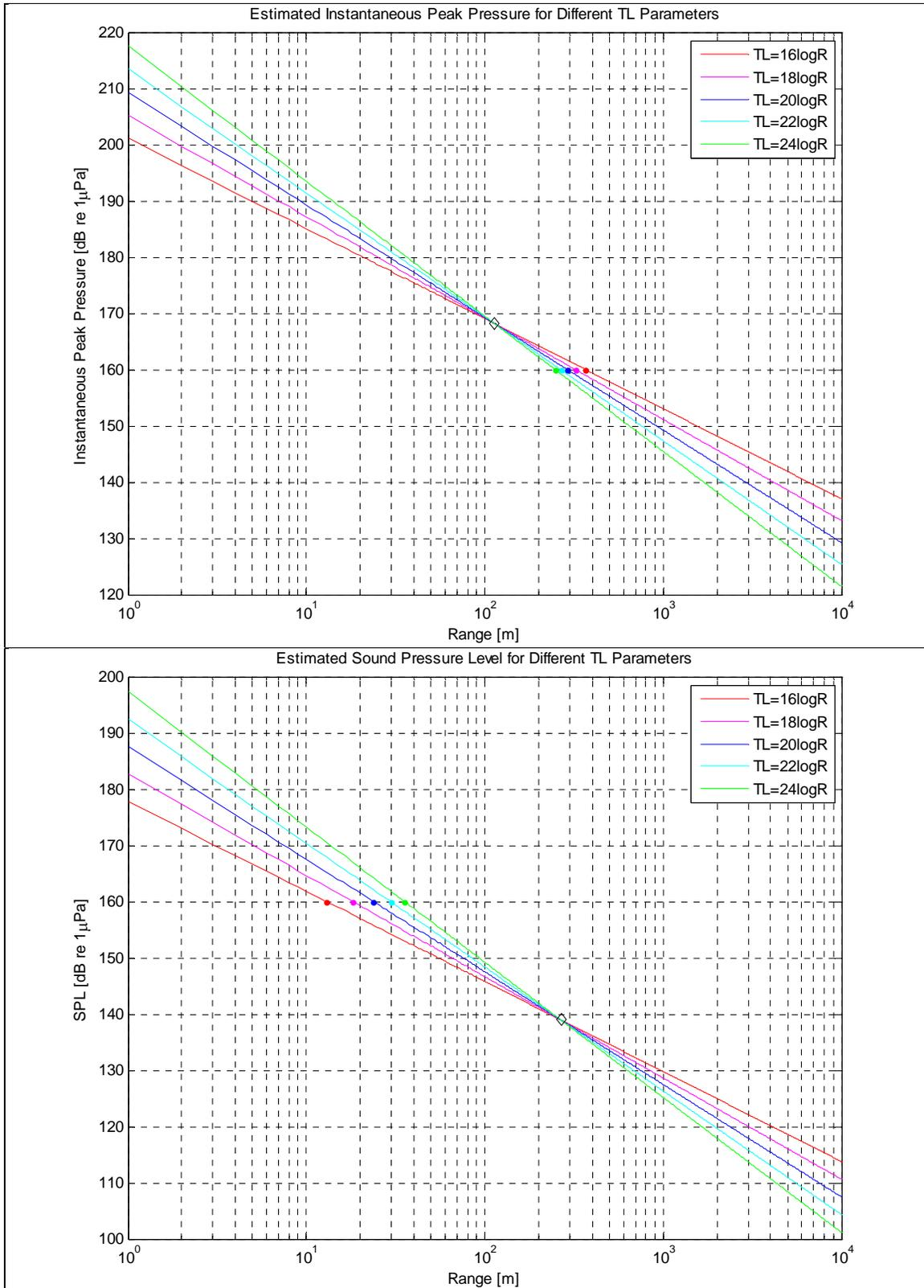
**Figure 68. Consideration of Different Transmission Loss Configurations (Impact, Sheet Pile – Tail Wall)**
