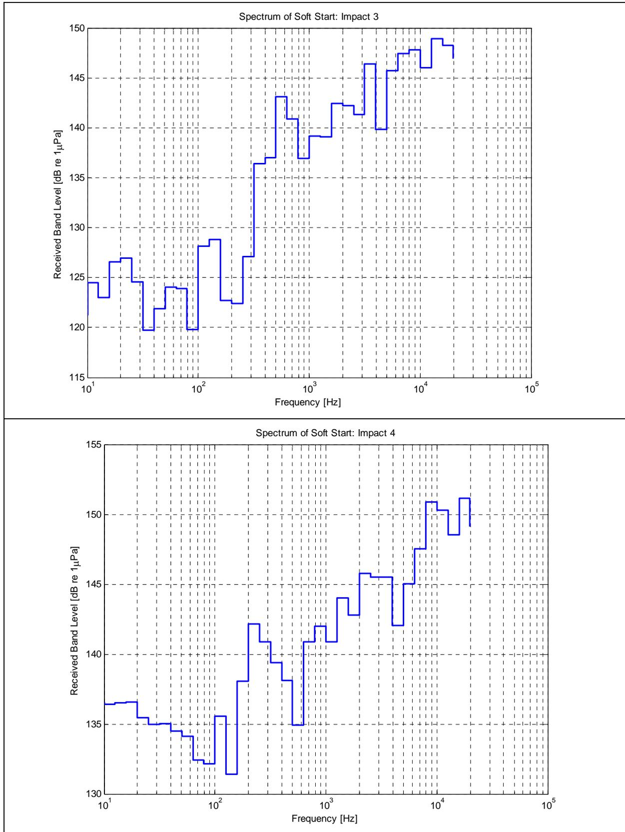
Figure 76 (b). One-Third Octave Spectrum for Pile Driving (Impact, Soft Start)
