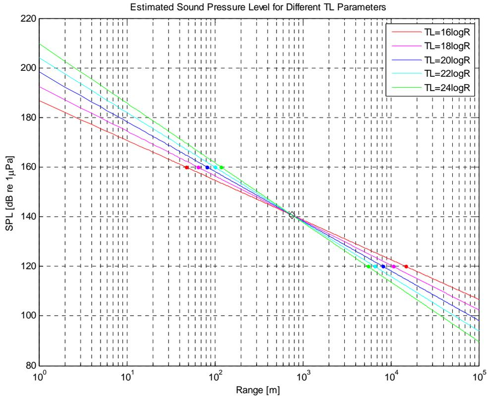
**Figure 10. Consideration of Different Transmission Loss Configuration, Vibratory Sheet Pile Driving**
