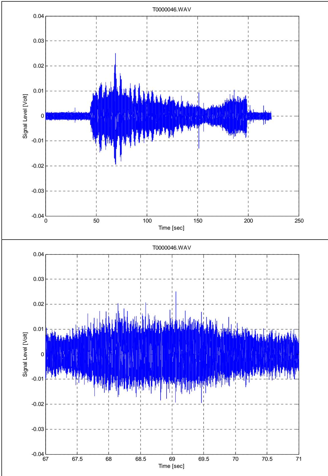
Figure 8. Raw Time Series of Pile Driving (Vibratory, Sheet Pile)
