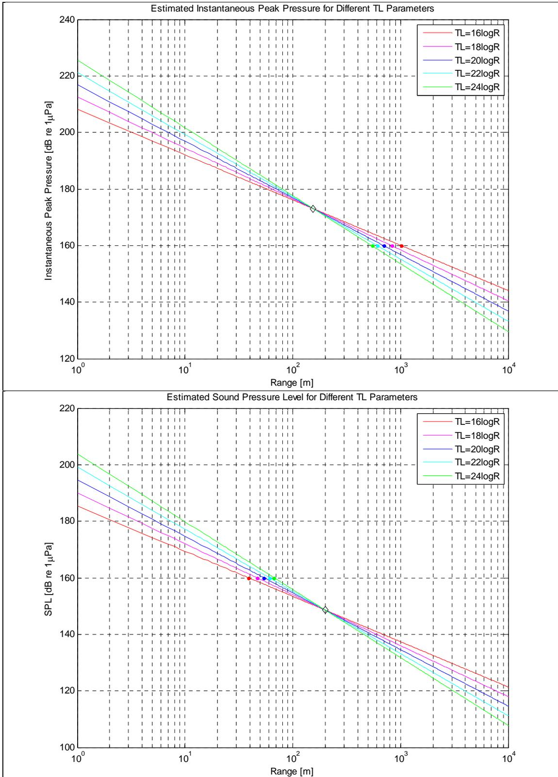
Figure 61. Consideration of Different Transmission Loss Configuration (Impact, Wye-Pile)
