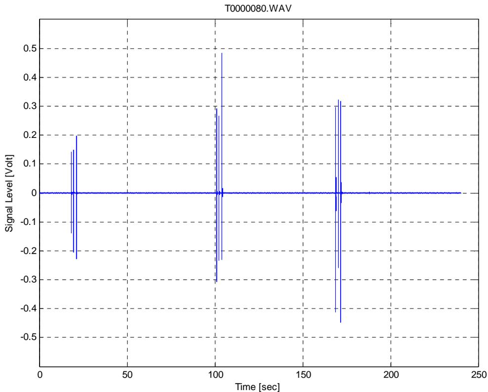
**Figure 75. Raw Time Series of Soft Start Impact Pile Driving (Impact, Soft Start)**
