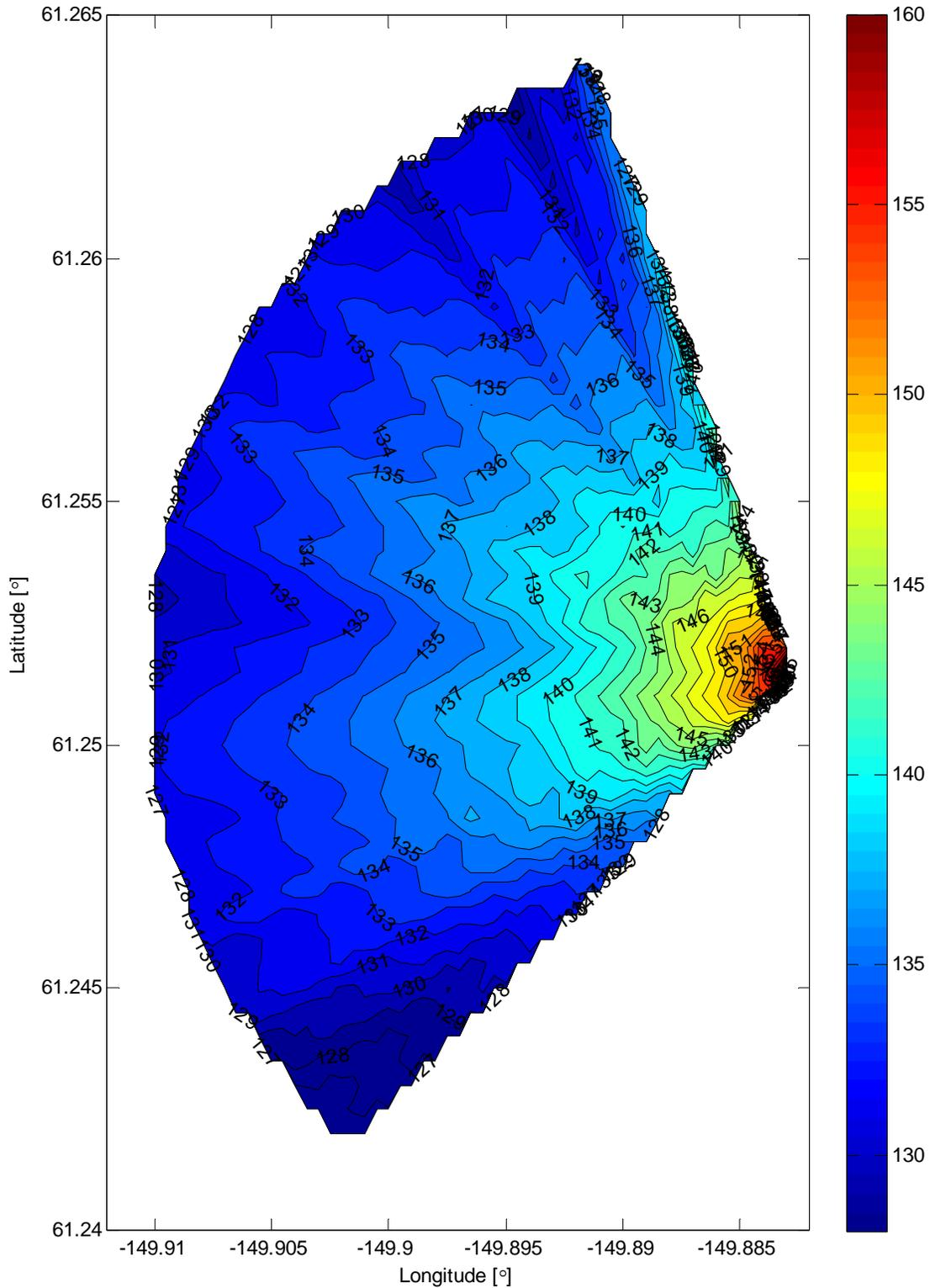
Figure 53. Isopleths from Sound Pressure Level with Smoothing Window Size of 5 (Impact, Sheet Pile, Shallow Hydrophone)
