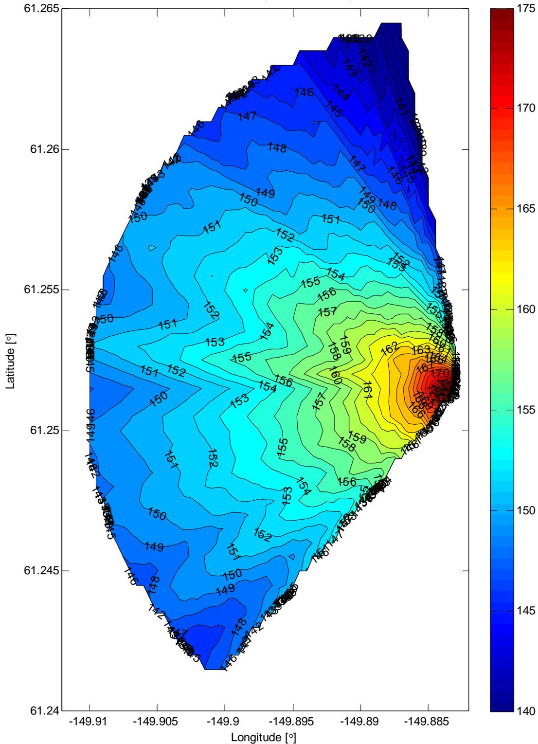
**Figure 40. Isopleths from Instantaneous Peak Pressure with Smoothing Window Size of 9 (Impact, Sheet Pile, Shallow Hydrophone)**
