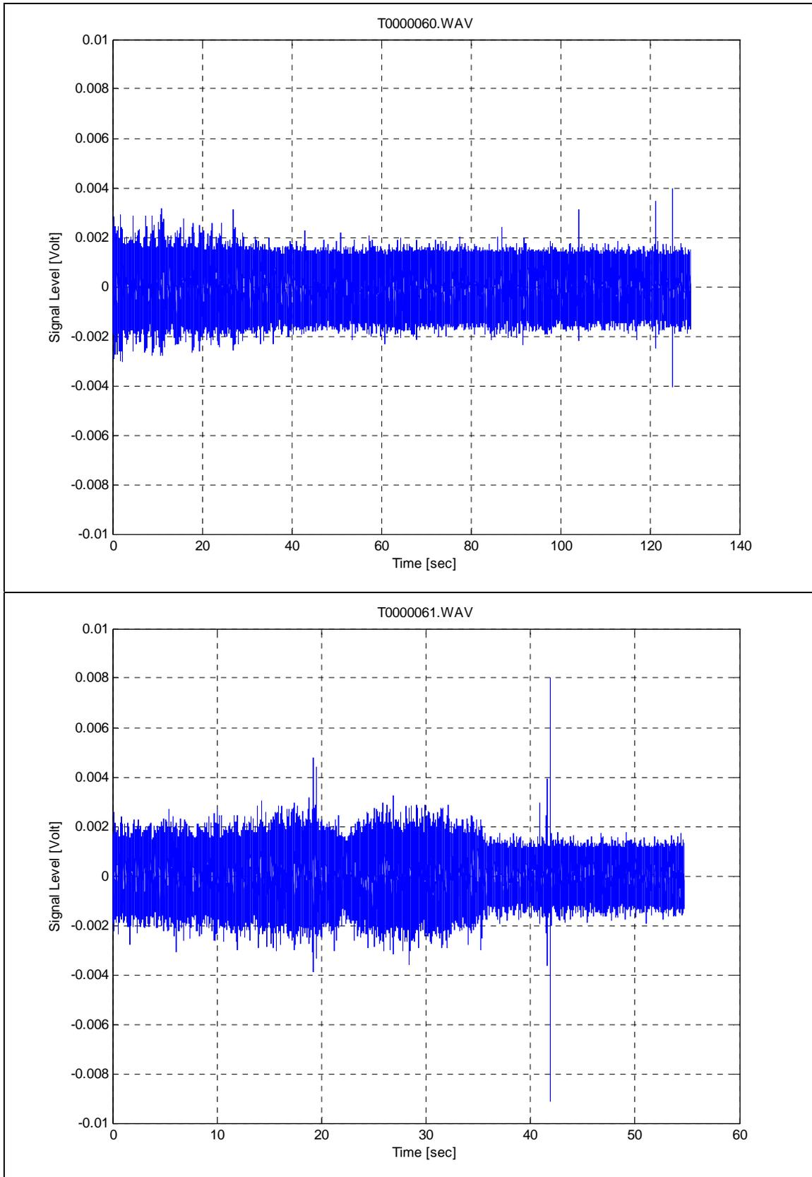
Figure 28. Raw Time Series of Pile Driving (Vibratory, Sheet Pile – Tail Wall)
