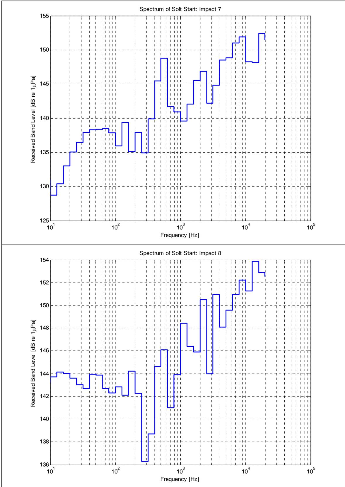
Figure 76 (d). One-Third Octave Spectrum for Pile Driving (Impact, Soft Start)
