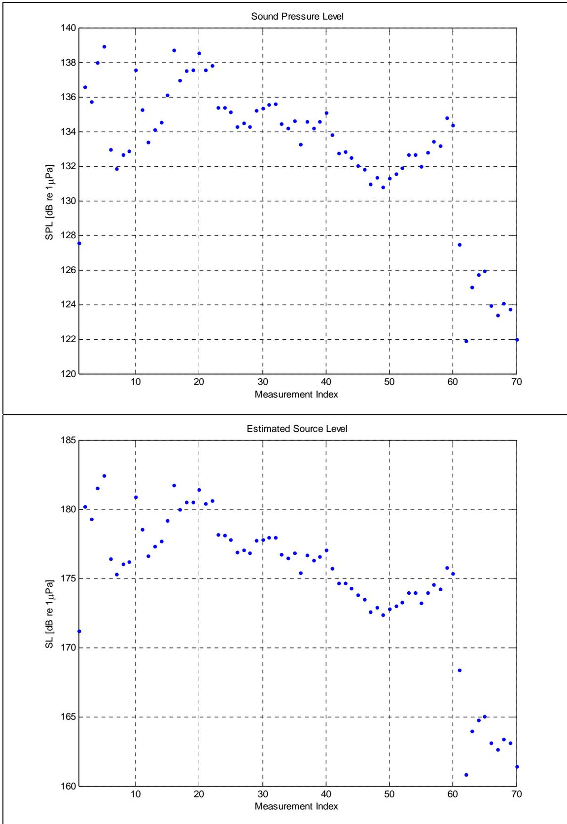
Figure 12. Sound Pressure Level and Estimated Source Level (Vibratory, Wye-Pile)
