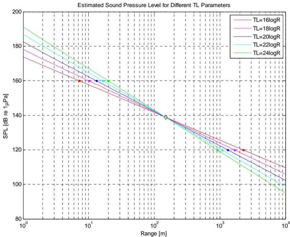
Figure 17. Consideration of Different Transmission Loss Configuration (Vibratory, Wye-Pile)
