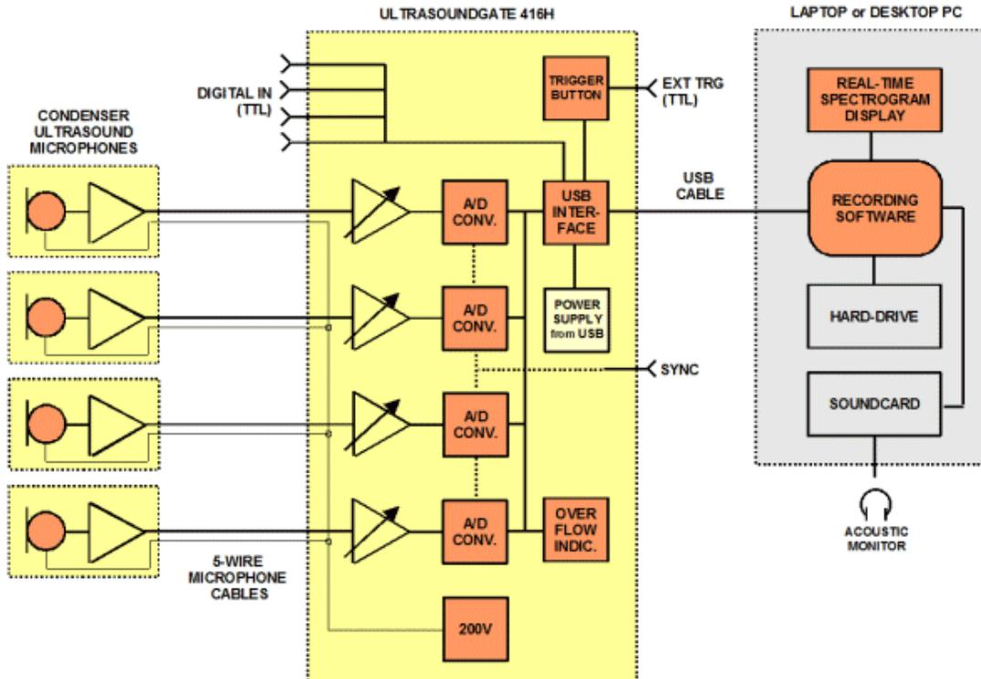
Functional principle of the UltraSoundGate 416H
