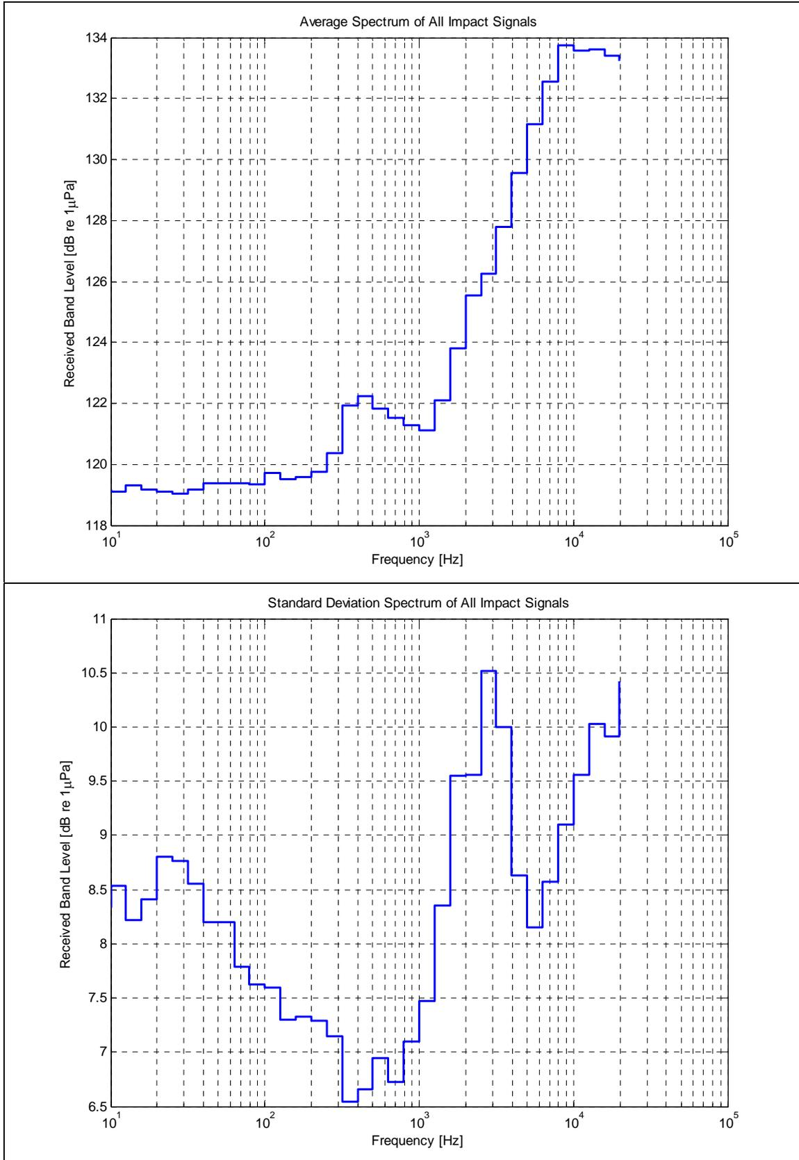
Figure 34. Average Spectrum and Standard Deviation (Impact, Sheet Pile, Shallow Hydrophone)
