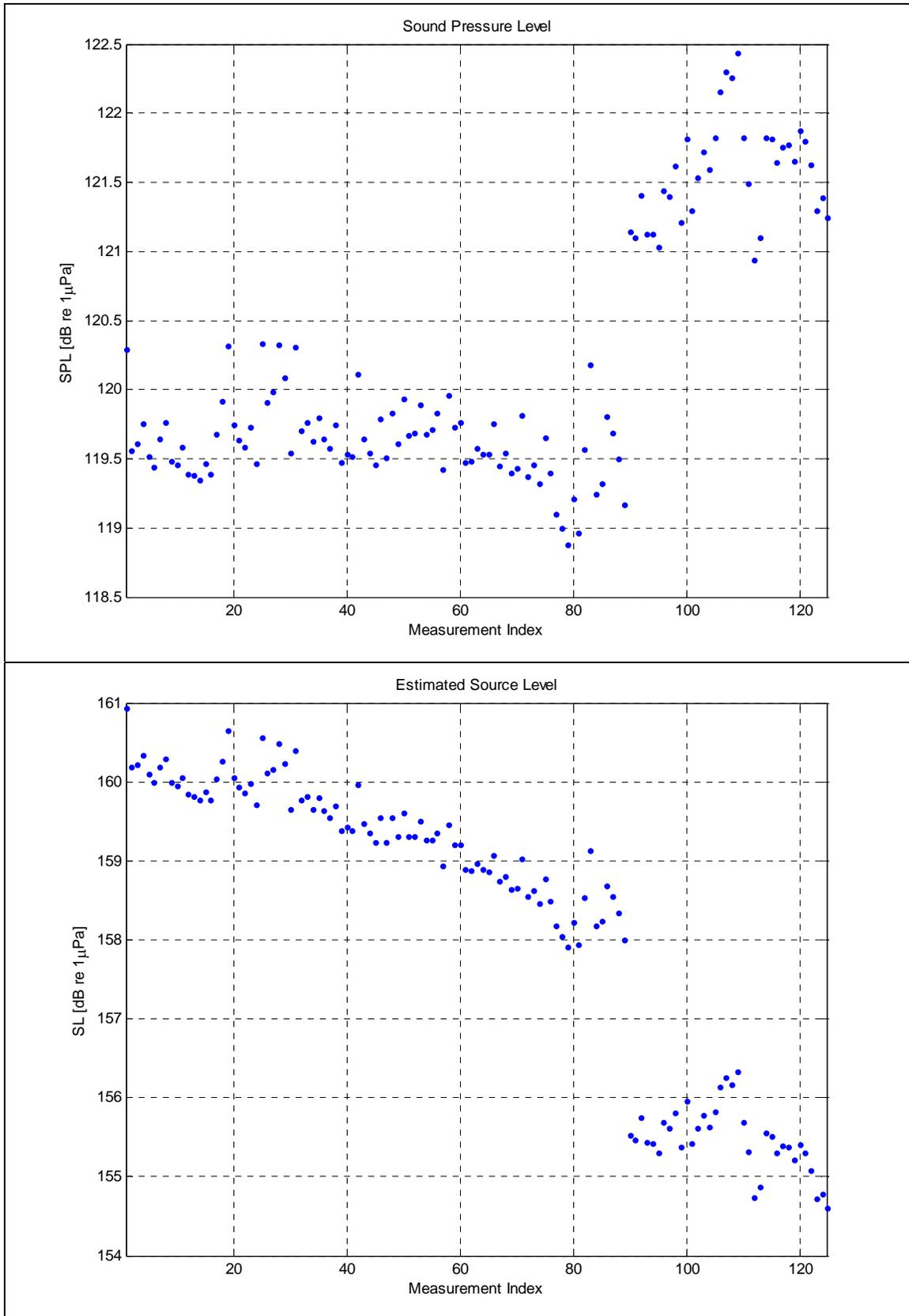
Figure 25. Sound Pressure Level and Estimated Source Level (Vibratory, Sheet Pile – Tail Wall)
