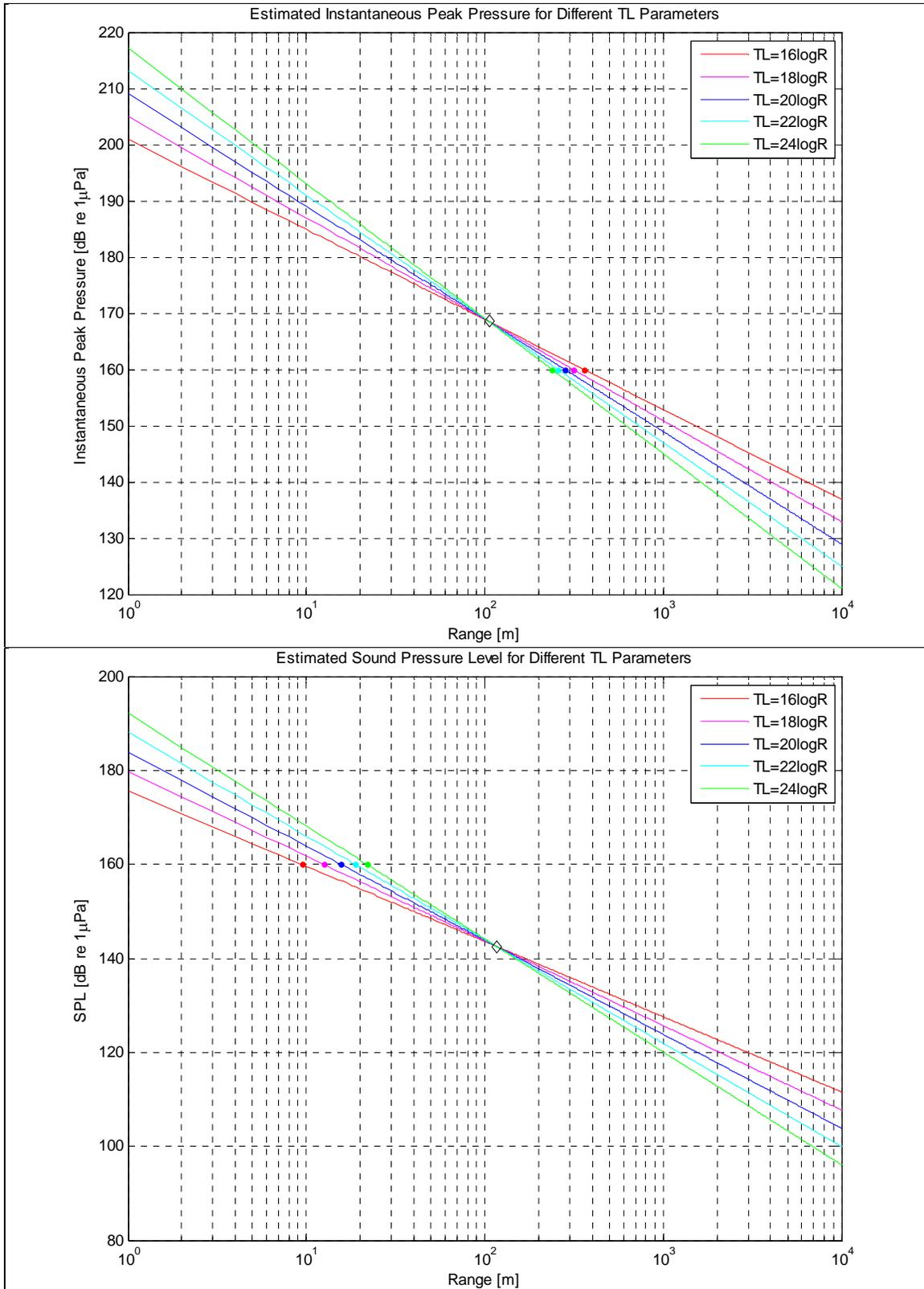
Figure 73. Consideration of Different Transmission Loss Configuration (Impact, Hairpin)
