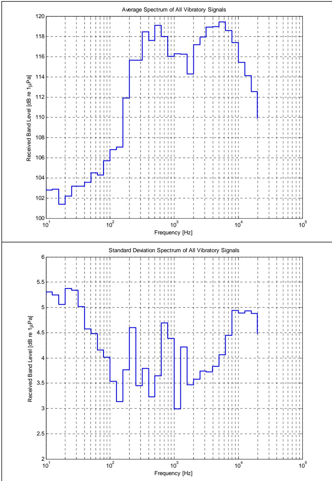
Figure 20. Average Spectrum and Standard Deviation (Vibratory, Round-Pile)
