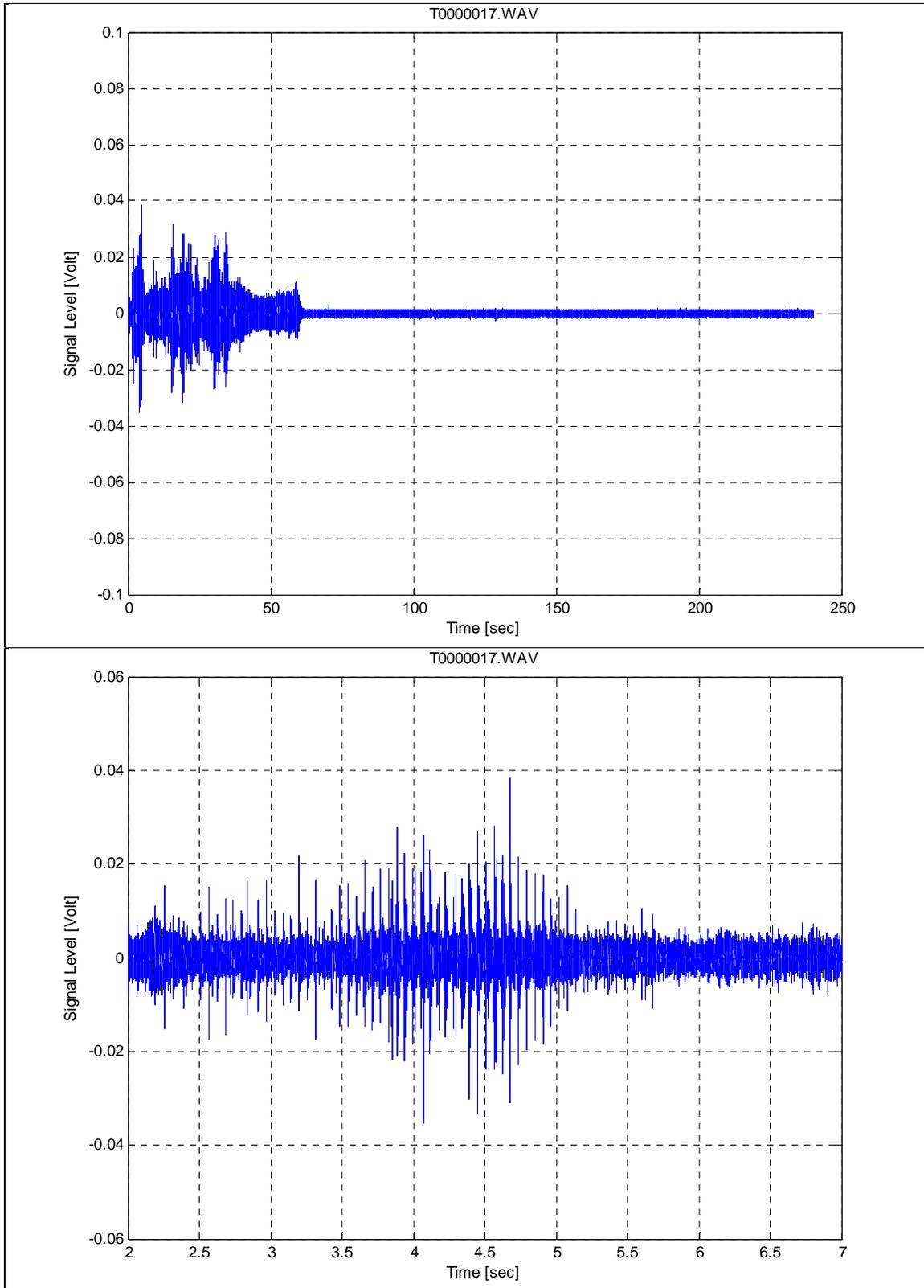
Figure 15. Raw Time Series of Pile Driving (Vibratory, Wye-Pile)
