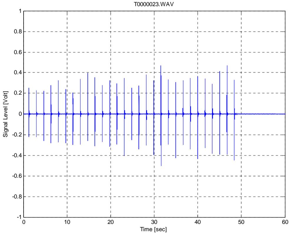
**Figure 35. Raw Time Series of Pile Driving (Impact, Sheet Pile, Shallow Hydrophone)**
