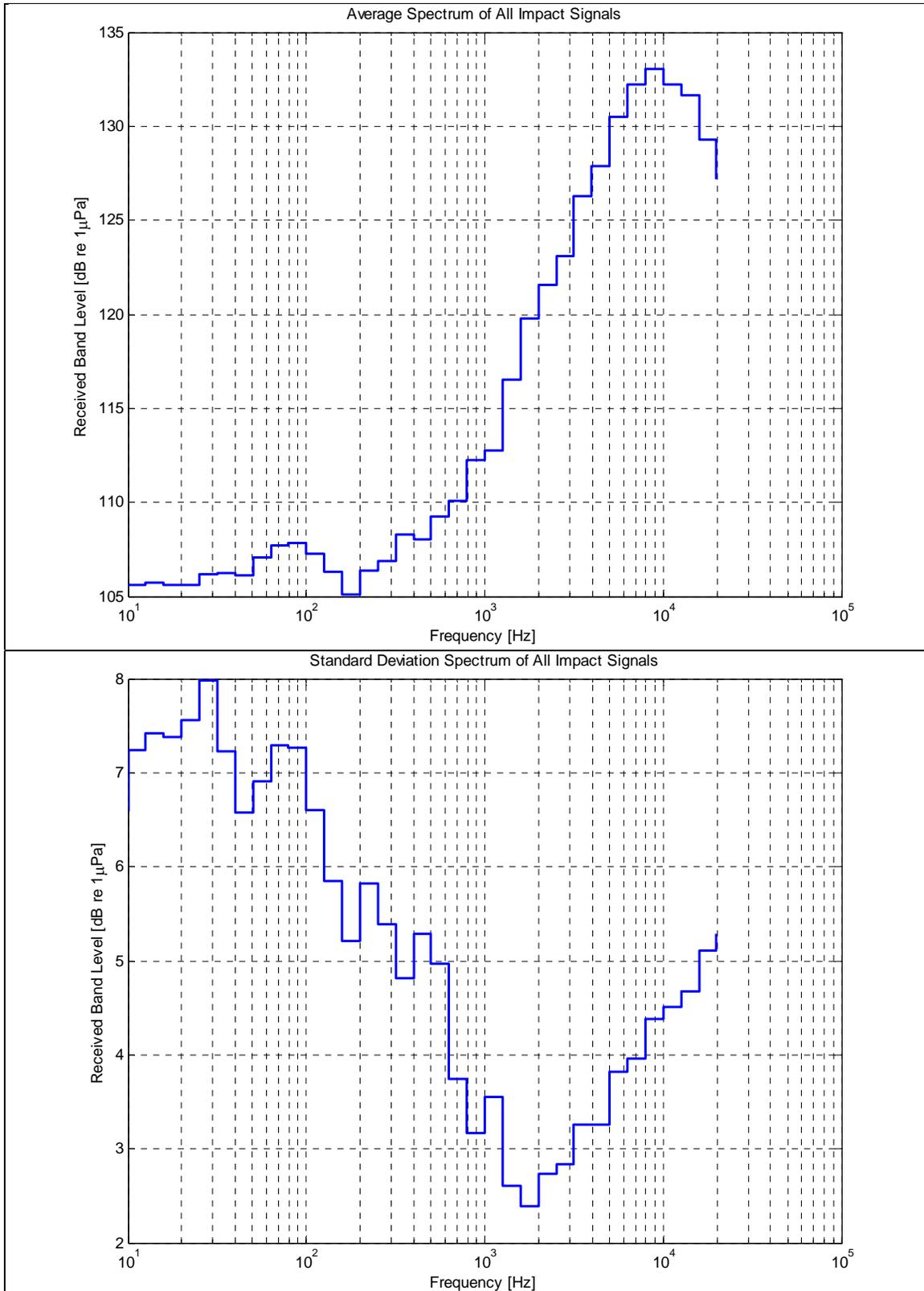
Figure 58. Average Spectrum and Standard Deviation (Impact, Wye-Pile)
