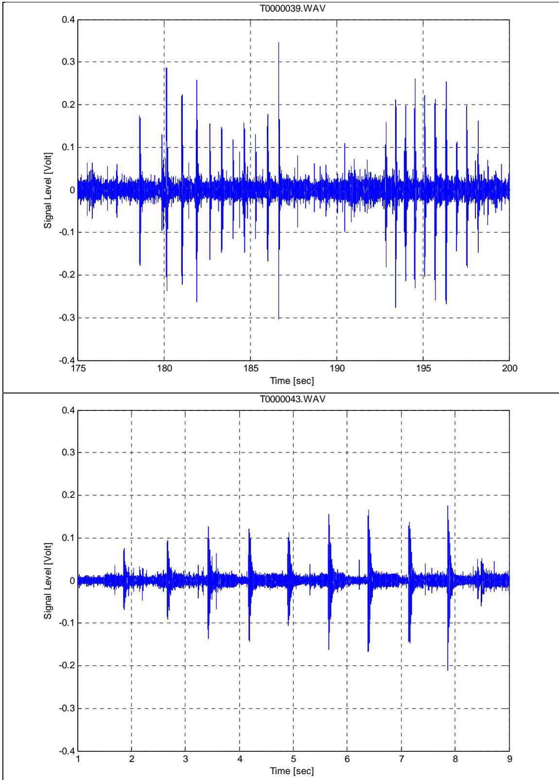
**Figure 90. Raw Time Series of Hand Hammer Impacts**
