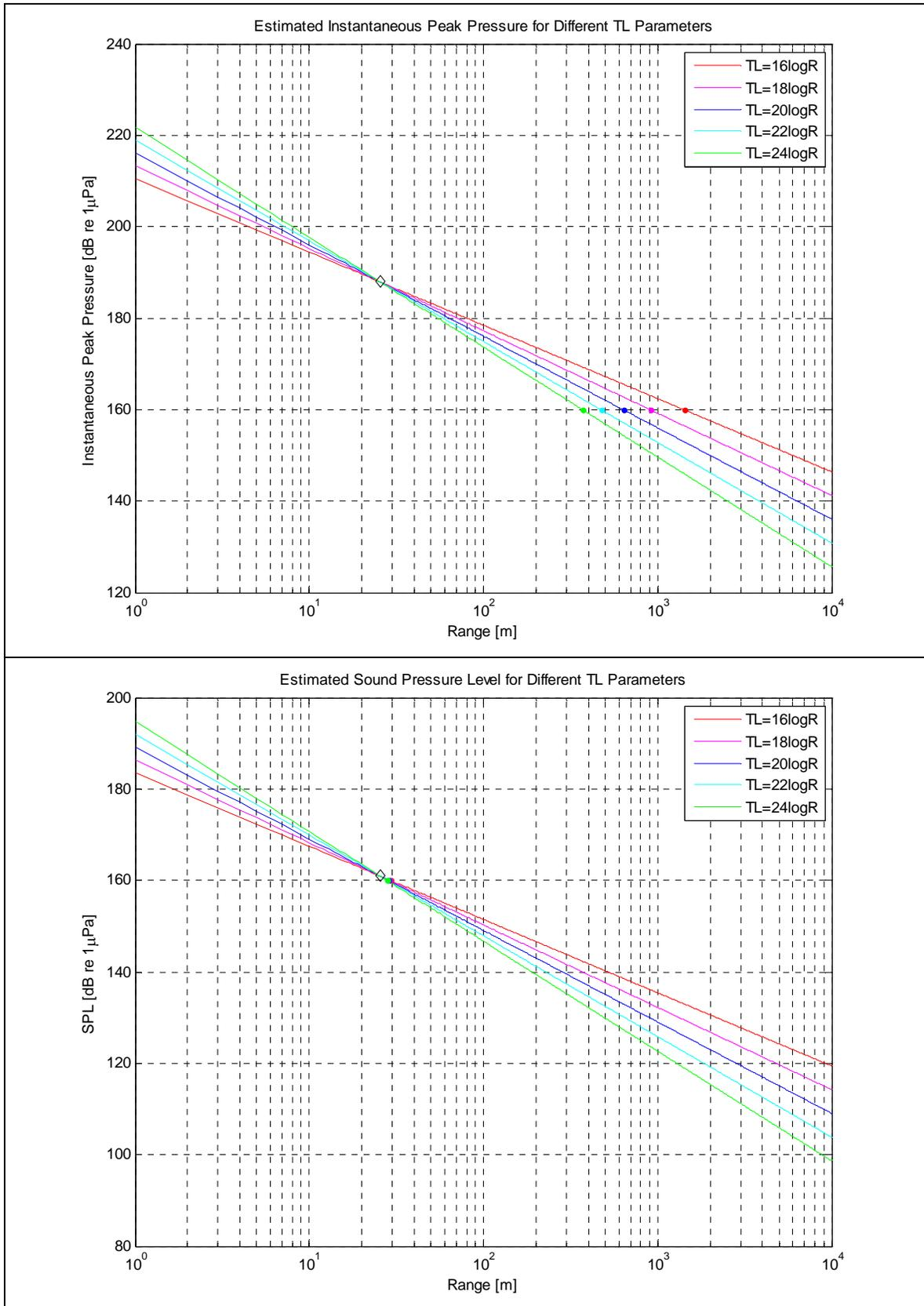
Figure 77 (g). Consideration of Different Transmission Loss Configuration for Impact ID 7
