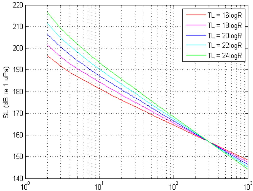
**Figure 88. Consideration of Different Transmission Loss Configurations (Bucket Dredging)**
