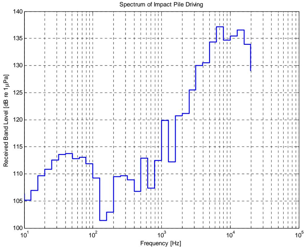
**Figure 67. One-Third Octave Spectrum for Pile Driving
