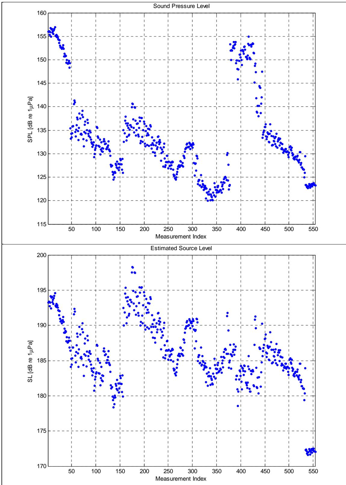
Figure 5. Sound Pressure Level and Estimated Source Level (Vibratory, Sheet Pile)
