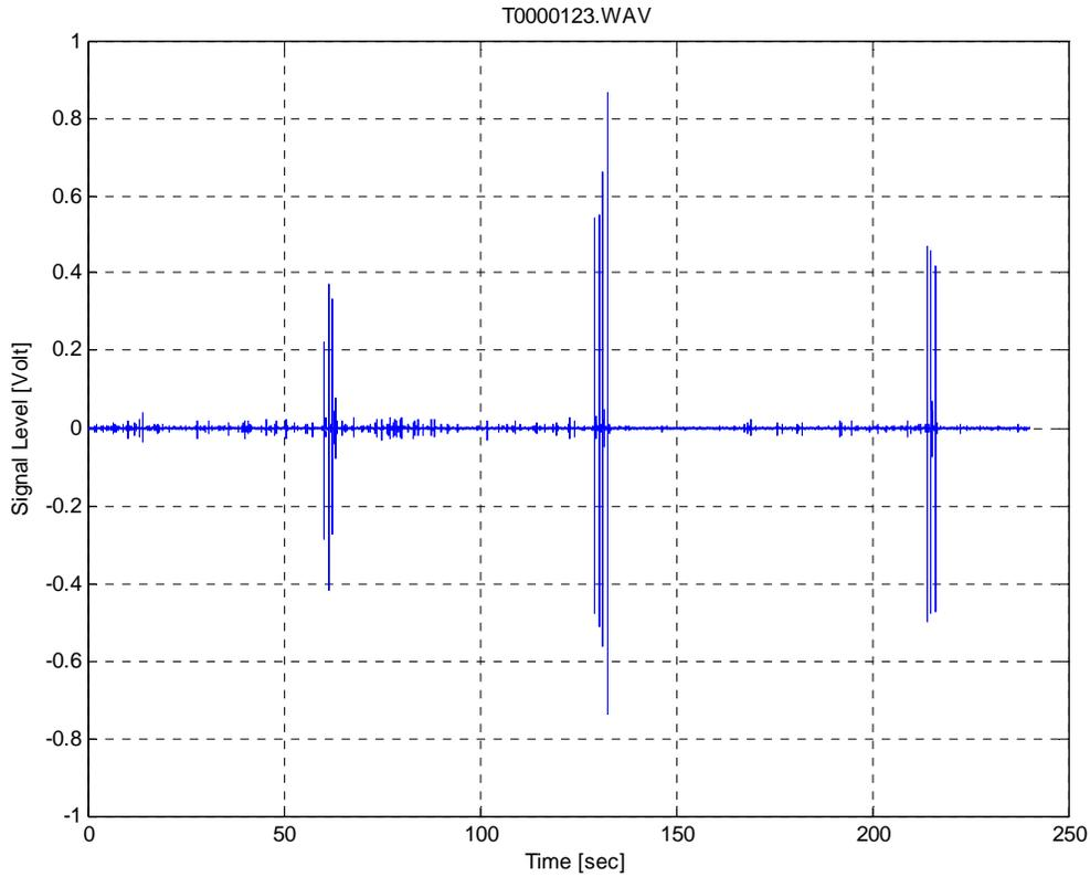
**Figure 59. Raw Time Series of Pile Driving (Impact, Wye-Pile)**
