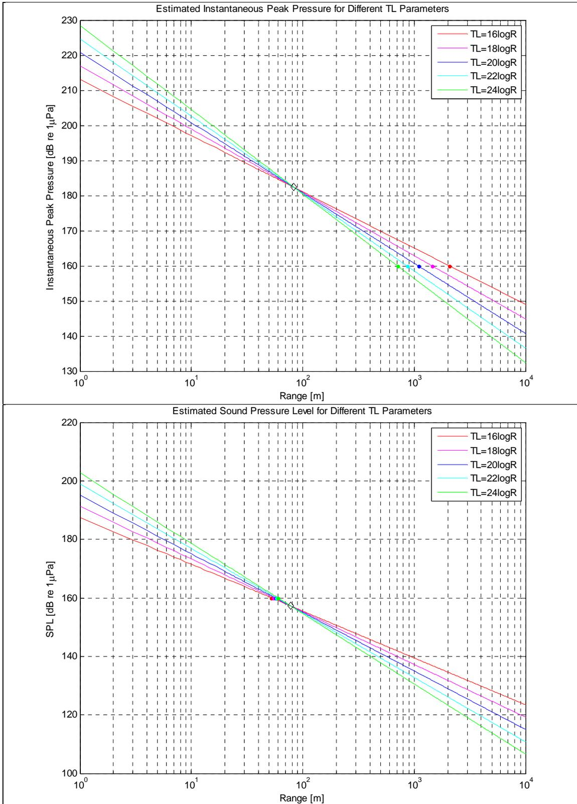
**Figure 37. Consideration of Different Transmission Loss Configuration (Impact, Sheet Pile, Shallow Hydrophone)**
