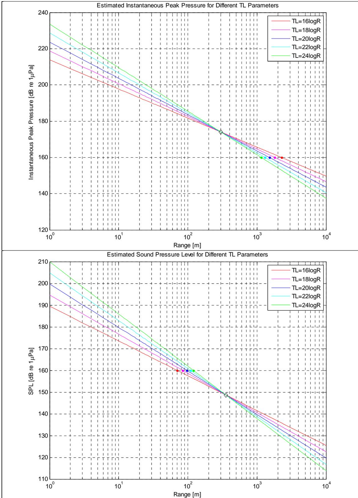
**Figure 49. Consideration of Different Transmission Loss Configuration
