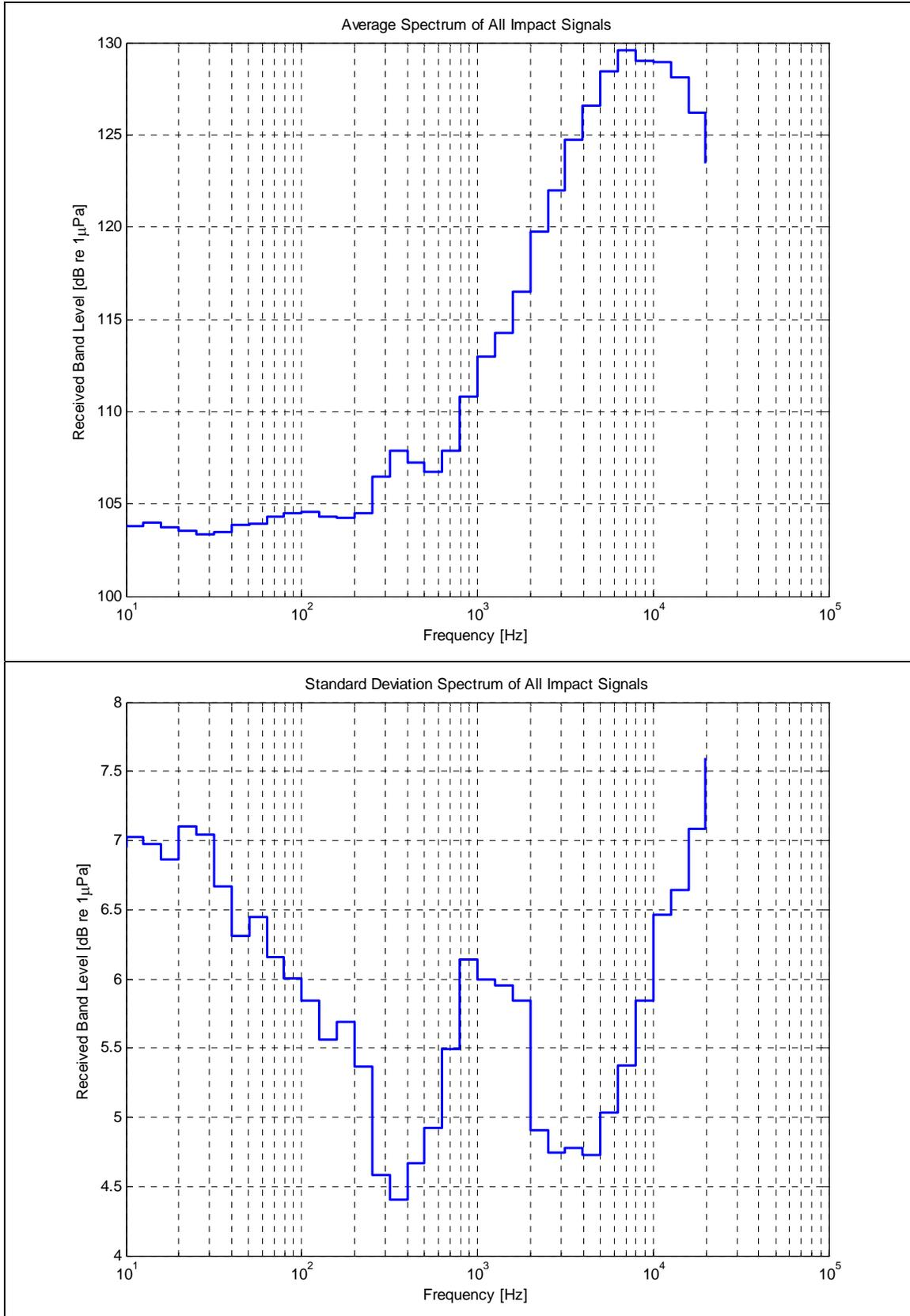
Figure 65. Average Spectrum and Standard Deviation (Impact, Sheet Pile, Shallow Hydrophone)
