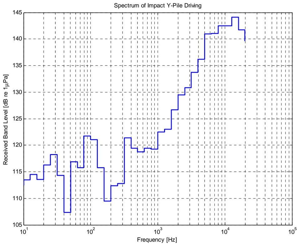
**Figure 60. One-Third Octave Spectrum for Pile Driving (Impact, Wye-Pile)**
