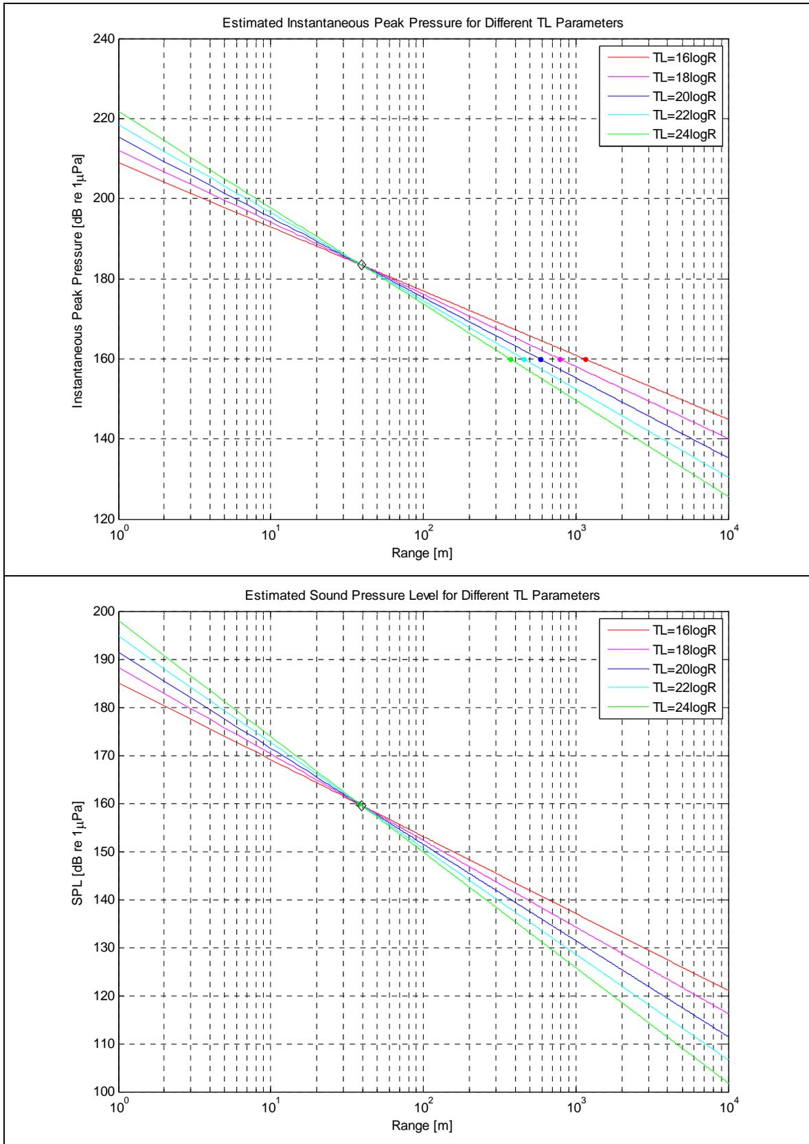
Figure 77 (d). Consideration of Different Transmission Loss Configuration for Impact ID 4
