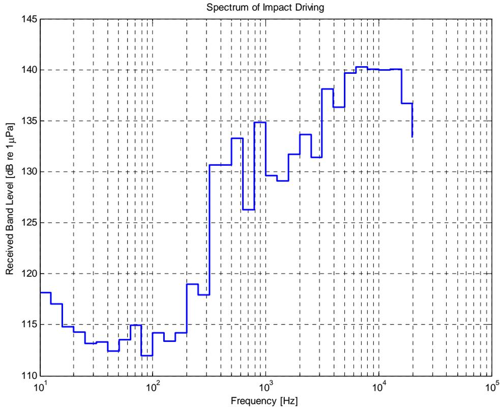
**Figure 48. One-Third Octave Spectrum for Pile Driving (Impact, Sheet Pile, Deep Hydrophone)**
