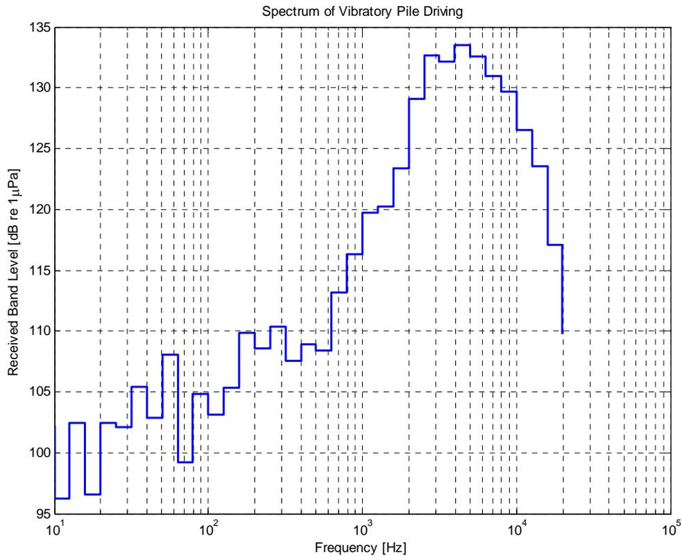
**Figure 9. One-Third Octave Spectrum for Pile Driving (Vibratory, Sheet Pile)**
