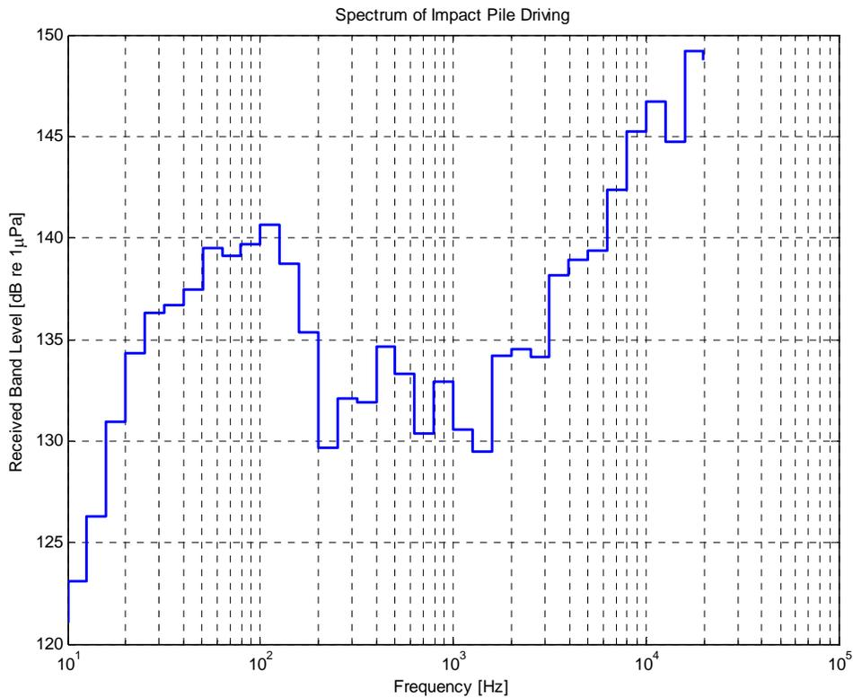
**Figure 36. One-Third Octave Spectrum for Pile Driving (Impact, Sheet Pile, Shallow Hydrophone)**
