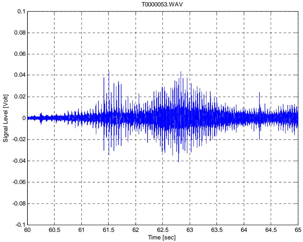
Figure 21. Raw Time Series of Pile Driving (Vibratory, Round Pile)
