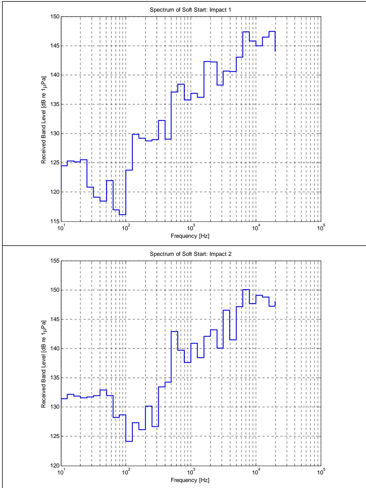
Figure 76 (a). One-Third Octave Spectrum for Pile Driving (Impact, Soft Start)
