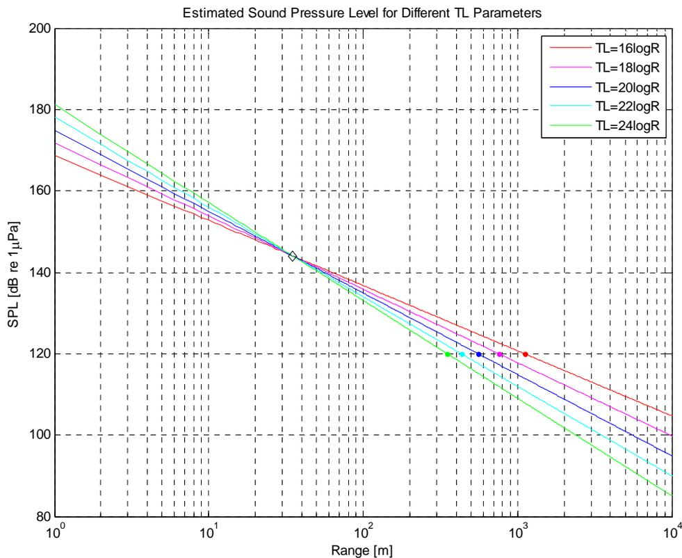
**Figure 23. Consideration of Different Transmission Loss Configuration (Vibratory, Round Pile)**
