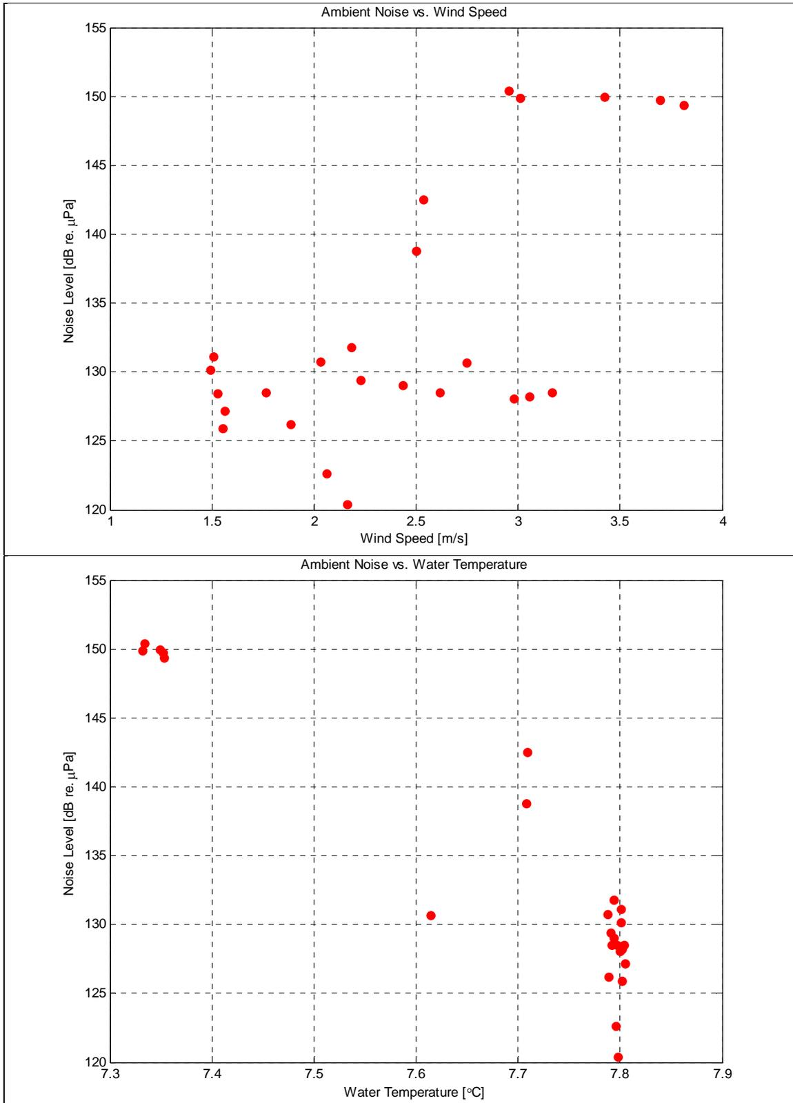
Figure 83. Wind Speed, Water Temperature, and the Relationship with Background Noise Level
