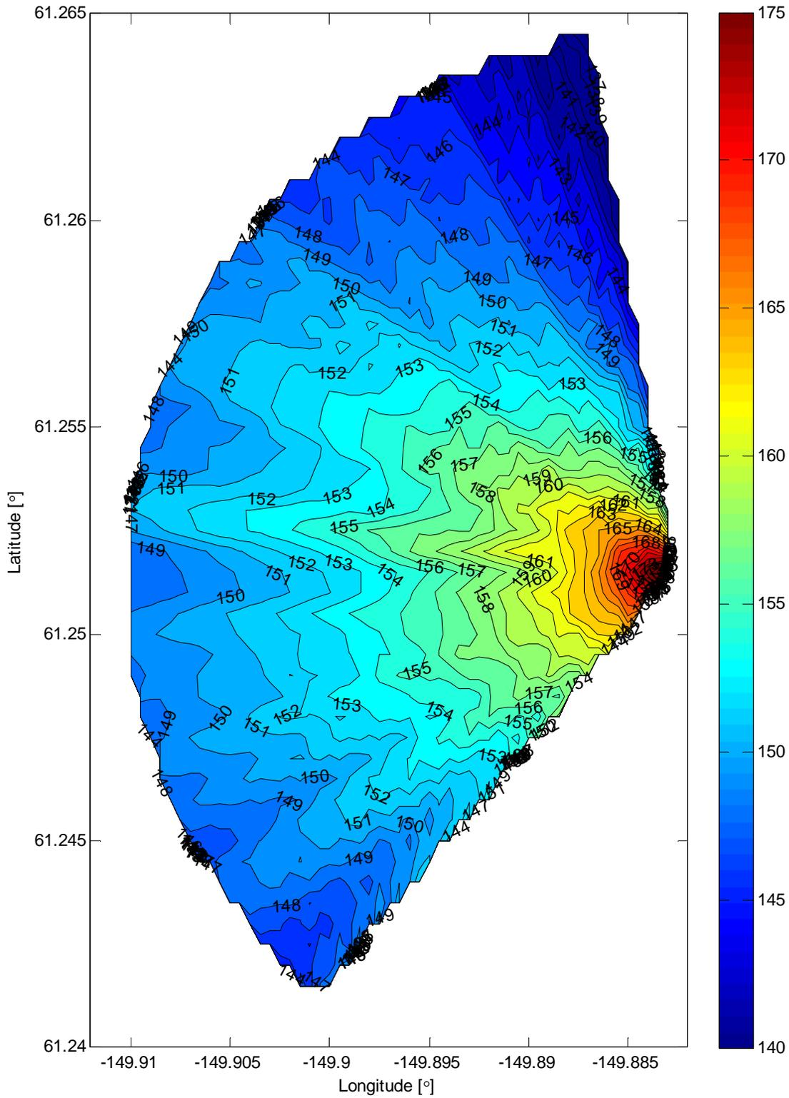
**Figure 39. Isopleths from Instantaneous Peak Pressure with Smoothing Window Size of 5 (Impact, Sheet Pile, Shallow Hydrophone)**
