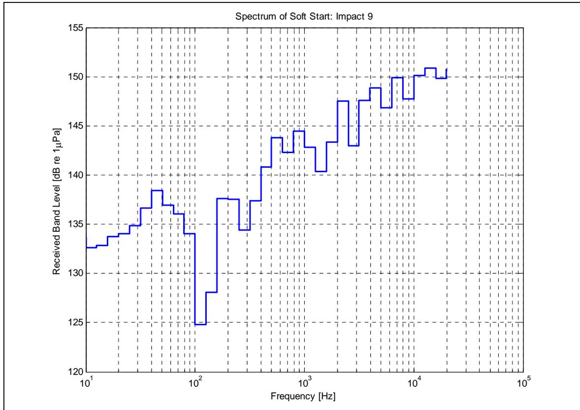
Figure 76 (e). One-Third Octave Spectrum for Pile Driving (Impact, Soft Start)
