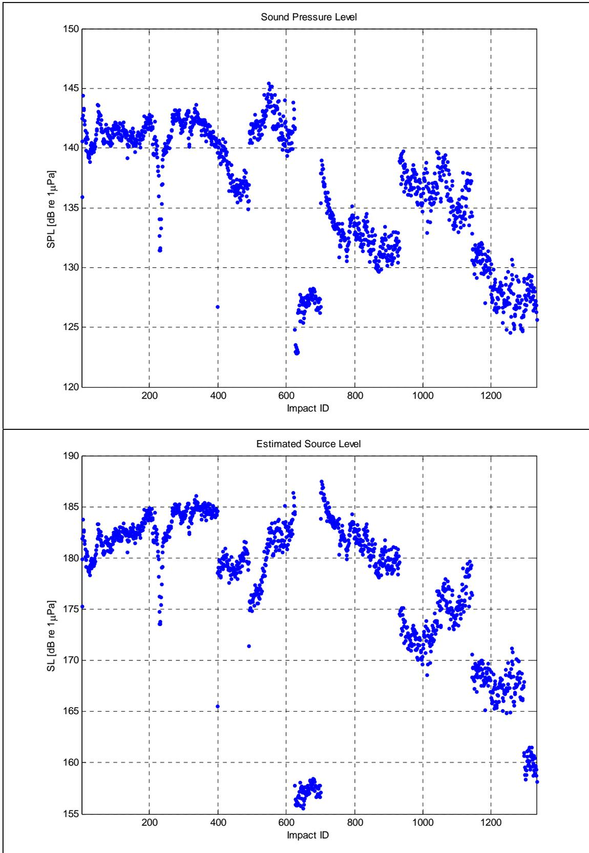
Figure 63. Sound Pressure Level and Estimated Source Level (Impact, Sheet Pile – Tail Wall)
