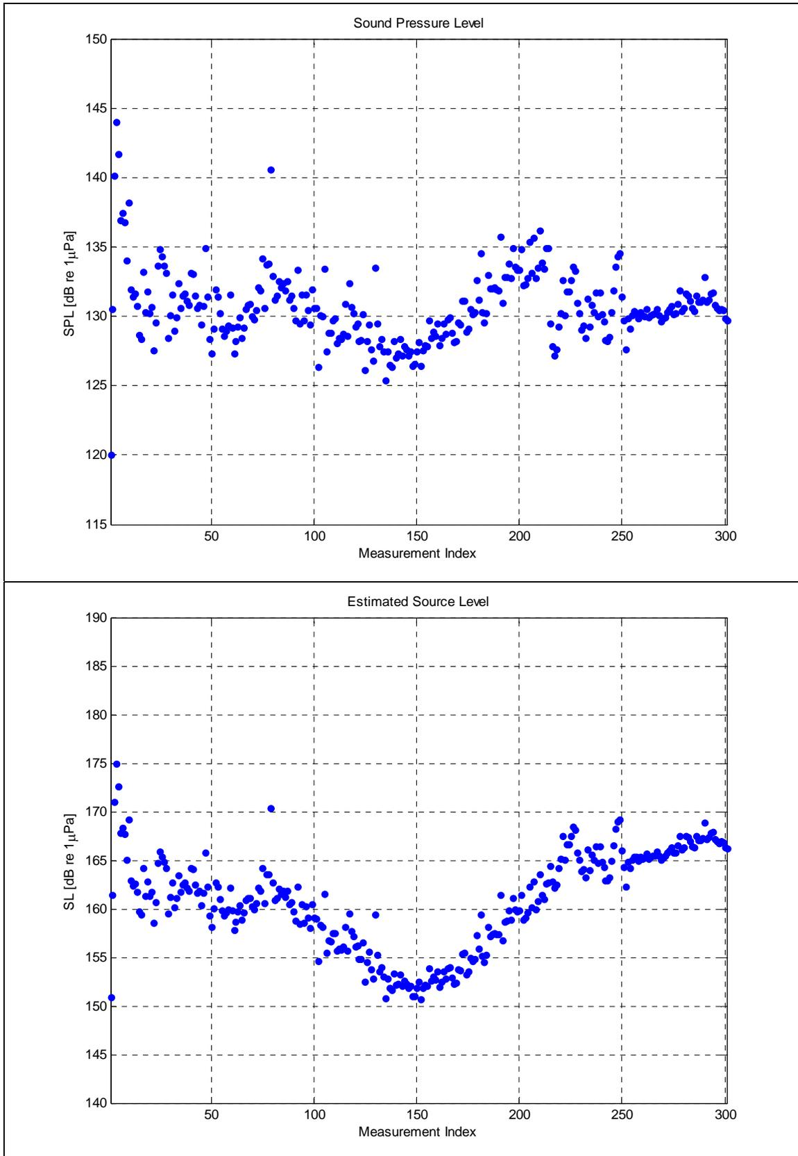
Figure 19. Sound Pressure Level and Estimated Source Level (Vibratory, Round-Pile)
