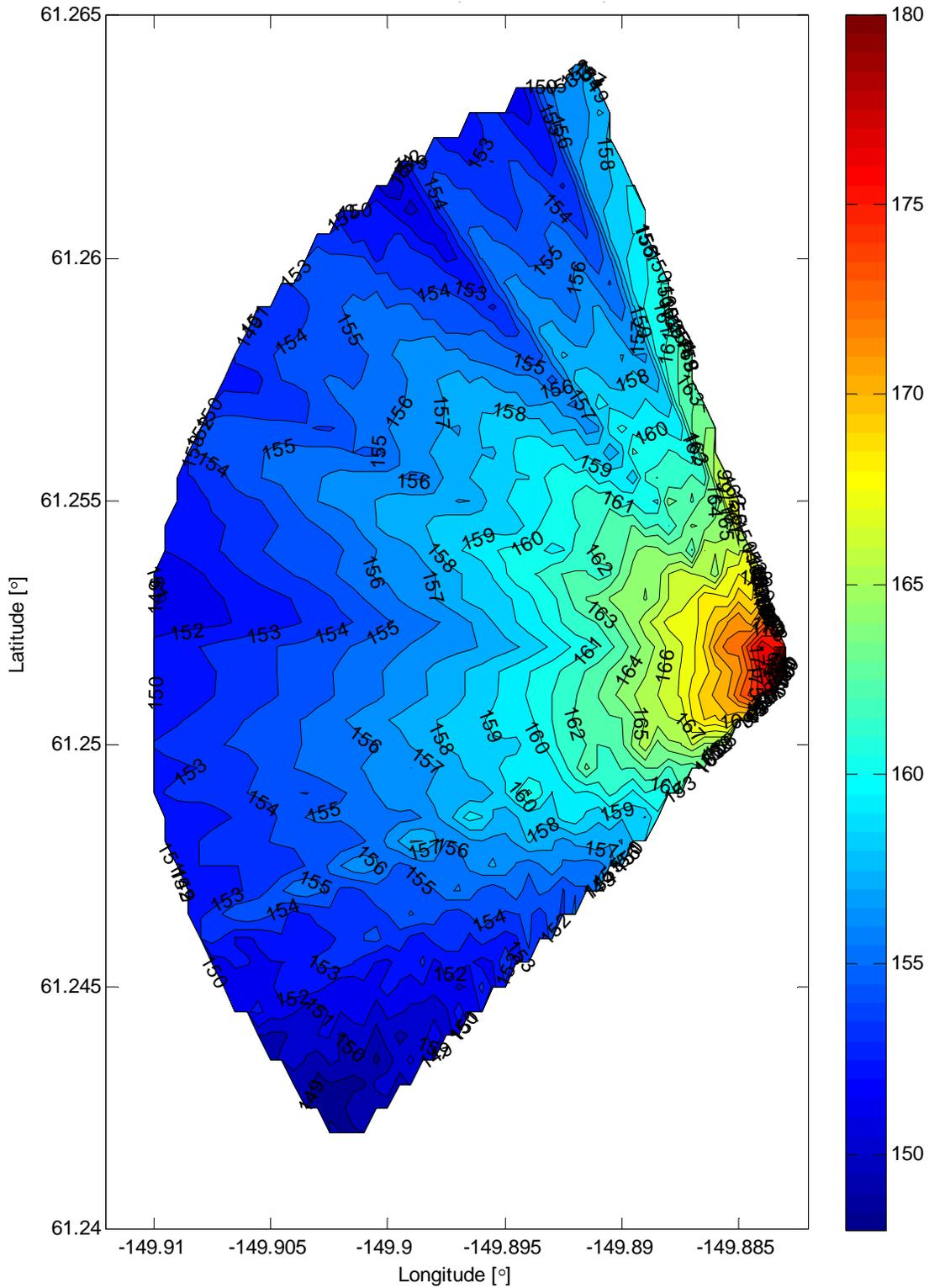
**Figure 51. Isopleths from Instantaneous Peak Pressure with Smoothing Window Size of 5 (Impact, Sheet Pile, Deep Hydrophone)**
