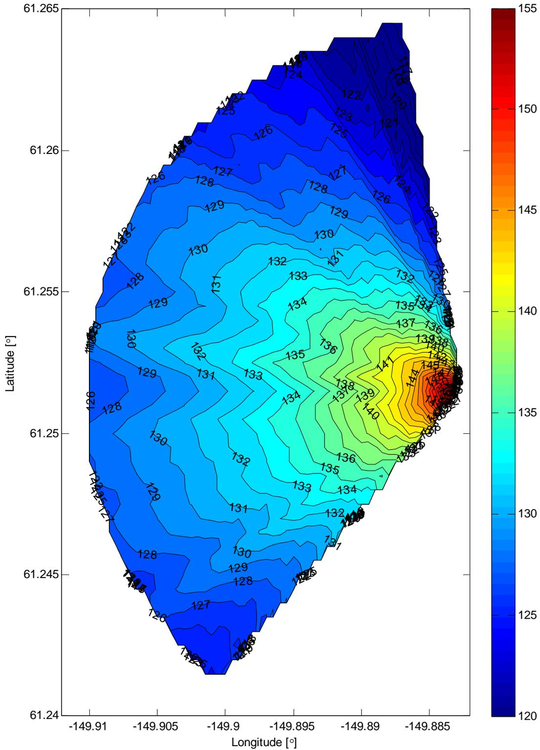
Figure 41. Isopleths from Sound Pressure Level with Smoothing Window Size of 5 (Impact, Sheet Pile, Shallow Hydrophone)
