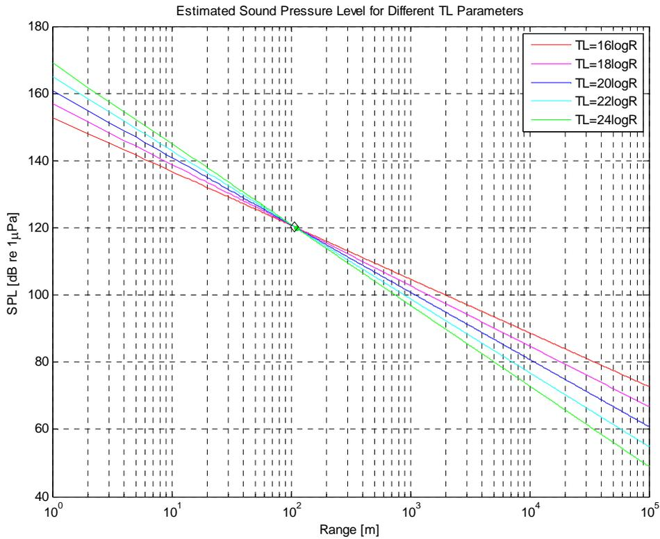
**Figure 30. Consideration of Different Transmission Loss Configuration (Vibratory, Sheet Pile – Tail Wall)**
