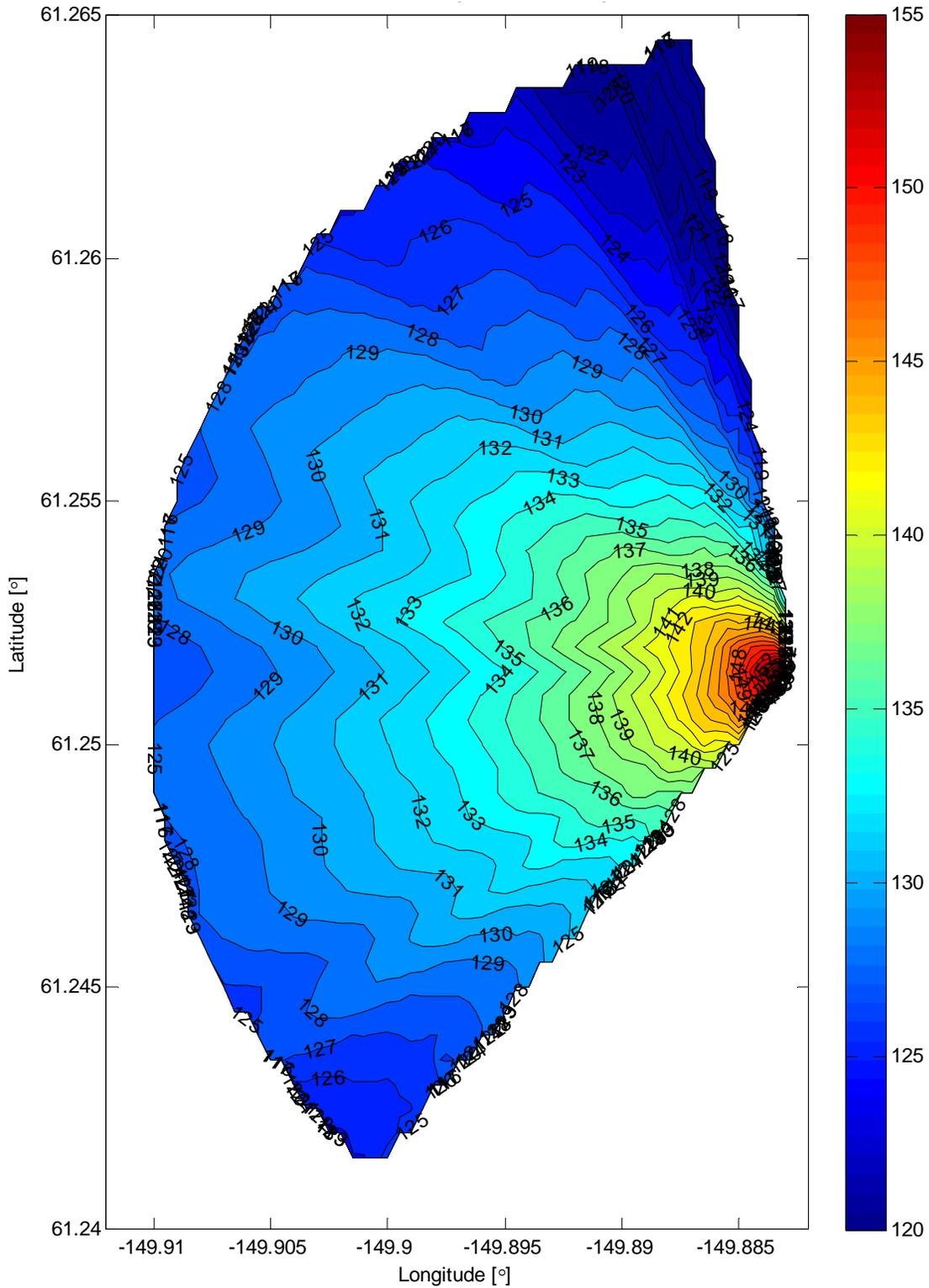
Figure 42. Isopleths from Sound Pressure Level with Smoothing Window Size of 9 (Impact, Sheet Pile, Shallow Hydrophone)
