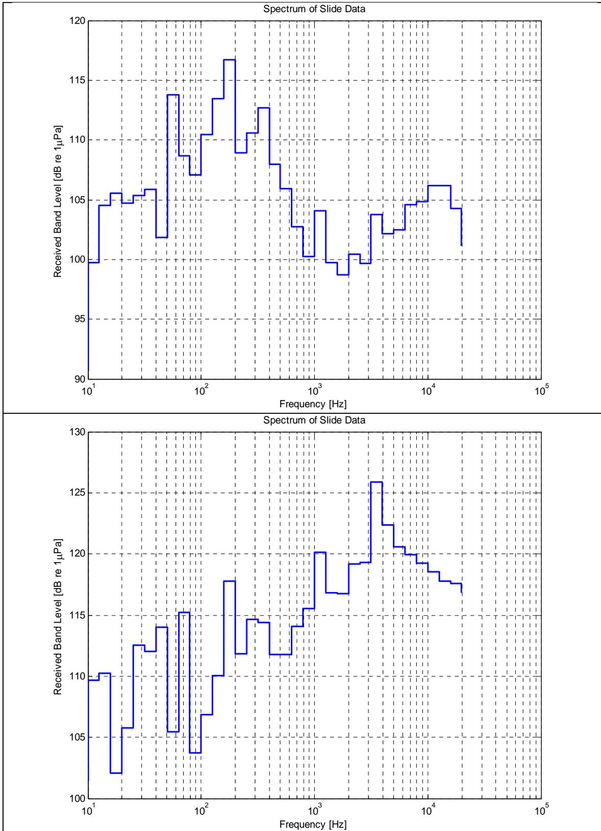
Figure 80. One-Third Octave Spectrum for Pile Driving (Stabbing)
