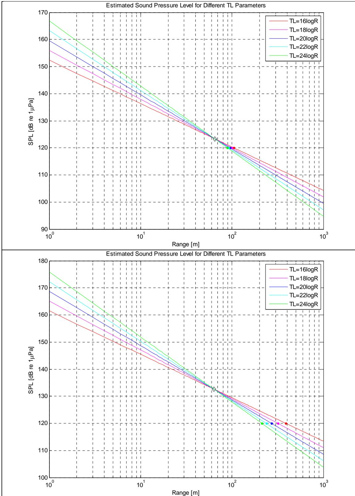
Figure 81. Consideration of Different Transmission Loss Configuration (Stabbing)
