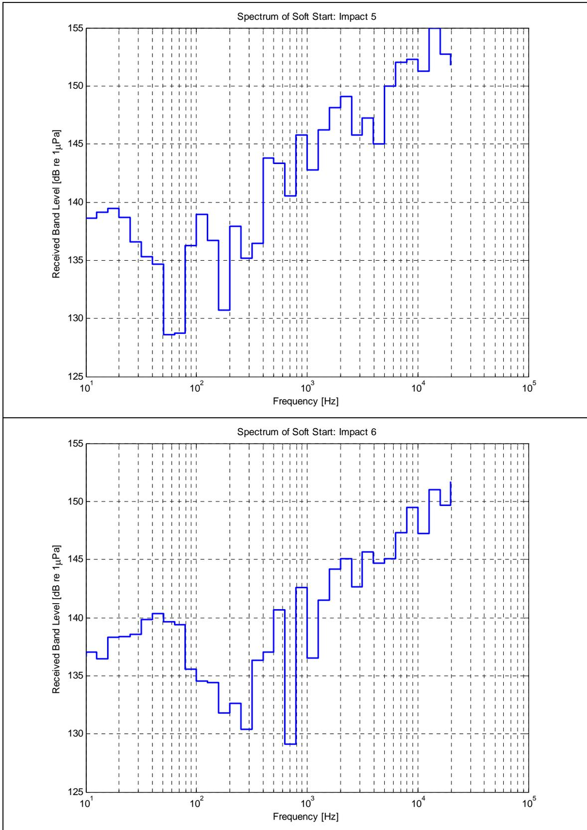
Figure 76 (c). One-Third Octave Spectrum for Pile Driving (Impact, Soft Start)
