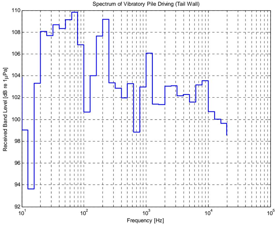
**Figure 29. One-Third Octave Spectrum for Pile Driving (Vibratory, Wye-Pile)**
