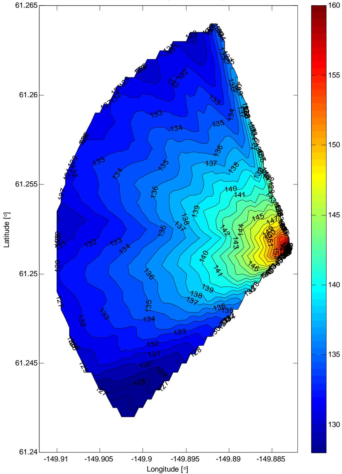
**Figure 54. Isopleths from Sound Pressure Level with Smoothing Window Size of 9 (Impact, Sheet Pile, Shallow Hydrophone)**
