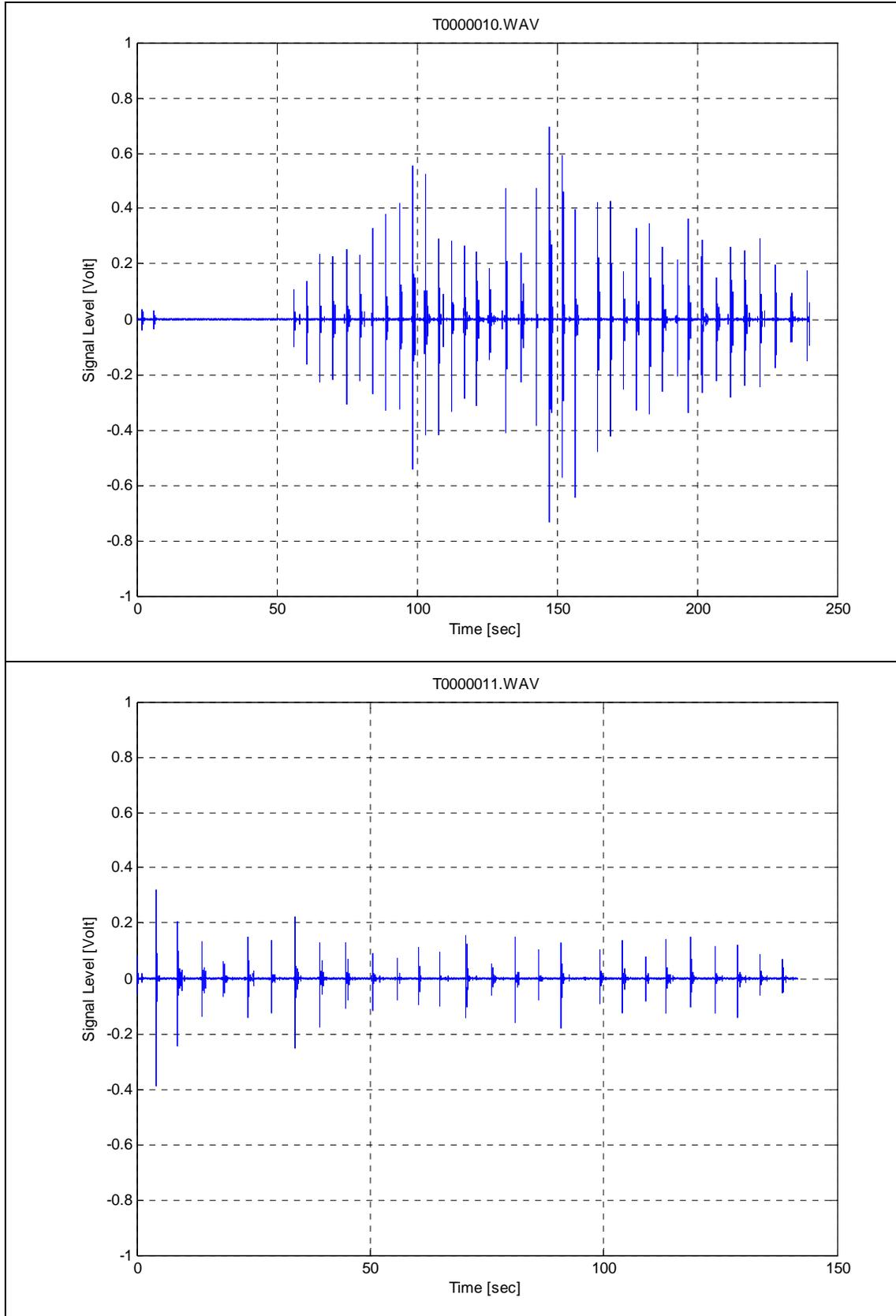
Figure 70 (a). Raw Time Series of Impact Pile Driving (Impact, Hairpin)
