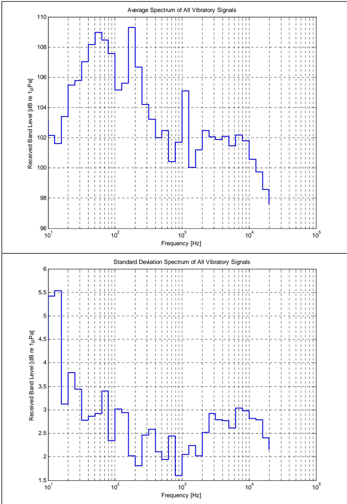
Figure 27. Average Spectrum and Standard Deviation (Vibratory, Sheet Pile – Tail Wall)
