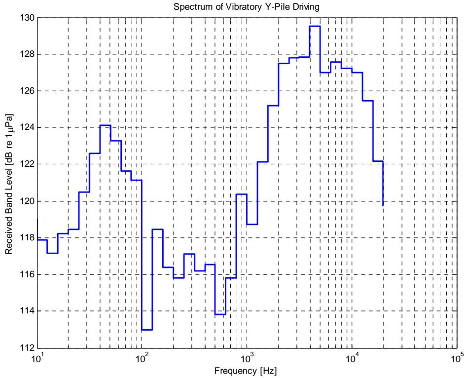
Figure 16. One-Third Octave Spectrum for Pile Driving (Vibratory, Wye-Pile)
