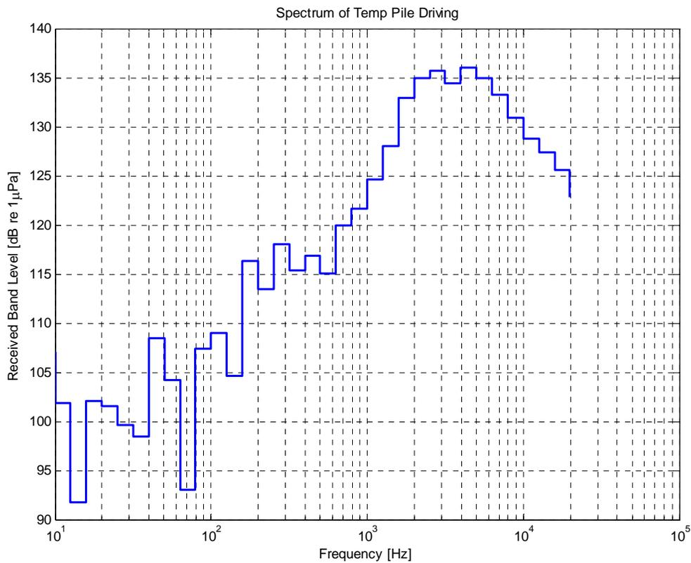
Figure 22. One-Third Octave Spectrum for Pile Driving (Vibratory, Round Pile)
