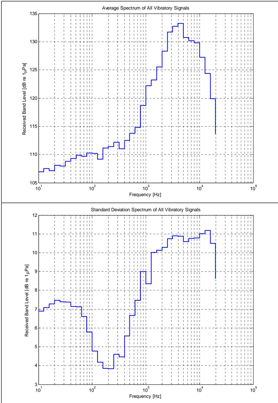
Figure 7. Average Spectrum and Standard Deviation (Vibratory, Sheet Pile)
