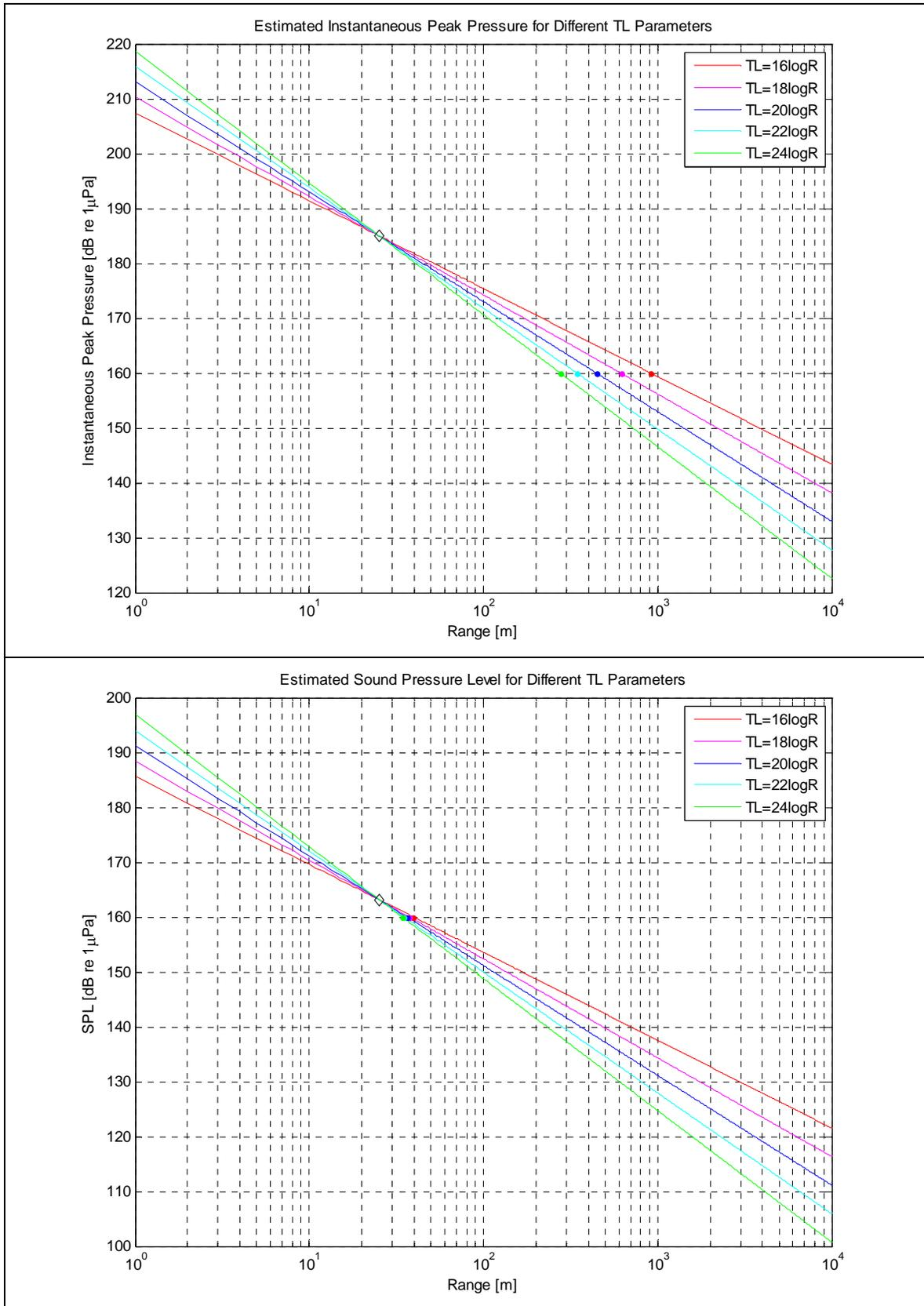
Figure 77 (h). Consideration of Different Transmission Loss Configuration for Impact ID 8
