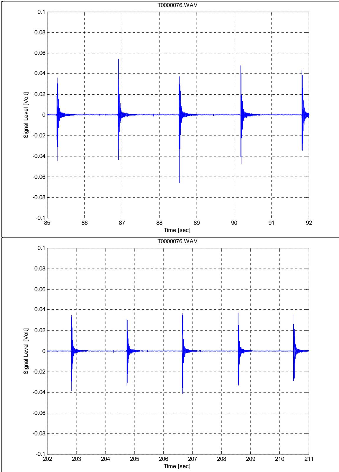
Figure 47. Raw Time Series of Pile Driving (Impact, Sheet Pile, Deep Hydrophone)
