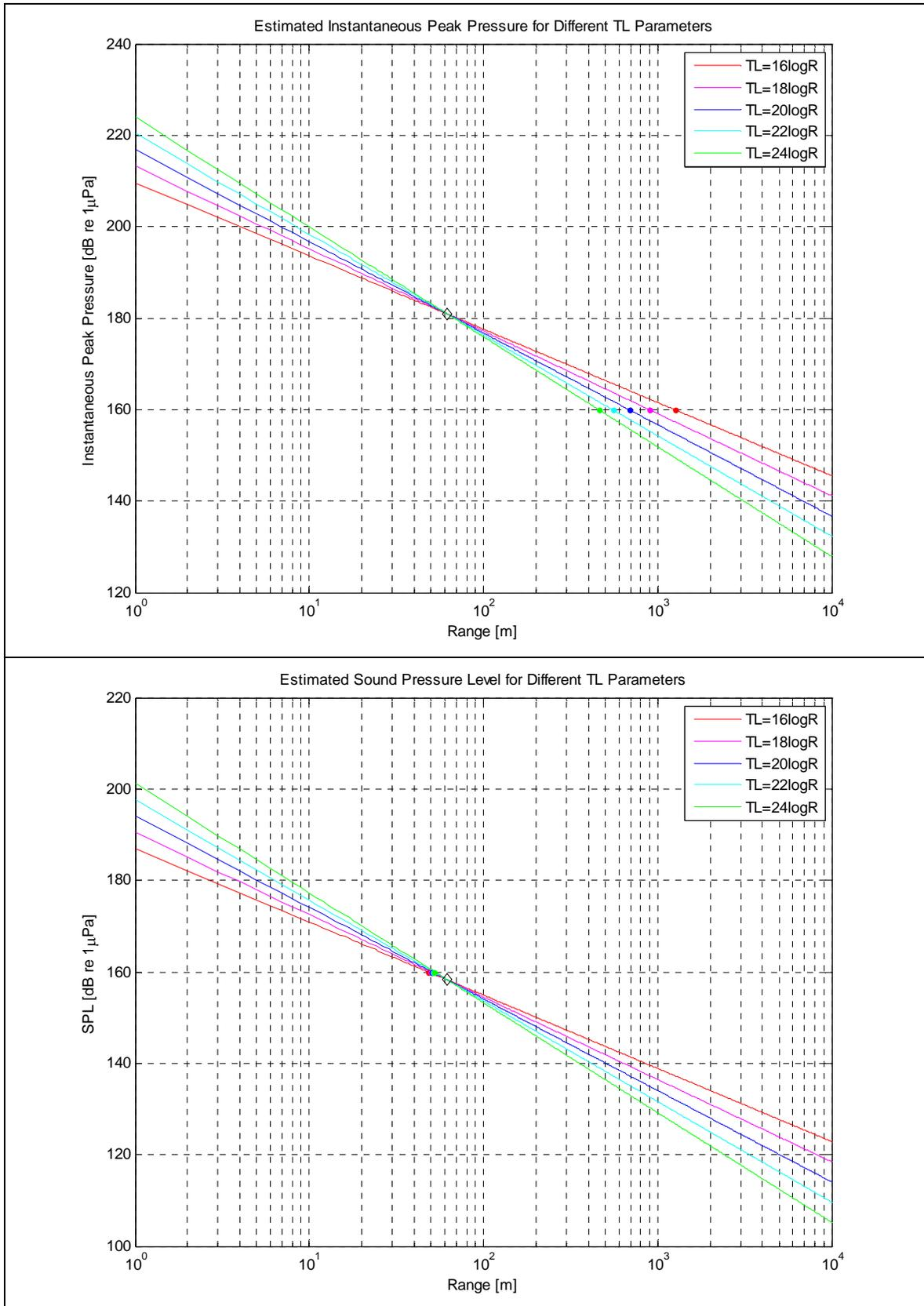
Figure 77 (b). Consideration of Different Transmission Loss Configuration for Impact ID 2
