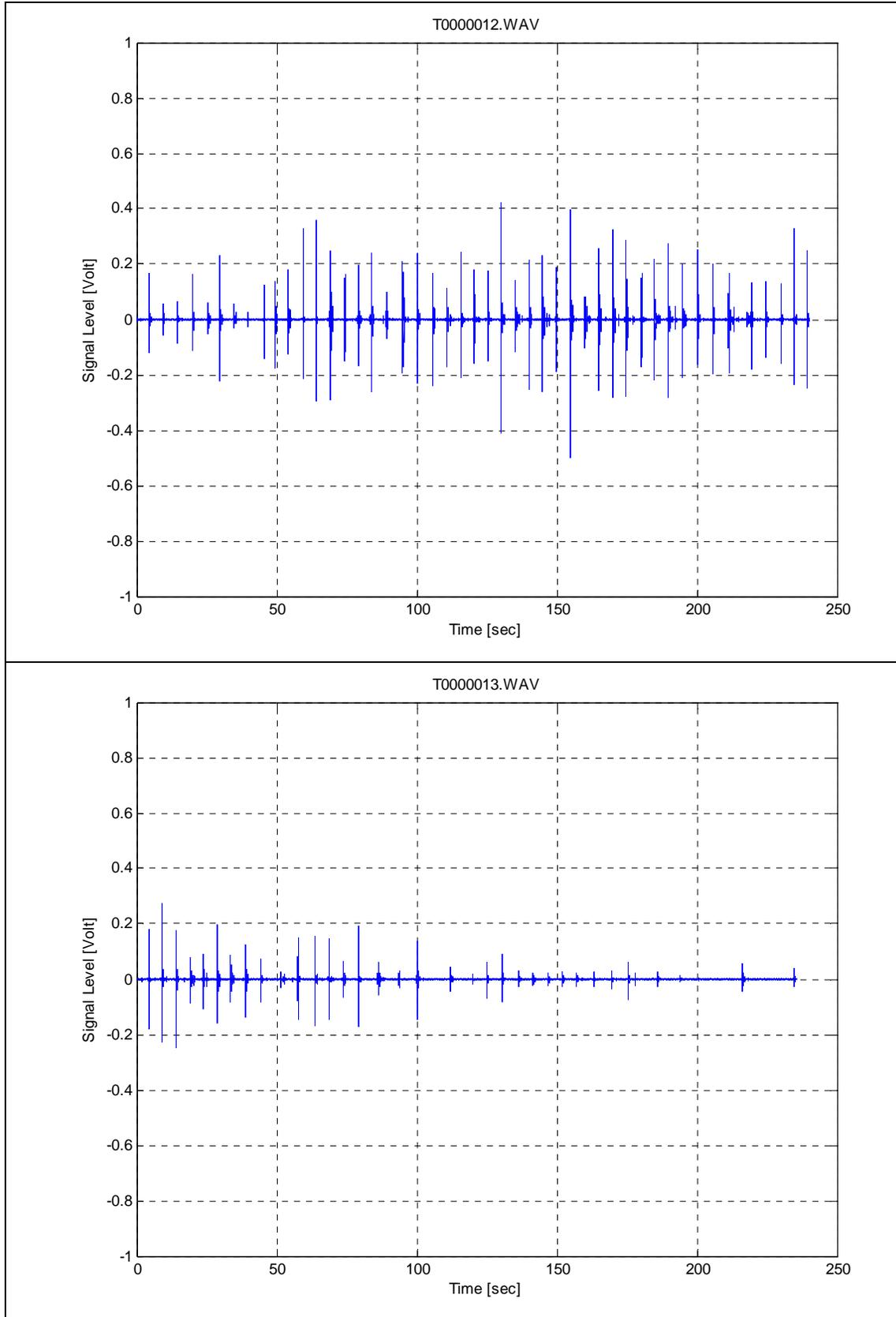
**Figure 70 (b). Raw Time Series of Impact Pile Driving (Impact, Hairpin)**
