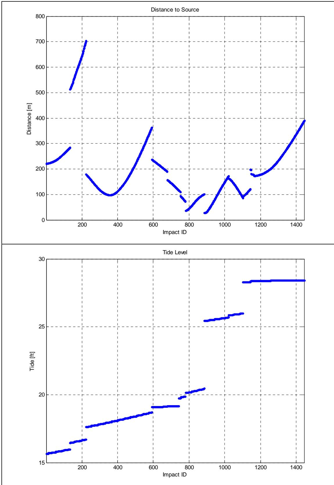
Figure 33. Distance to Source and Tide Level (Impact, Sheet Pile, Shallow Hydrophone)
