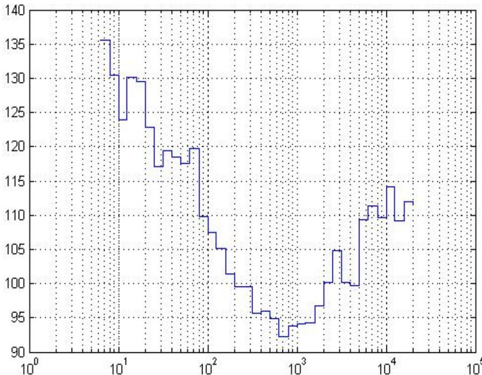
**Figure 87. One-Third Octave Spectrum for Bucket Dredging**
