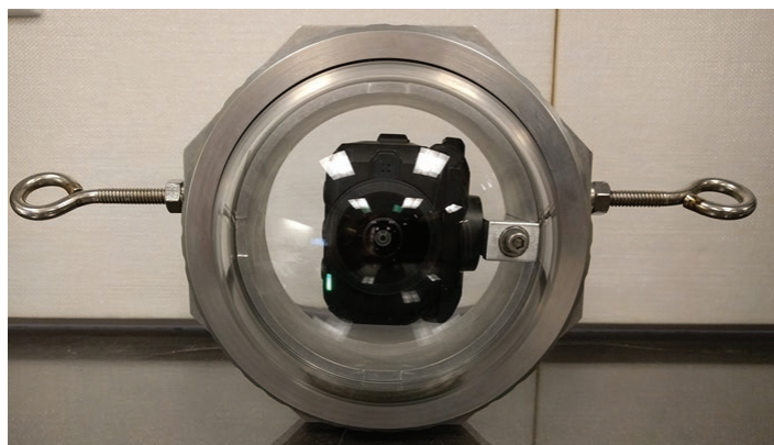
The Moana360 underwater rig is compatible with a range of small and large off-the-shelf 360-degree cameras.
