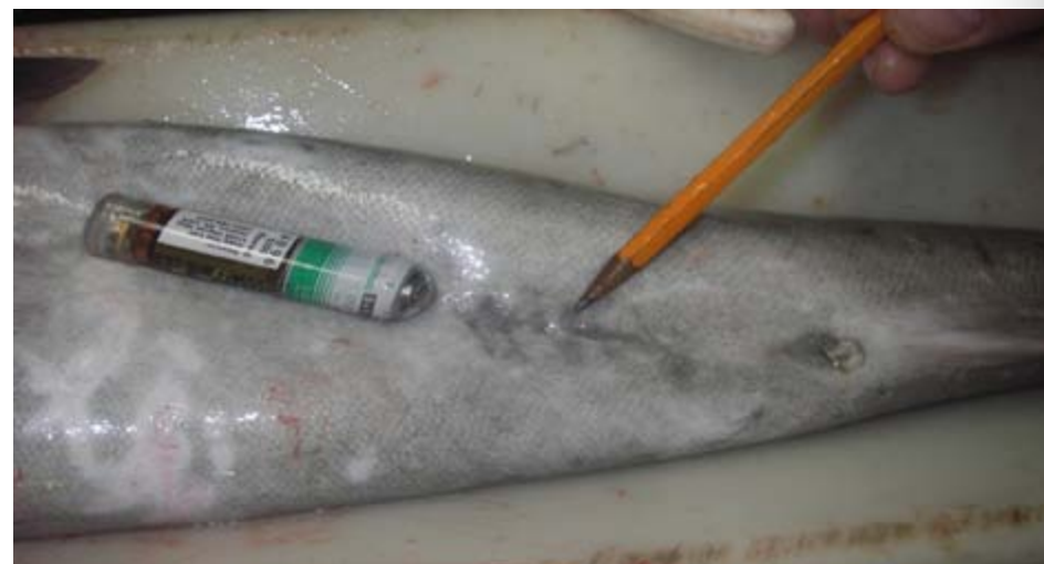
Figure 2. Picture of an electronic archival tag. The pencil is pointing to the location on the sablefish in which an incision will be made to insert the tag.
