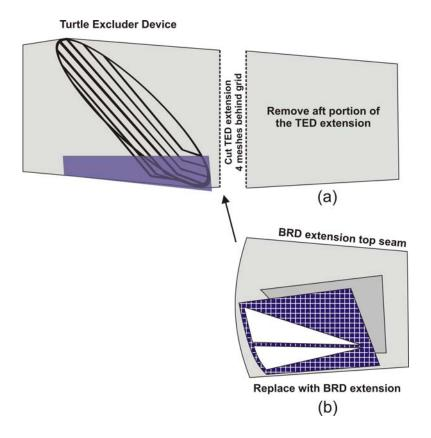
Figure 10: The Composite Panel BRD is installed in the trawl by removing a portion of the TED extension starting four (4) meshes behind the TED grid (a) and replacing it with the BRD extension. The codend is then attached to the trailing edge of the BRD extension (b).
