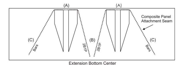
Figure 8: A schematic for the attachment of the composite panels to the BRD extension. (A) leading edge attachment, (B) inner seams, (C) outer seams
