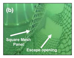
Figure 3: Composite panel on the port side with the square mesh component detached, causing the diamond mesh to collapse (a). Square mesh on the starboard side (b) supporting the diamond mesh maintaining space between the composite panel and trawl extension.
