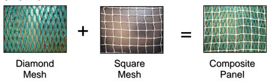
Figure 2: Components of the Composite Panel
