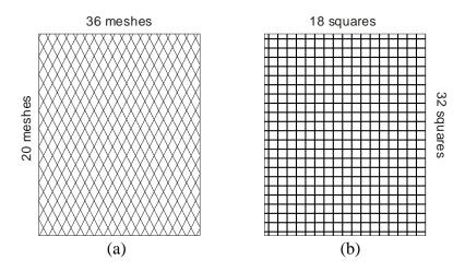
Figure 5: Components of the Composite Panel; (a) diamond mesh panel (DM), (b) Square mesh panel (SM).
