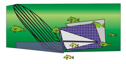
Figure 1: Composite Panel Shrimp Trawl Bycatch Reduction Device.
