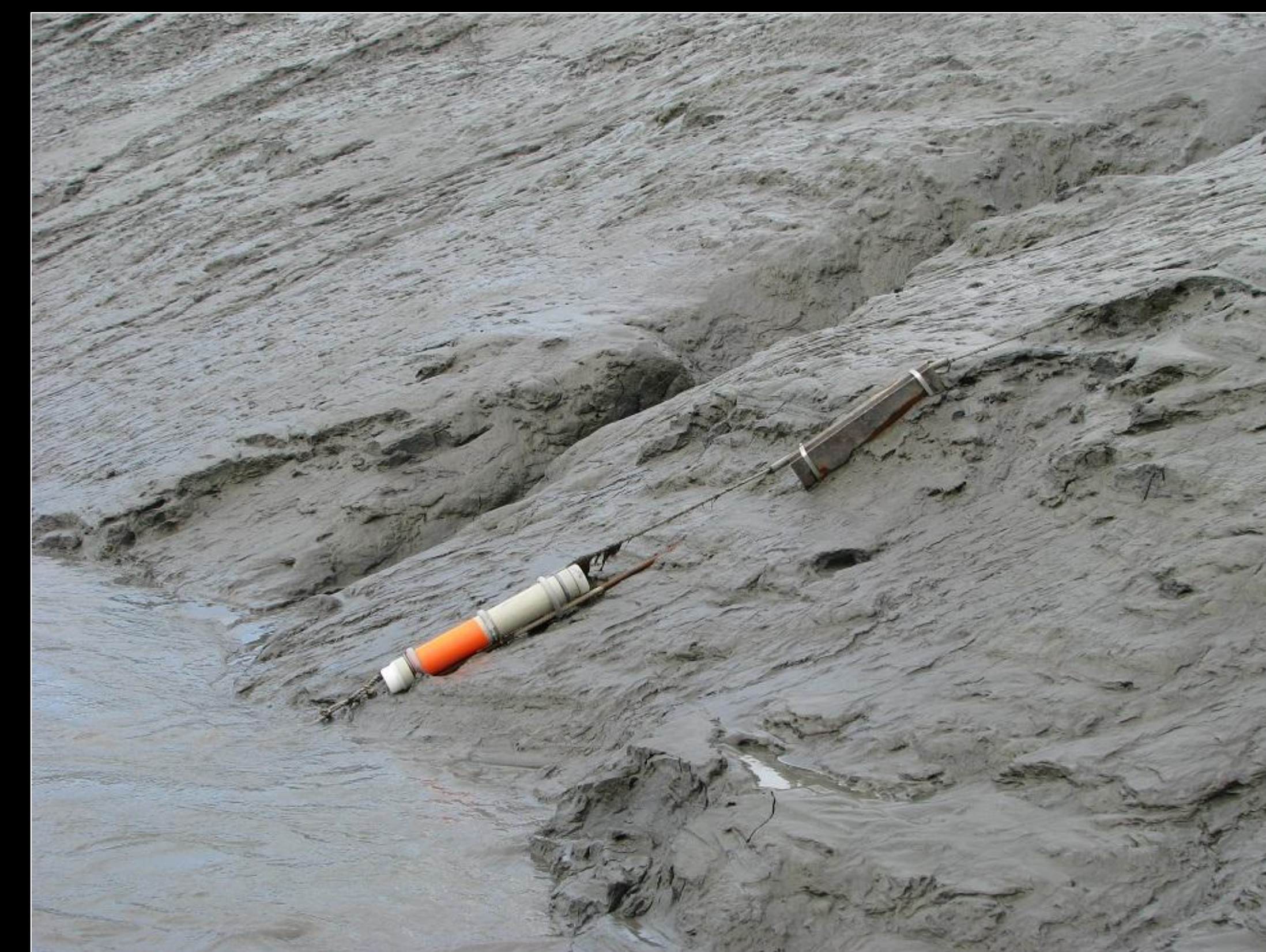
Figure 3: Echolocation logger installed in the river bank at low tide.
