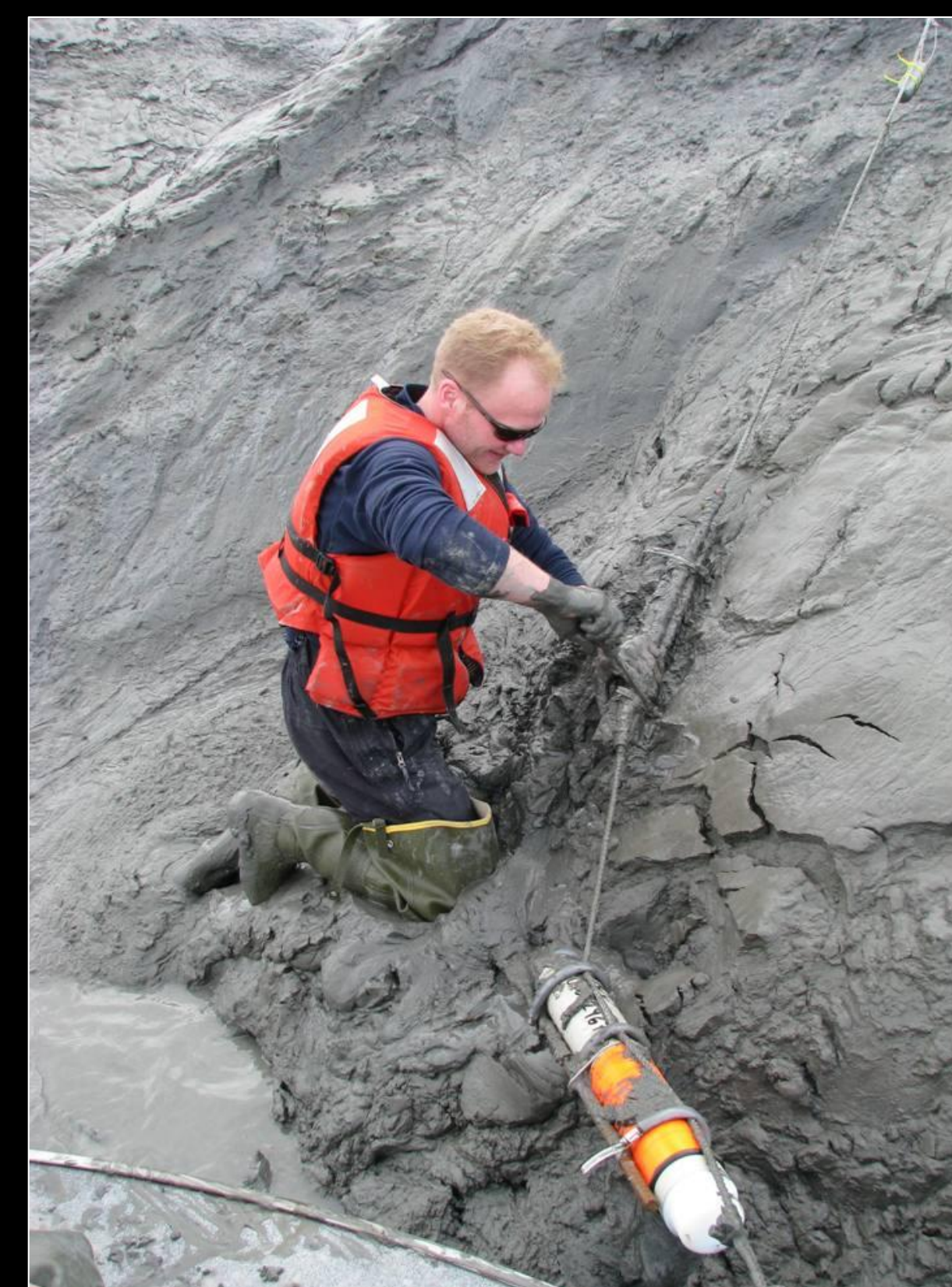
Figure 2: C. Garner installing an echolocation logger in the river bank at low tide.
