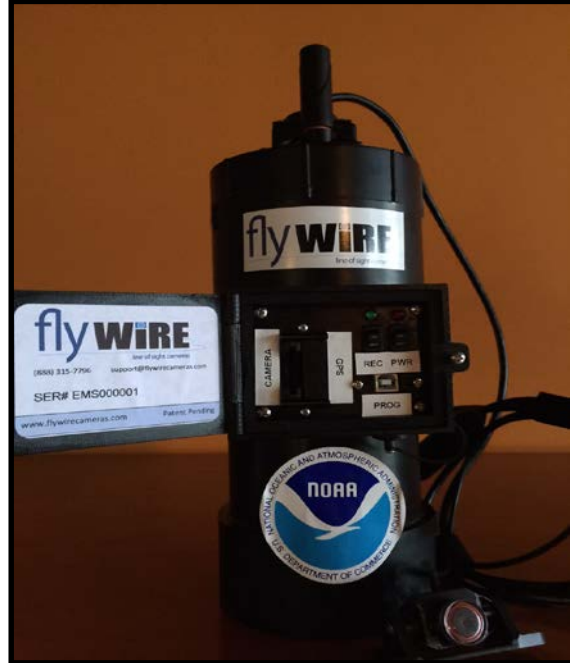
Figure 2. Flywire Unit for Small Vessel Electronic Monitoring.
