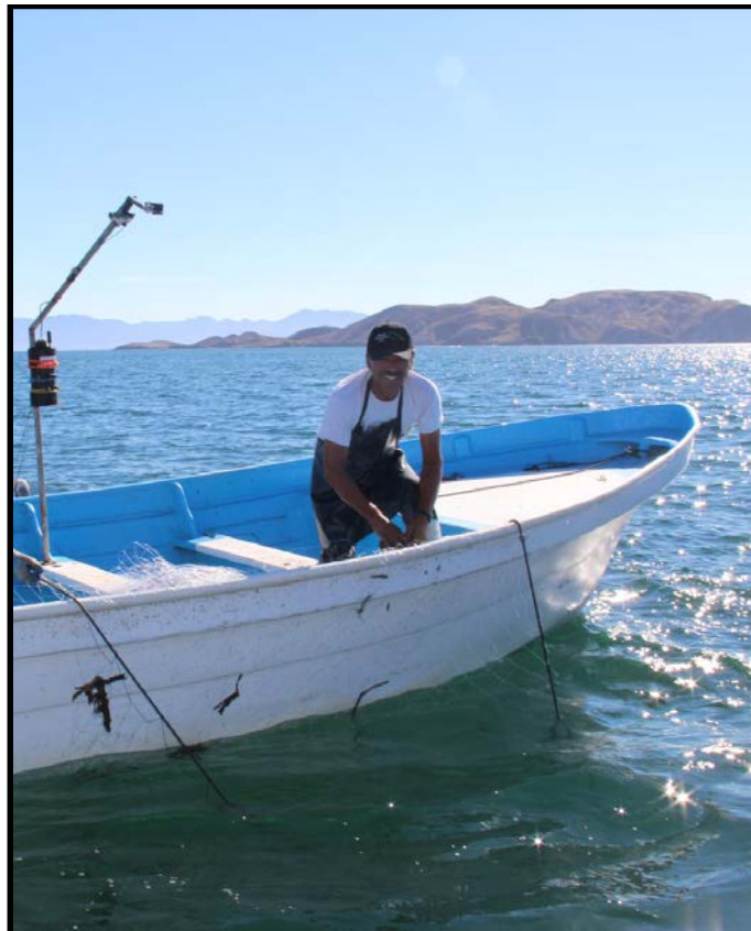
Figure 3. Flywire Camera System on Small Vessel
