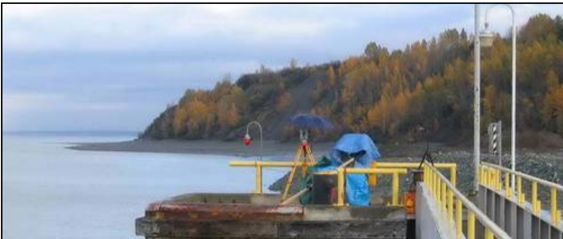
Figure 1.2. These photographs show the monitoring stations at (a) Cairn Point and (b) the Port of Anchorage with the computer-linked theodolite facing in the direction of the Phase 1 North Backlands expansion site from both vantages.
