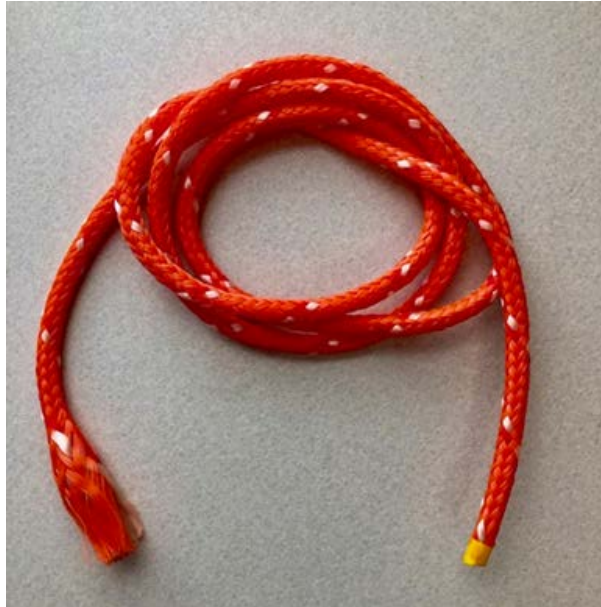
South Shore Sleeve, other weak inserts include spliced in 5/16 th rope and other devices that break at 1700 lbs.
