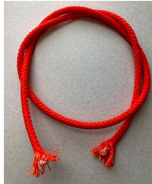
Examples of “weak” rope obtained for testing by the Massachusetts Lobstermen’s Association: Ketchum rope and Shippagan rope
