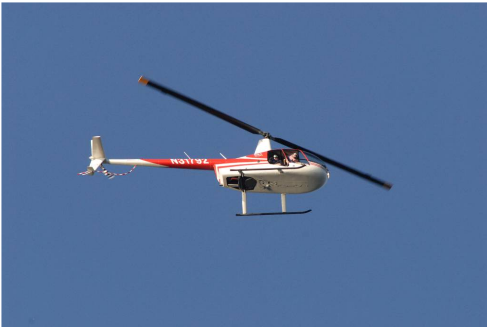
Figure 1: The Robinson R44 clipper helicopter used to obtain aerial photogrammetric images, with the pilot (forward) and photographer (rear) leaning out of the open doors to spot surfacing whales.
