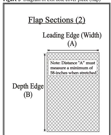
Figure 3 Diagram of exit hole cover piece (flap)
