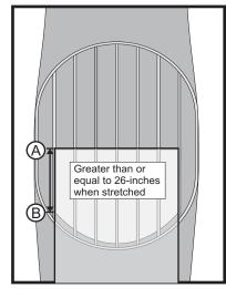
Measure the distance from the TED frame forward along the side of the escape hole cut to the leading edge of the escape hole cut **A to B**.
