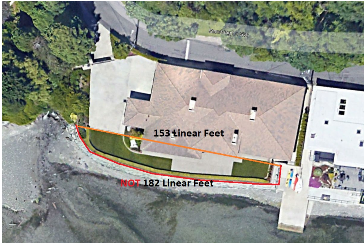
Figure 17: Determination of Length of Shoreline Stabilization.
