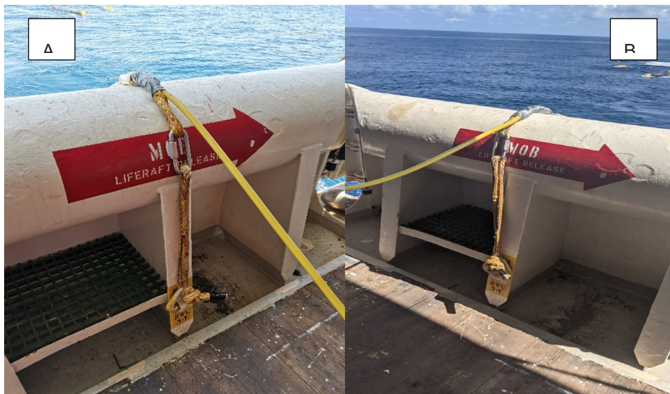
Figure 4. Chinese finger secured to the anchoring rope. (A) Chinese finger at 50m (B) Chinese finger at 120m
