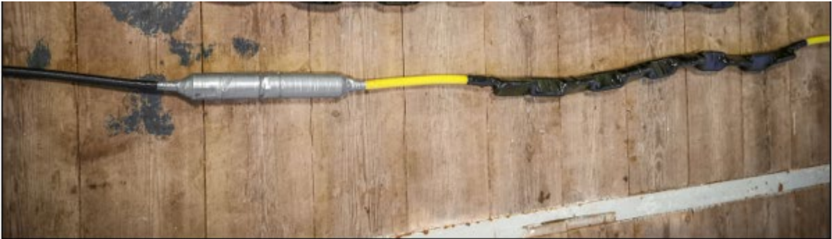
Figure 1: Chain secured to tow/hydrophone cable.
