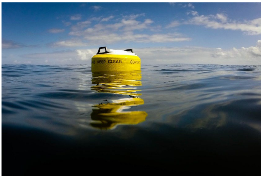
A hypoxia buoy floats in the Chesapeake Bay; photo by NOAA Chesapeake Bay Office
