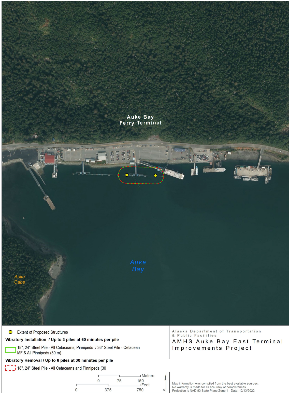
Figure 6-1. Shutdown Zones during Vibratory Pile Installation and Removal at Auke Bay East Ferry Terminal
