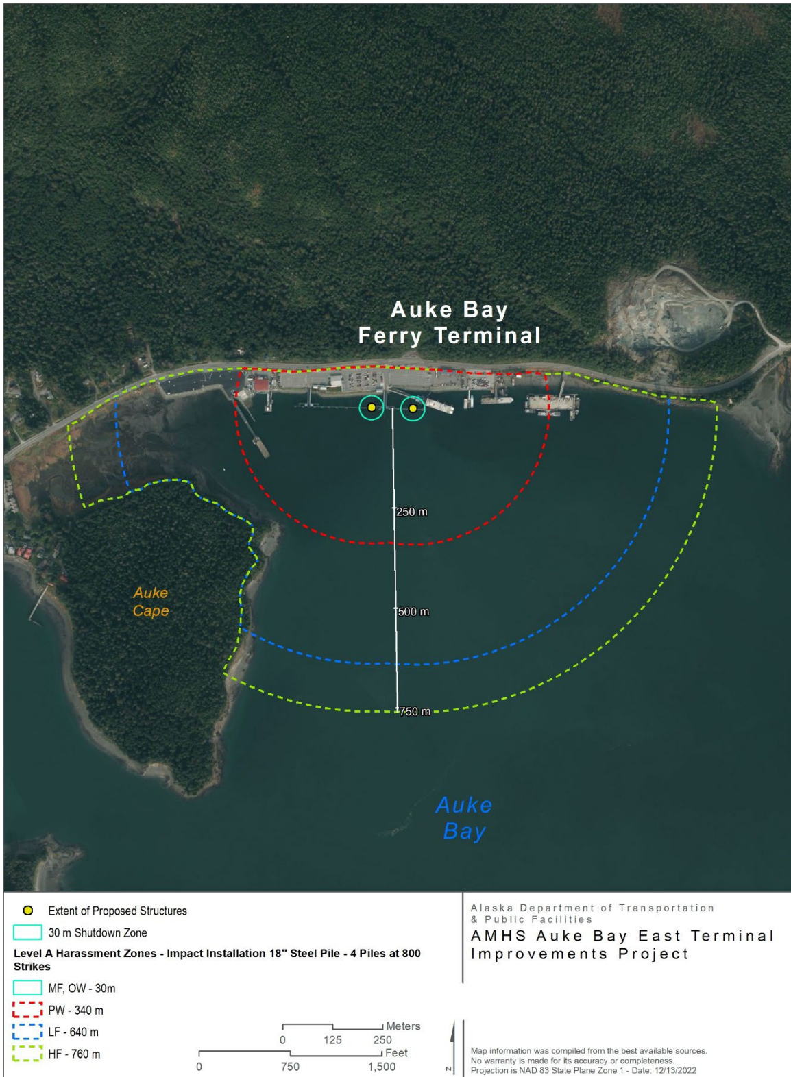
Figure 2-3. Largest Level A Harassment Zones during Impact Installation of 18-inch Steel Piles (four piles at 800 strikes each)
