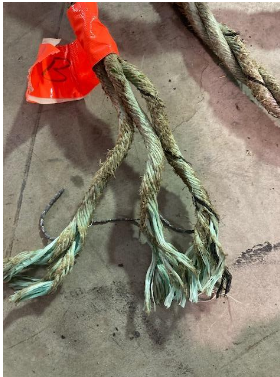
E04-23 image – Beaded lead in sink line.
