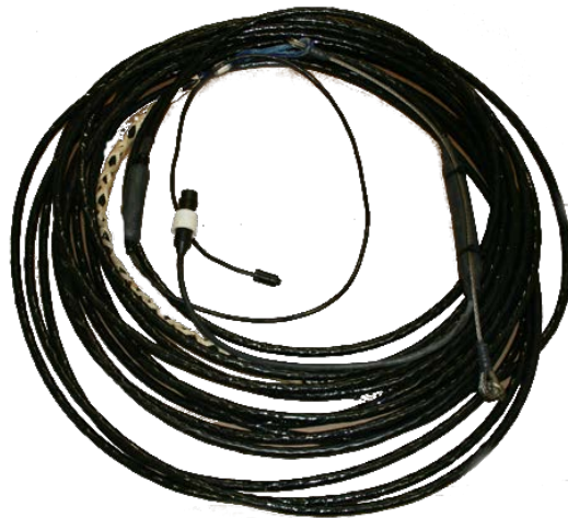
Figure 1-4: 35-Meter Kevlar Reinforced Tow Cable
