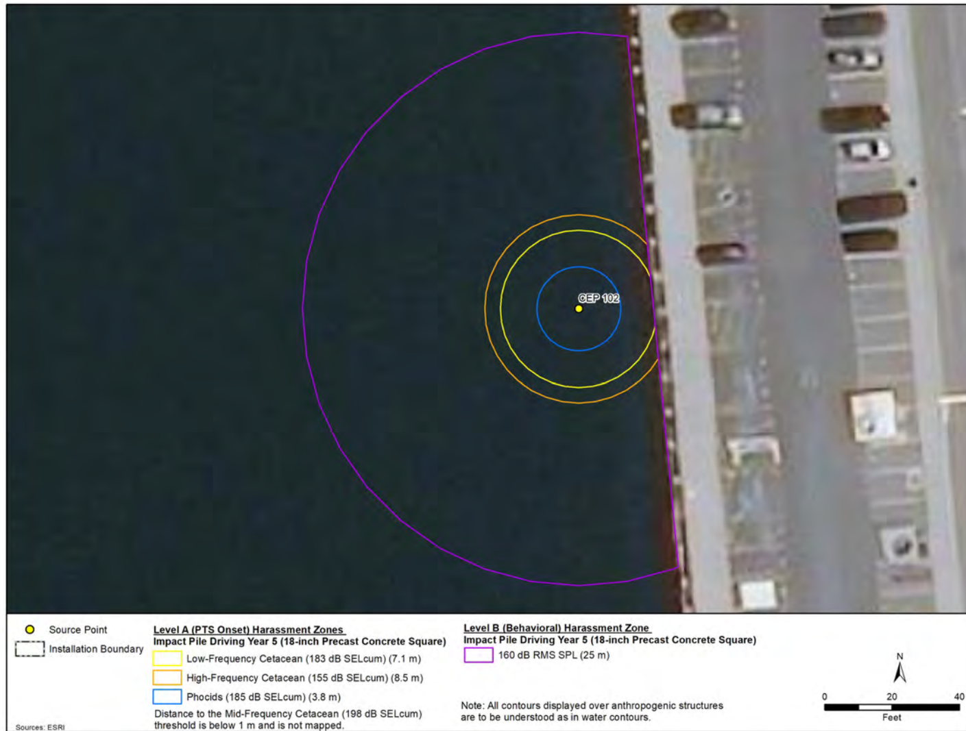
Figure 6-17 Year 5-Maximum Distance to Level A (PTS Onset) and Level B (Behavioral) Harassment Zones from Impact Pile Driving 18-inch Square Precast Concrete Piles at CEP-102 Platform Center
