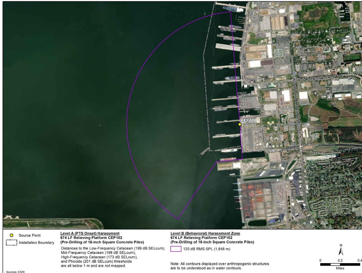
Figure A-8: ZOIs For Level A (PTS Onset) & Level B (Behavioral) Harassment From Vibratory Pile Driving At CEP 102 – 18-Inch Square Concrete
