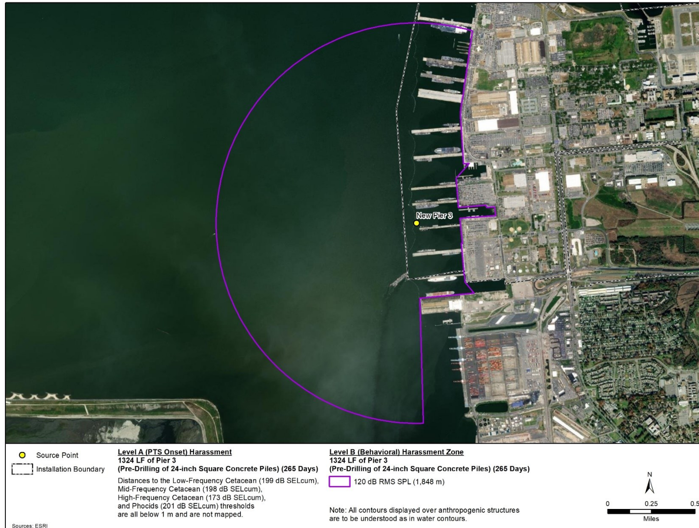
Figure A-23: ZOIs For Level A (PTS Onset) & Level B (Behavioral) Harassment From Vibratory Pile Driving At New Pier 3 – 24-Inch Square Concrete 265 Days
