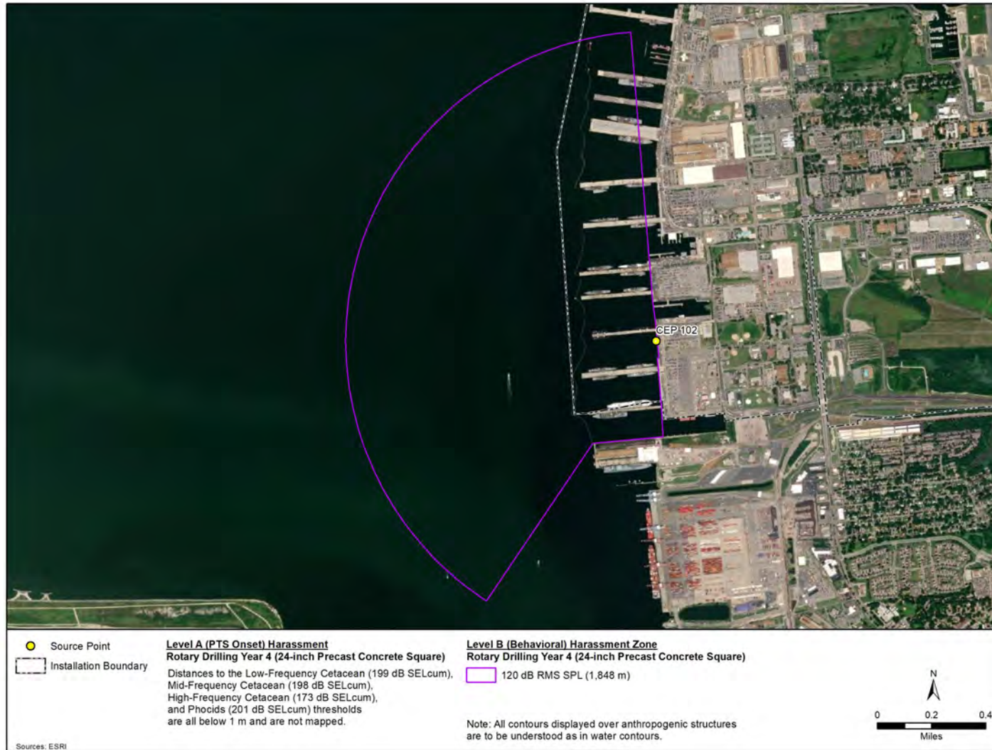
Figure 6-33 Year 4- Maximum Distance to Level B (Behavioral) Harassment Zone from Rotary Drilling for 24-inch Square Precast Concrete Piles at CEP-102 Center Platform
