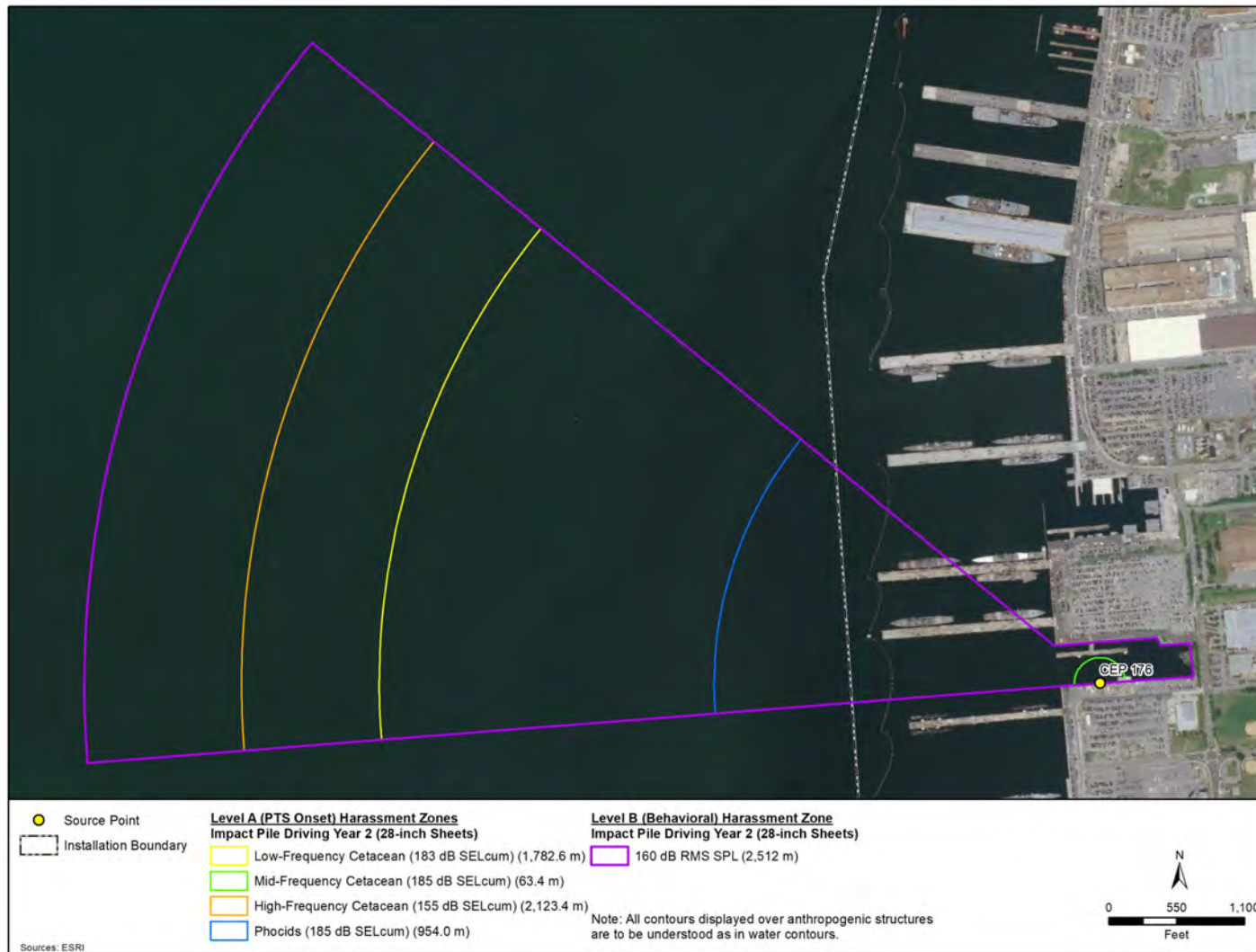
Figure 6-2 Year 2-Maximum Distance to Level A (PTS Onset) and Level B (Behavioral) Harassment Zones from Impact Pile Driving 28-inch Steel Sheet Piles at CEP-176 Bulkhead
