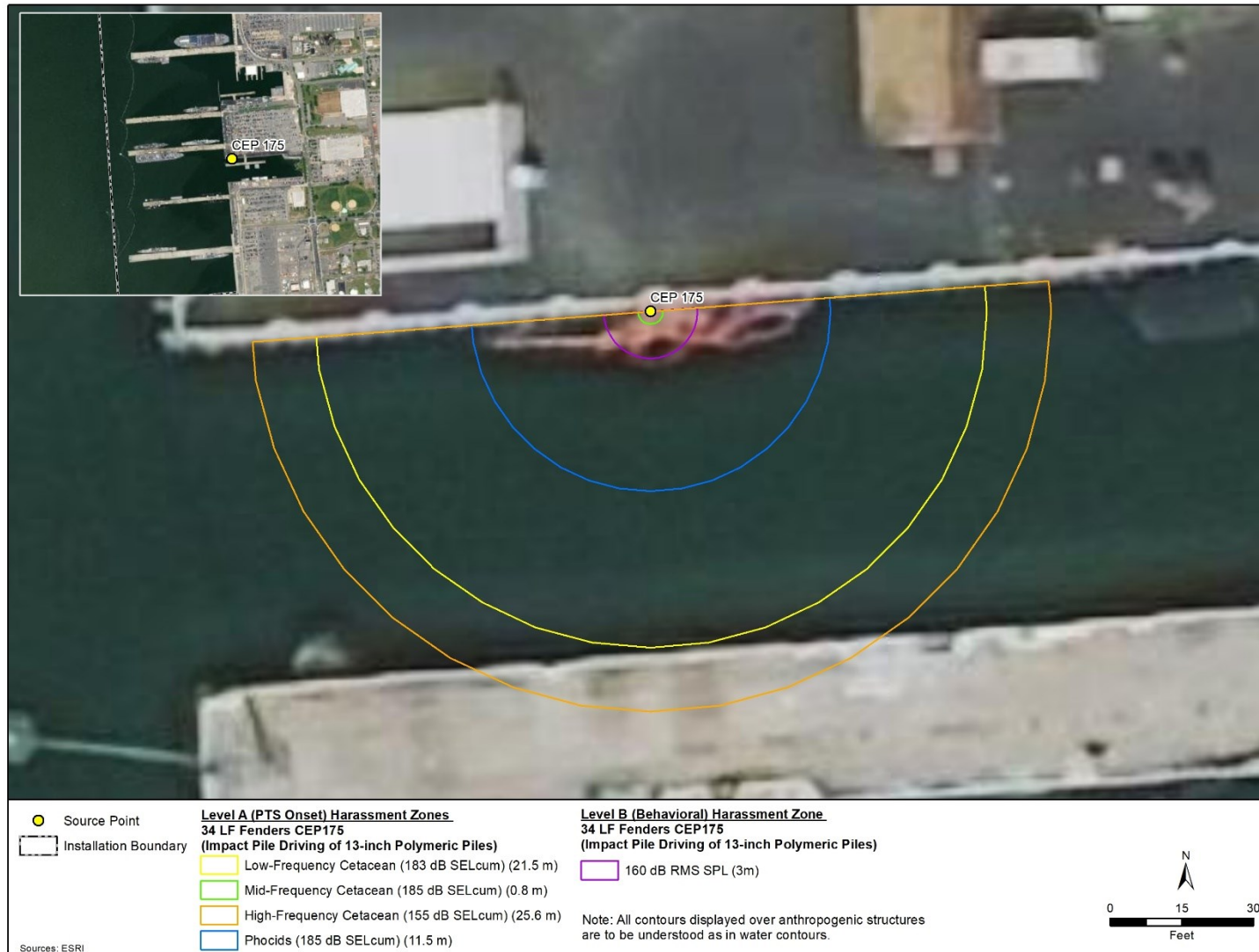
Figure A-12: ZOIs For Level A (PTS Onset) & Level B (Behavioral) Harassment From Impact Pile Driving At CEP 175 – 13-Inch Polymeric
