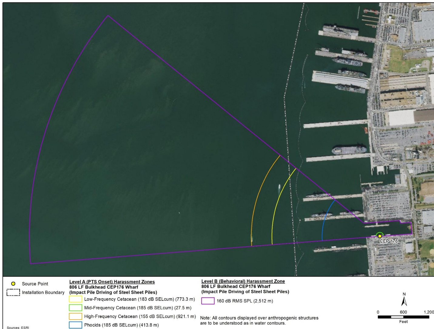
Figure A-15: ZOIs For Level A (PTS Onset) & Level B (Behavioral) Harassment From Impact Pile Driving At CEP 176 – Steel Sheet
