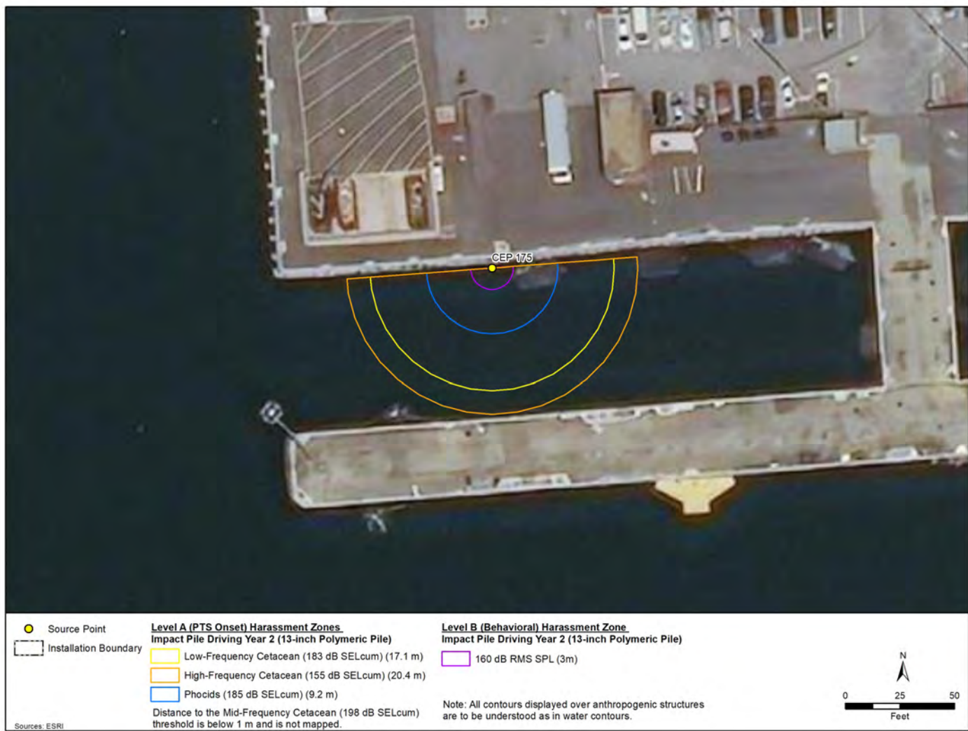
Figure 6-3 Year 2-Maximum Distance to Level A (PTS Onset) and Level B (Behavioral) Harassment Zones from Impact Pile Driving 13-inch Polymeric Piles at CEP-175 Bulkhead
