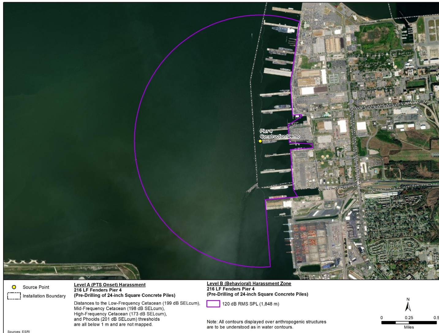
Figure A-31: ZOIs For Level A (PTS Onset) & Level B (Behavioral) Harassment From Vibratory Pile Driving At Pier 4 – 24-Inch Square Concrete
