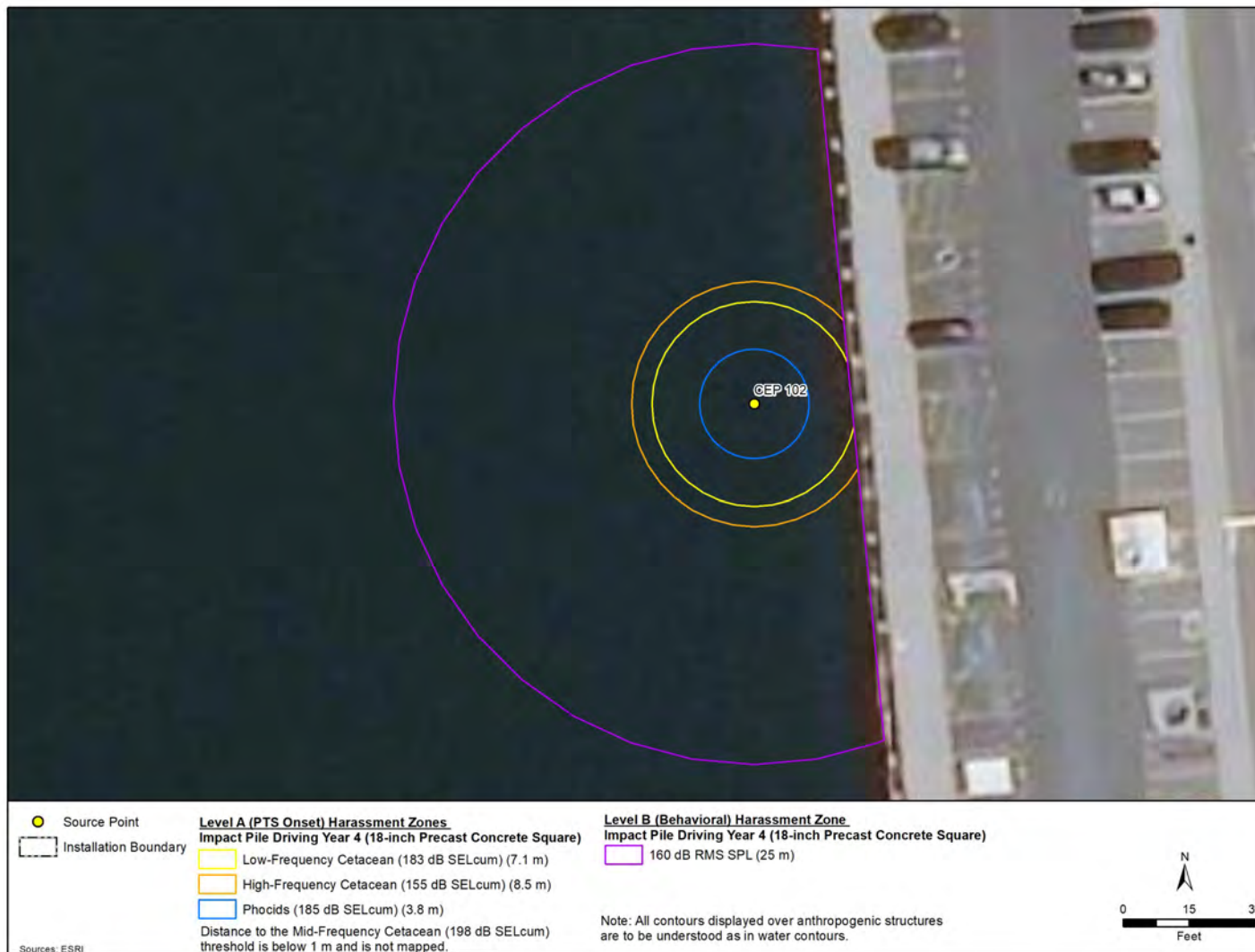
Figure 6-12 Year 4-Maximum Distance to Level A (PTS Onset) and Level B (Behavioral) Harassment Zones from Impact Pile Driving 18-inch Square Precast Concrete Piles at CEP-102 Platform Center
