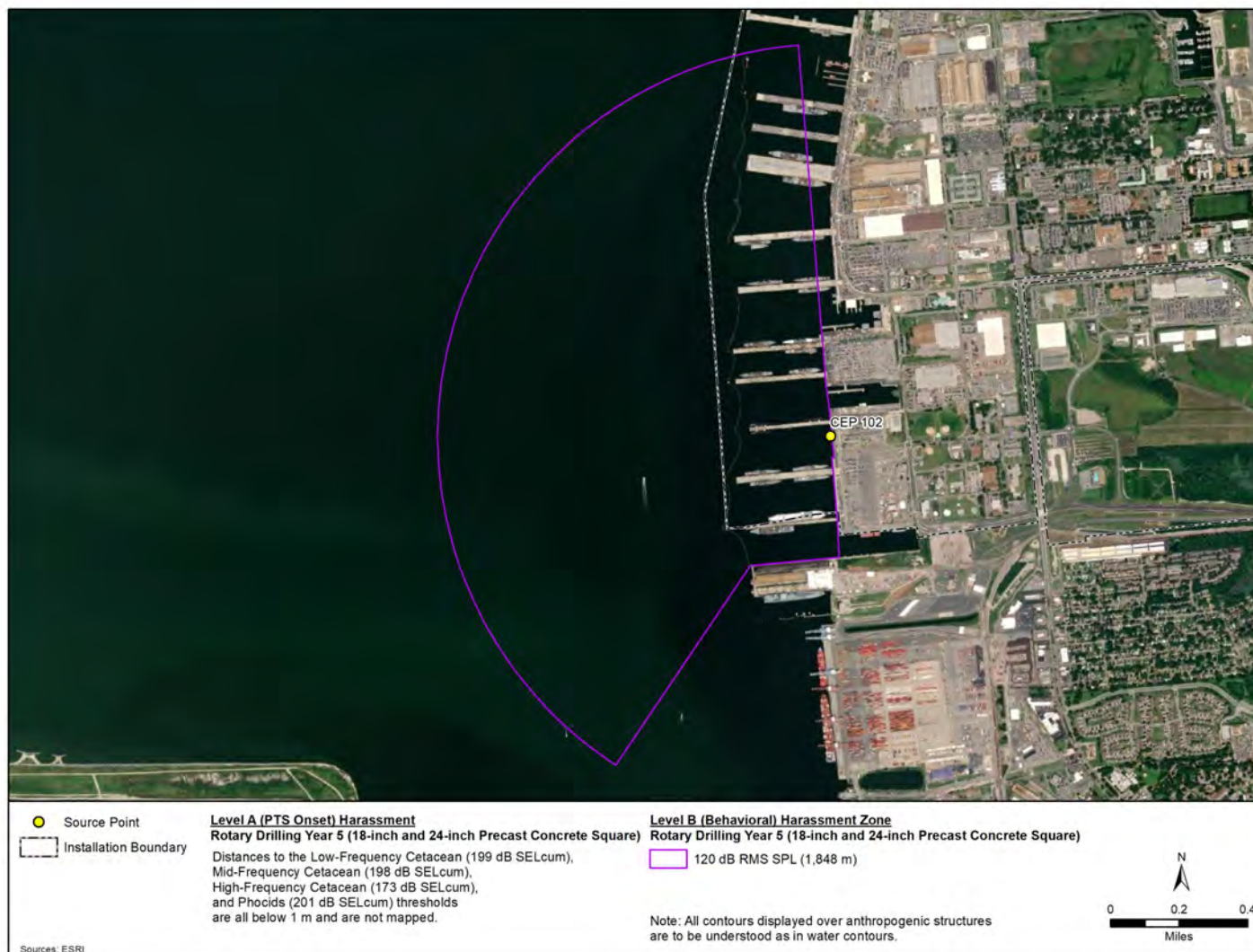
Figure 6-34 Year 5-Maximum Distance to Level B (Behavioral) Harassment Zone from Rotary Drilling for 18-inch and 24-inch Square Precast Concrete Piles at CEP-102 Center Platform
