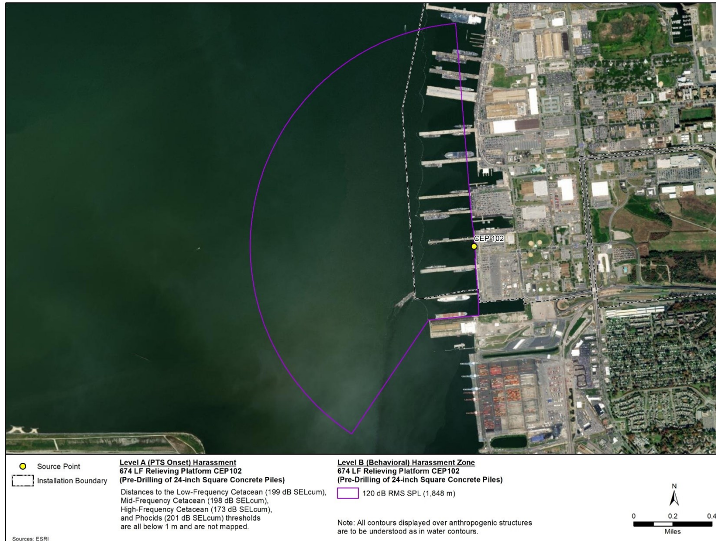
Figure A-9: ZOIs For Level A (PTS Onset) & Level B (Behavioral) Harassment From Vibratory Pile Driving At CEP 102 – 24-Inch Square Concrete
