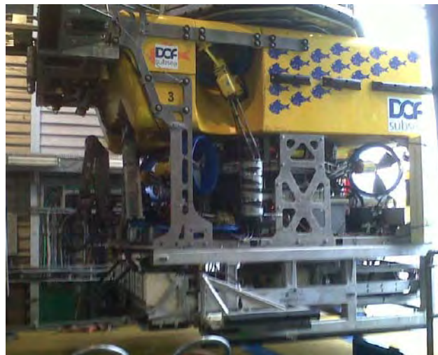
Figure 1: Sub-Bottom Imager™ (complete SBI equipment on an ROV skid (top panel) and SBI on a WROV bottom skid with multibeam also onboard (bottom panel)
