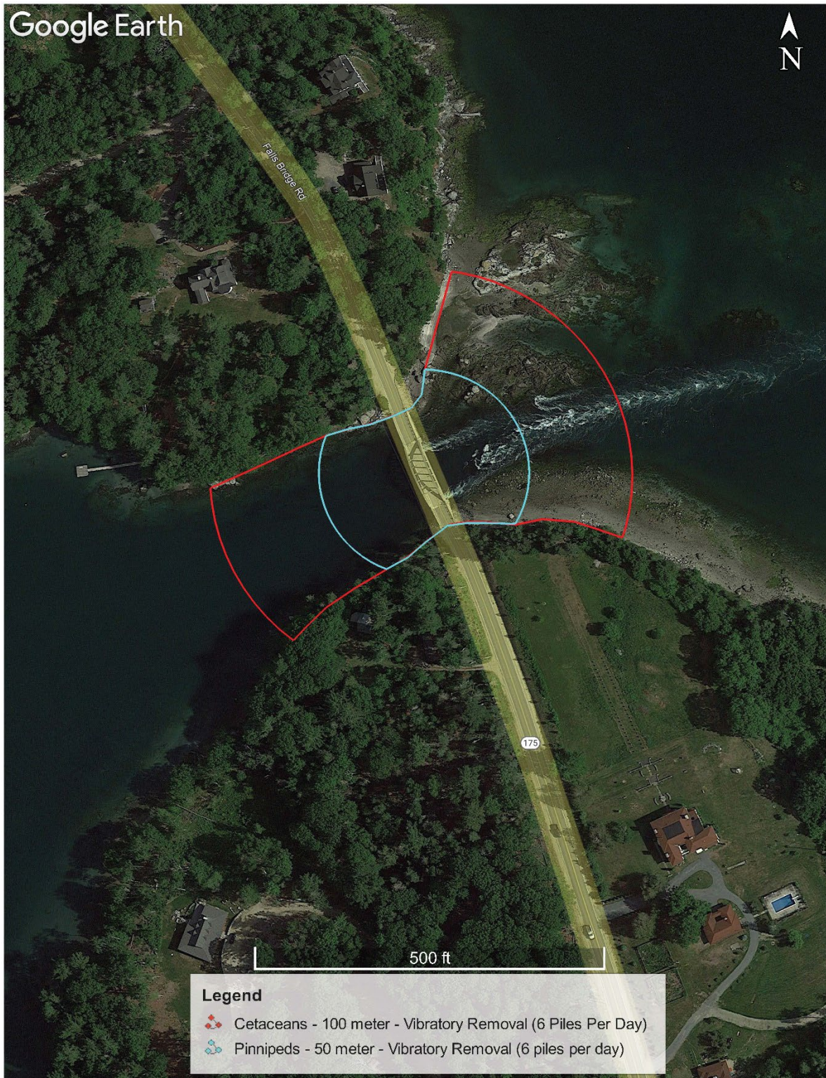
Figure 1-1. Shutdown Zones for Cetaceans and Pinnipeds during Vibratory Pile Removal for Falls Bridge Replacement Project
