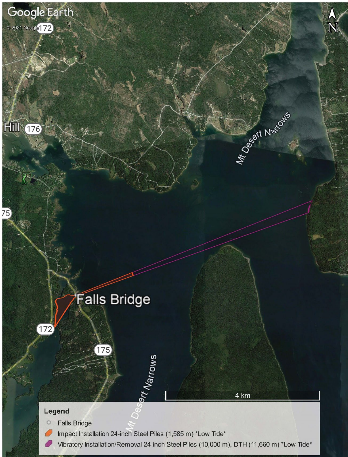
Figure 2–4. Level B Harassment Zones (and shutdown zones for species not covered by this IHA) during Pile Installation and Removal at Low Tide for Falls Bridge Replacement Project
