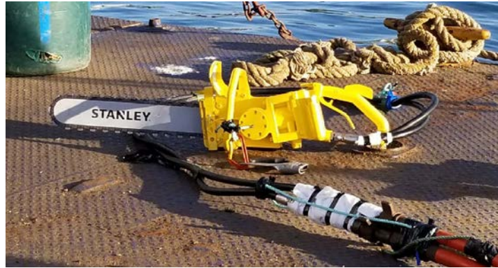
Figure 38. Hydraulically-Actuated Underwater Chainsaw.
