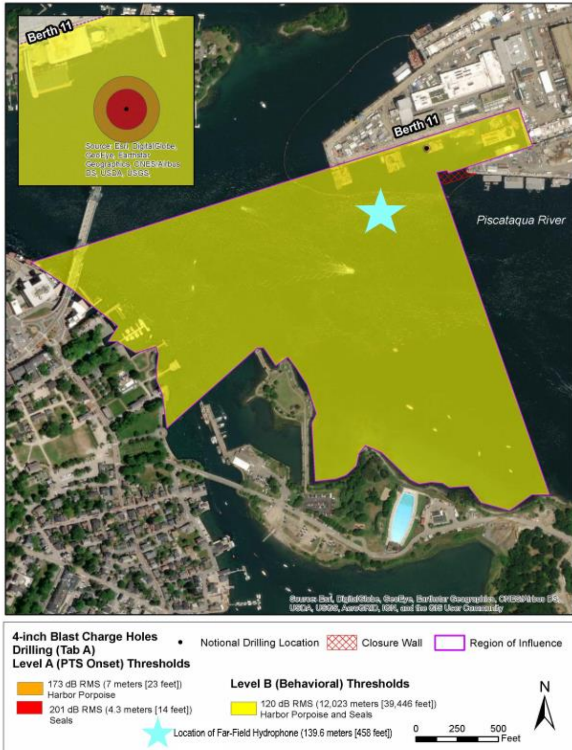
Figure 11. Representative Far-Field Monitoring Location for Underwater Pile Driving Noise from Drilling Activities
