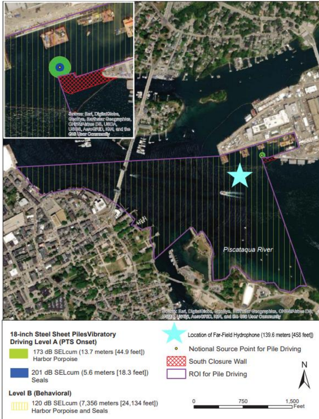
Figure 10. Representative Far-Field Monitoring Location for Underwater Pile Driving Noise from Vibratory Driving of 18-inch, Flat-Webbed Sheet Piles*
