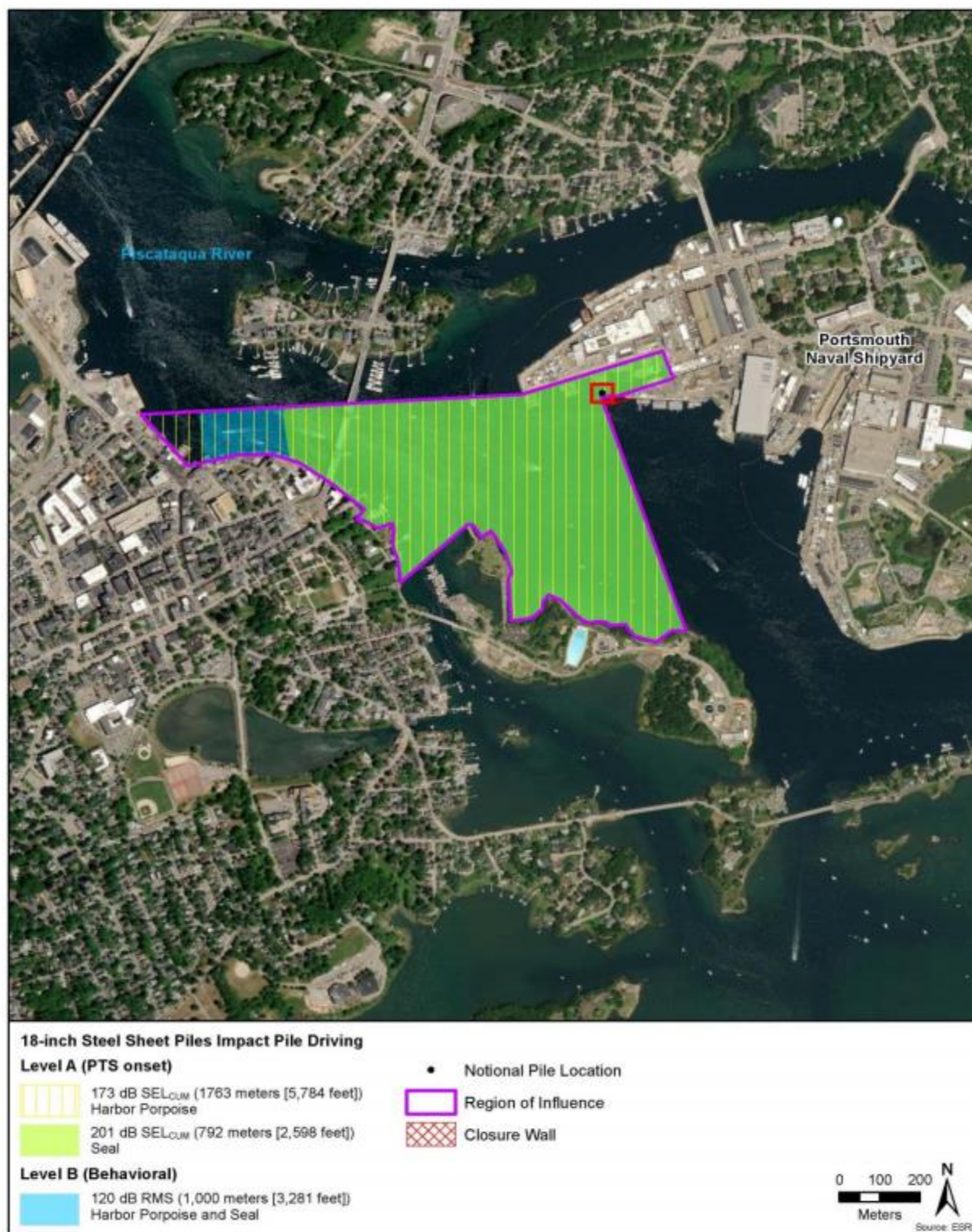
Figure 18. Distances to Level A and Level B from Impact Driving of 18-inch, Flat-Webbed Sheet Piles
