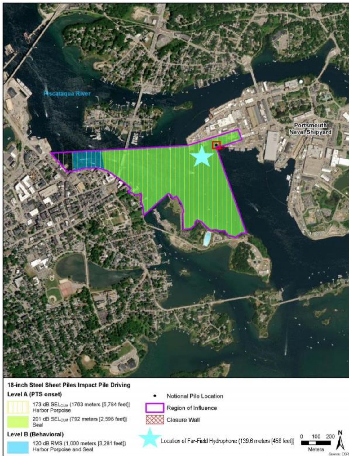
Figure 9. Representative Far-Field Monitoring Location for Underwater Pile Driving Noise from Impact Driving of 18-inch, Flat-Webbed Sheet Piles*
