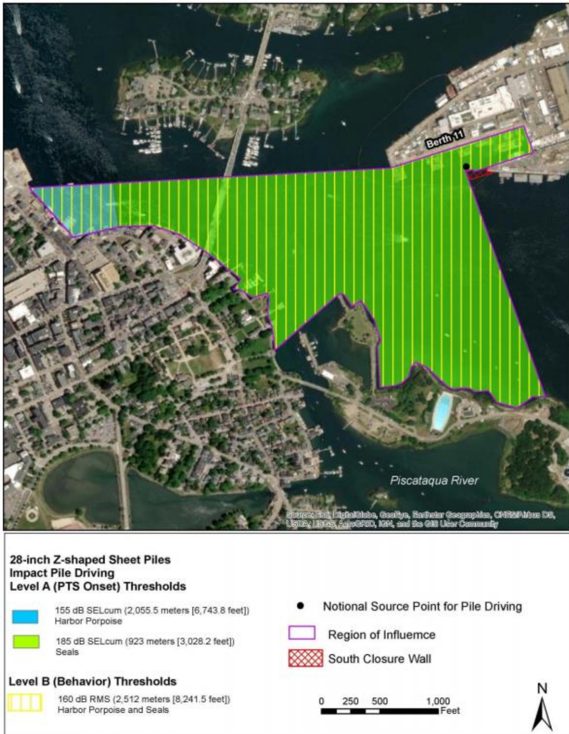
Figure 15. Distances to Level A and Level B from Impact Driving of 28-inch, Z-shaped Sheet Piles
