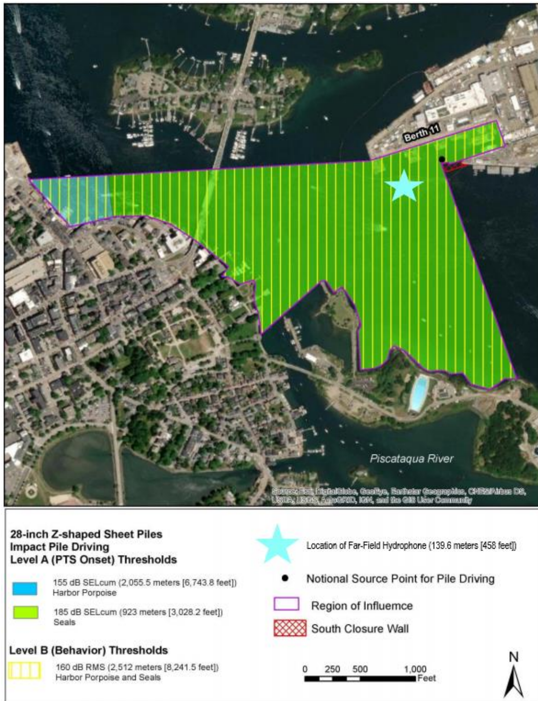
Figure 6. Representative Far-Field Monitoring Location for Underwater Pile Driving Noise from Impact Driving of 28-inch, Z-shaped Sheet Piles*
