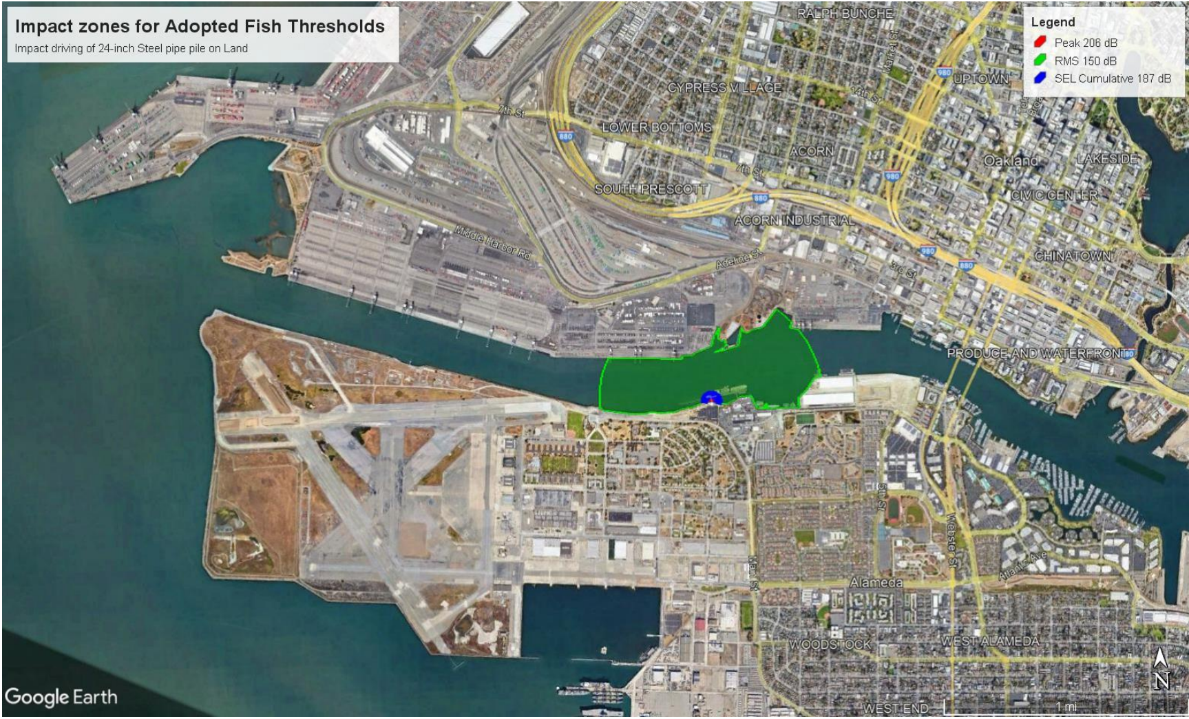
Figure A1 – Fish Injury Zones – 206 dB Peak, 150 dB RMS and 187 SEL cum ; for 24-inch Steel pile on Land impact driven
