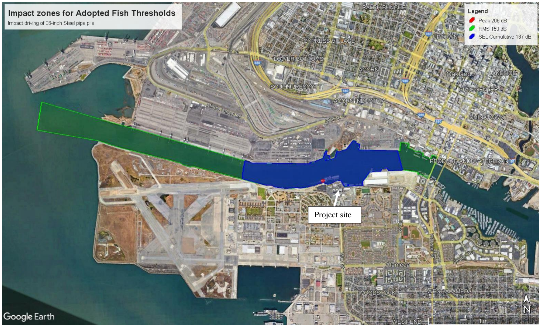
Figure A2 – Fish Injury Zones – 206 dB Peak, 150 dB RMS and 187 SEL cum ; for 36-inch Steel pile impact driven
