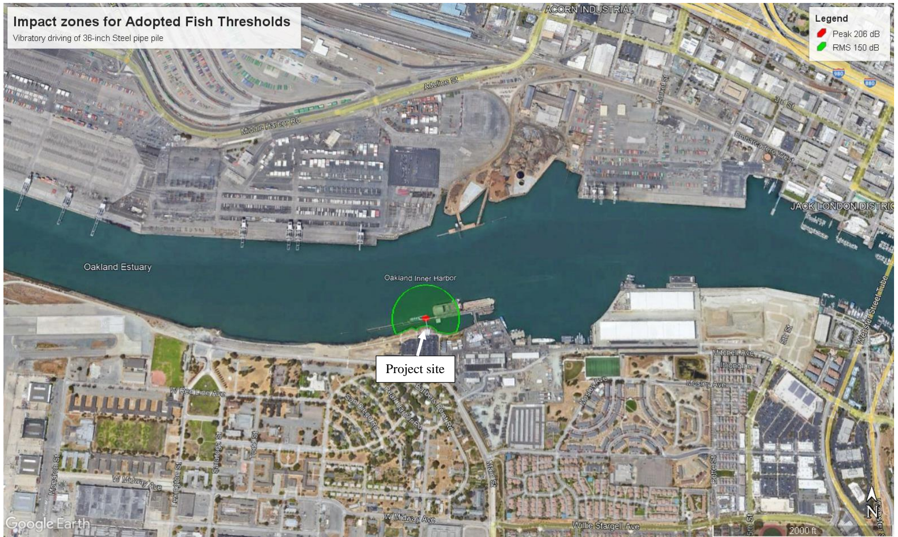
Figure A5 – Fish Injury Zones – 206 dB Peak, 150 dB RMS and 187 SEL cum ; for 36-inch Steel pile driven using a vibratory hammer
