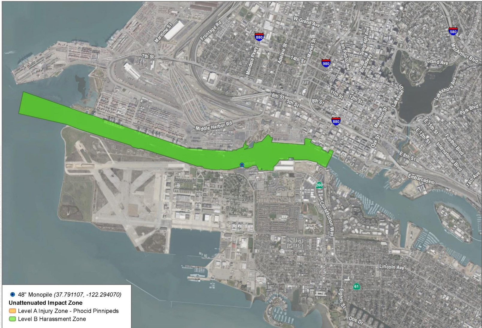
FIGURE 8 Marine Mammal Thresholds Level A and B Impact Zones - 48-inch Monopile: Driven with Vibratory Hammer
