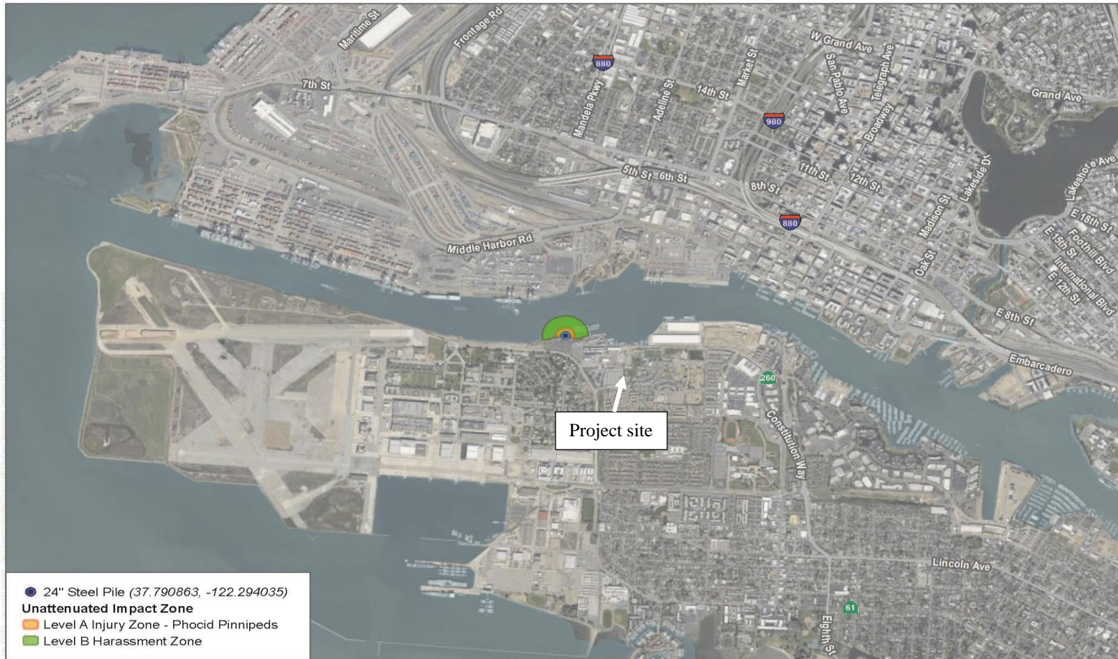
FIGURE 3 Marine Mammal Thresholds Level A and B Impact Zones - 24-inch Steel Pile: Land Impact Driven Alameda Main Street Terminal Refurbishment Project
