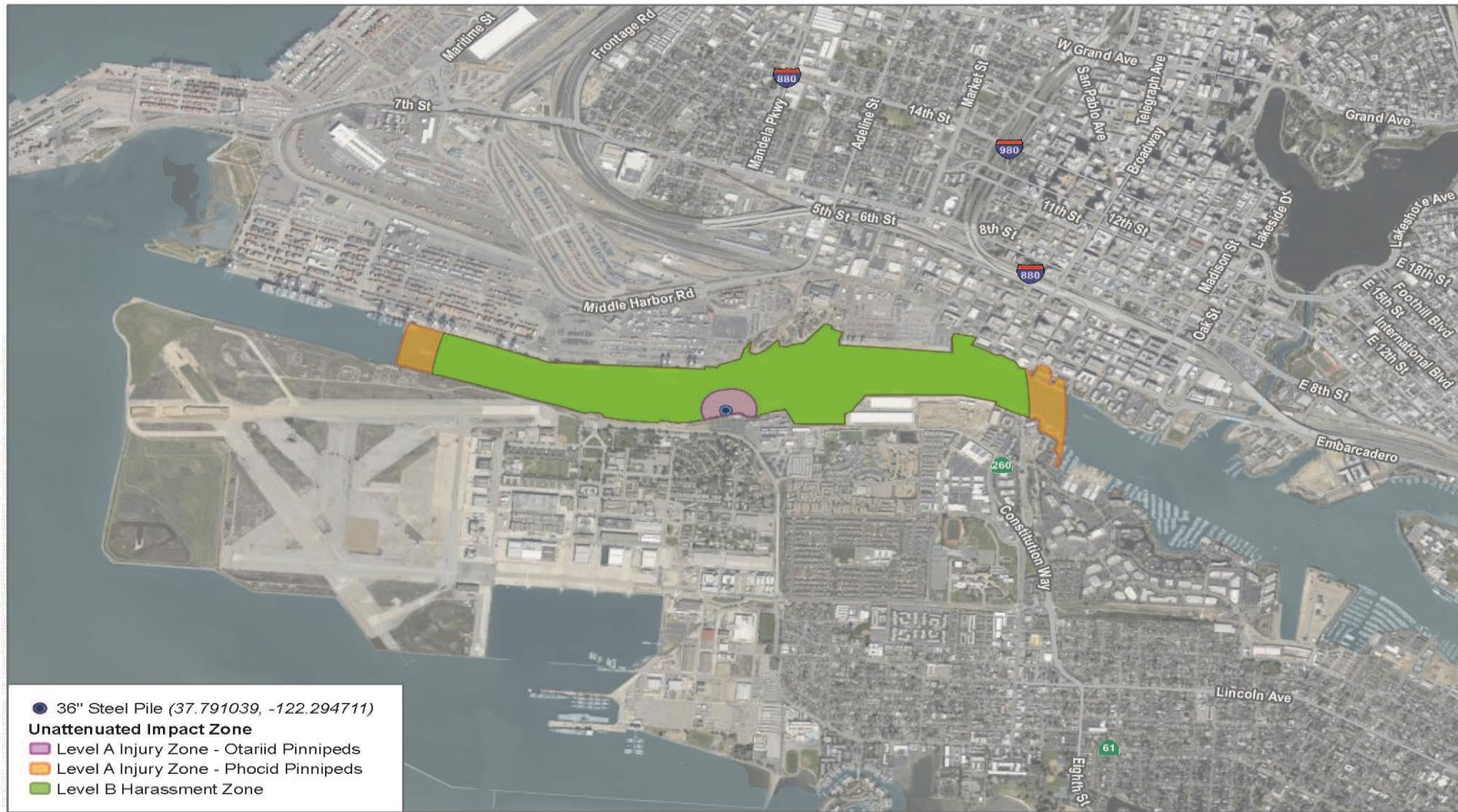
FIGURE 4A Marine Mammal Thresholds Level A and B Impact Zones - 36-inch Steel Pile: Impact Driven Alameda Main Street Terminal Refurbishment Project
