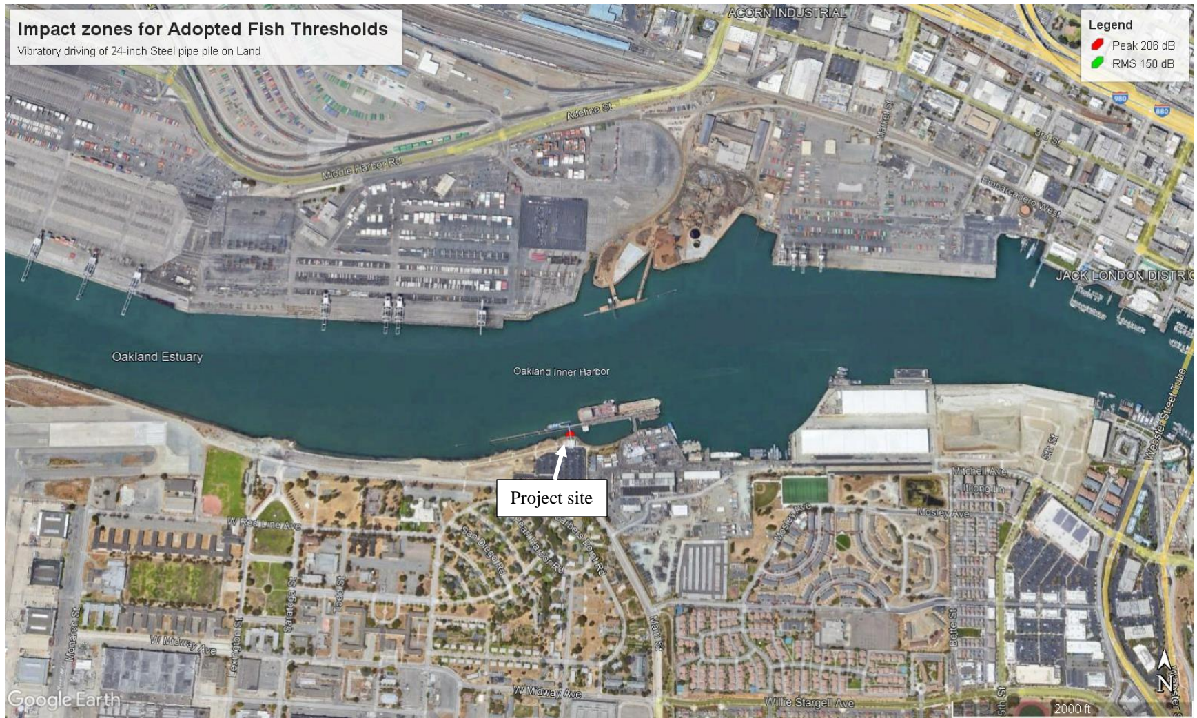
Figure A4 – Fish Injury Zones – 206 dB Peak, 150 dB RMS and 187 SEL cum ; for 24-inch Steel pile on Land driven using a vibratory hammer
