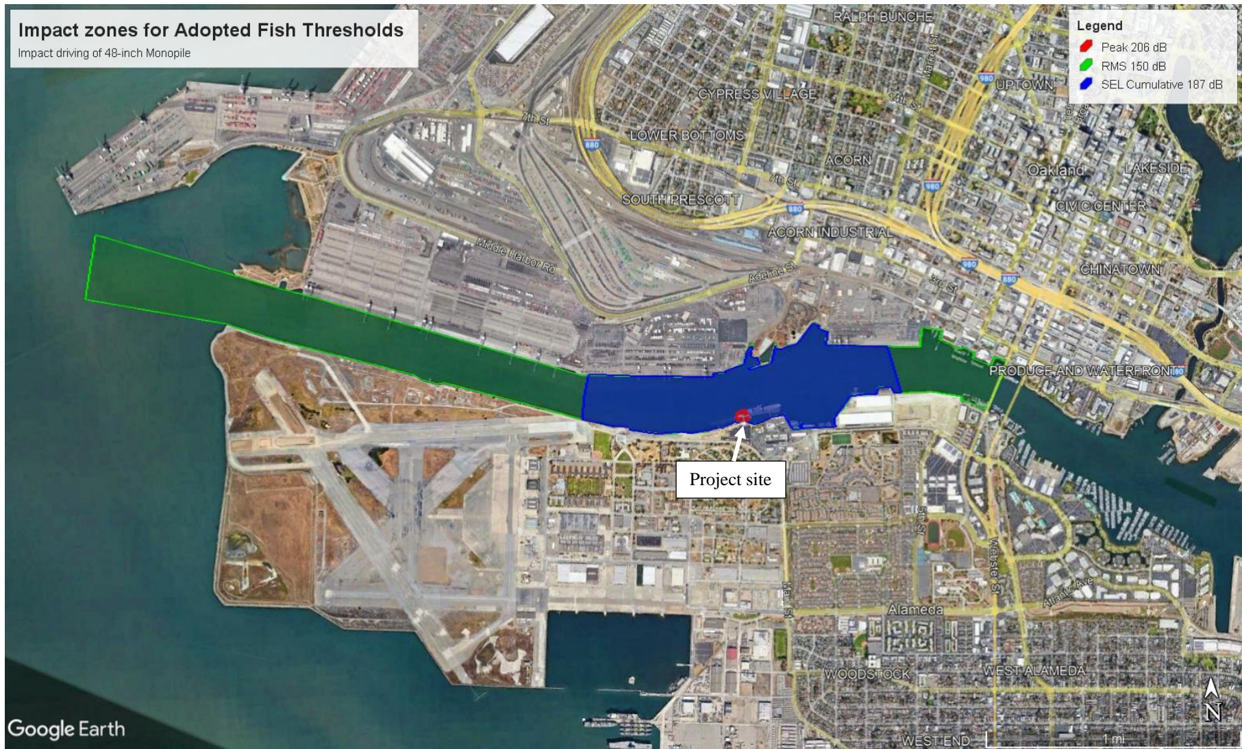
Figure A3 – Fish Injury Zones – 206 dB Peak, 150 dB RMS and 187 SEL cum ; for 48-inch monopile impact driven
