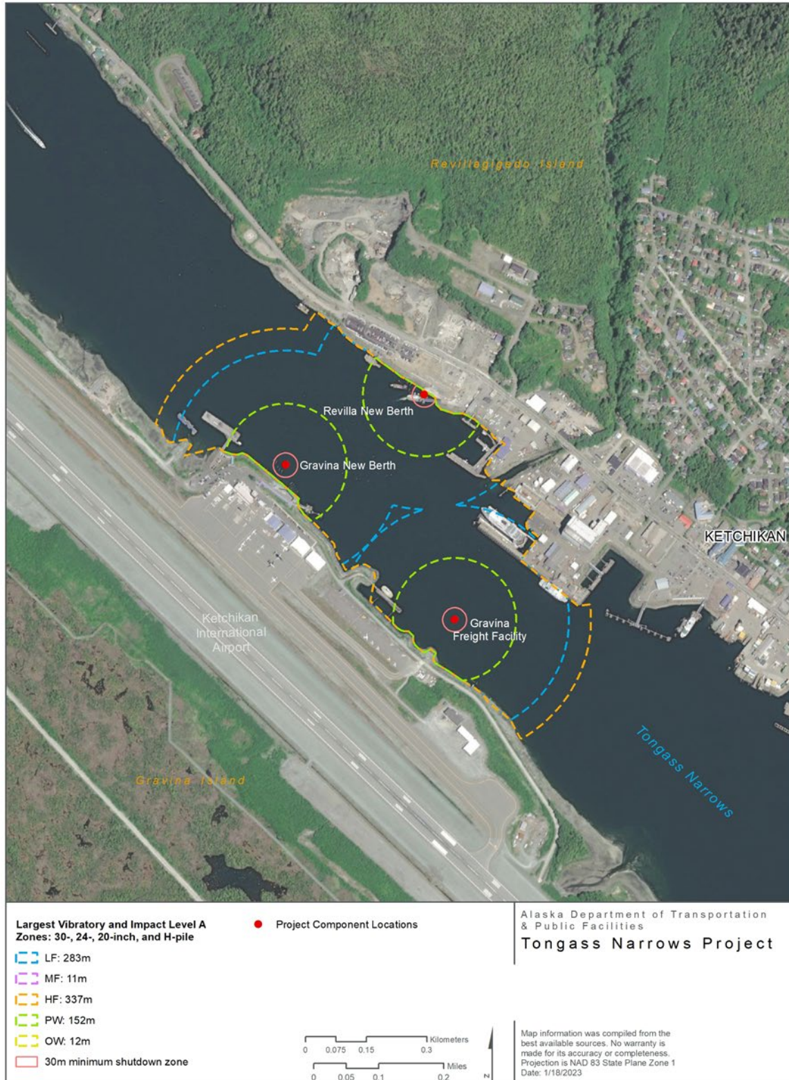
Figure 2-1. Level A Zones and 30-meter Shutdown Zone during Impact and Vibratory Pile Installation and Removal at Representative Project Components
