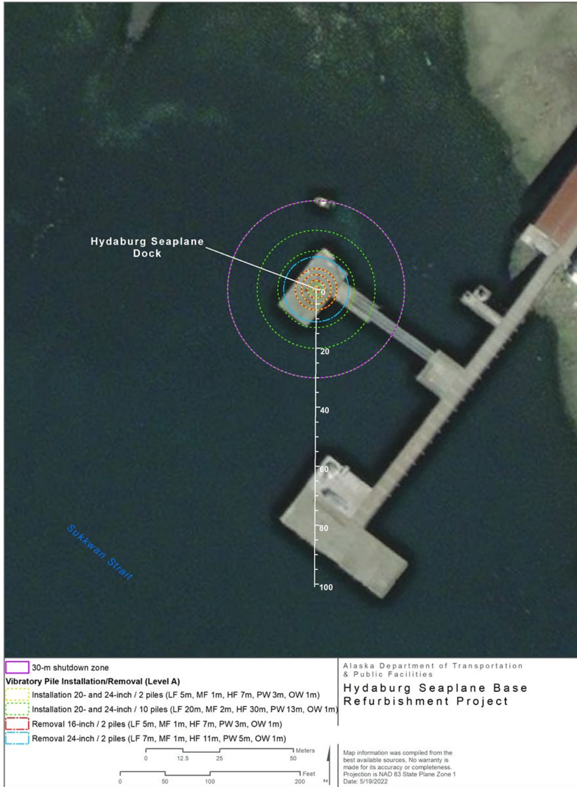
Figure 2-2. Level A Harassment Isopleths for Vibratory Pile Installation or Removal
