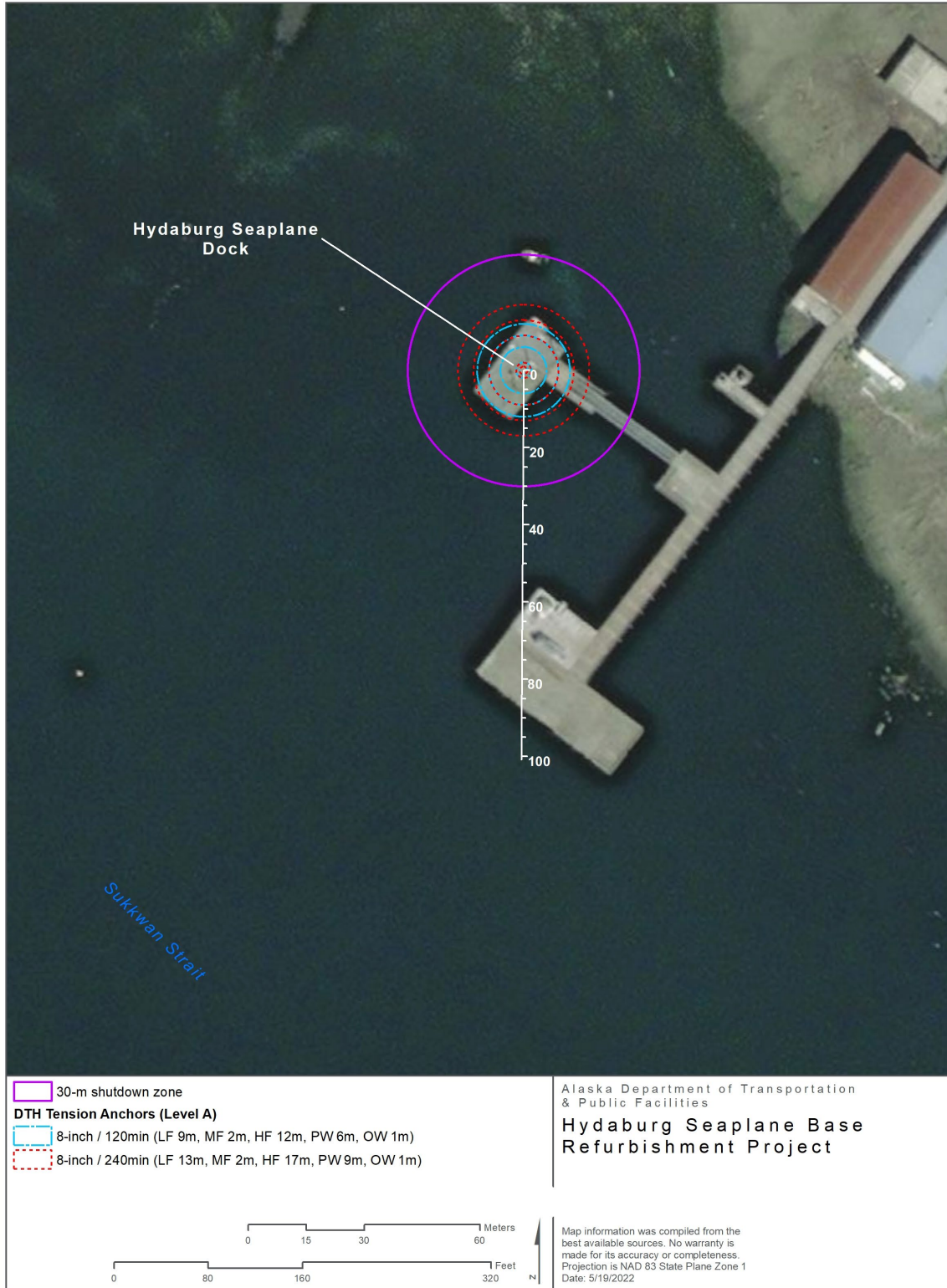
Figure 6-4. Level A Harassment Zones during Tension Anchor Installation at Hydaburg Seaplane Base
