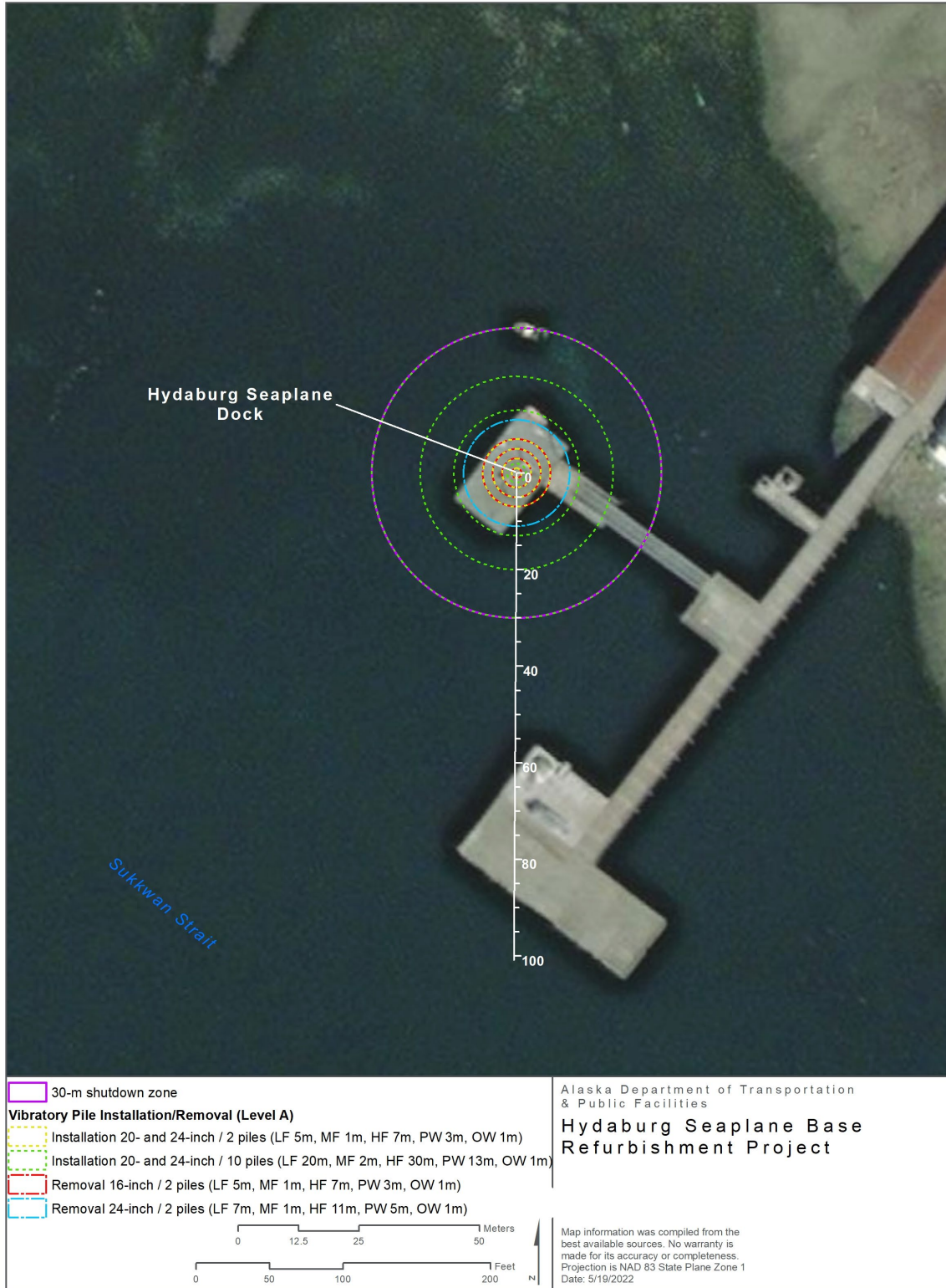
Figure 6-6. Level A Harassment Zones during Vibratory Installation and Removal at Hydaburg Seaplane Base
