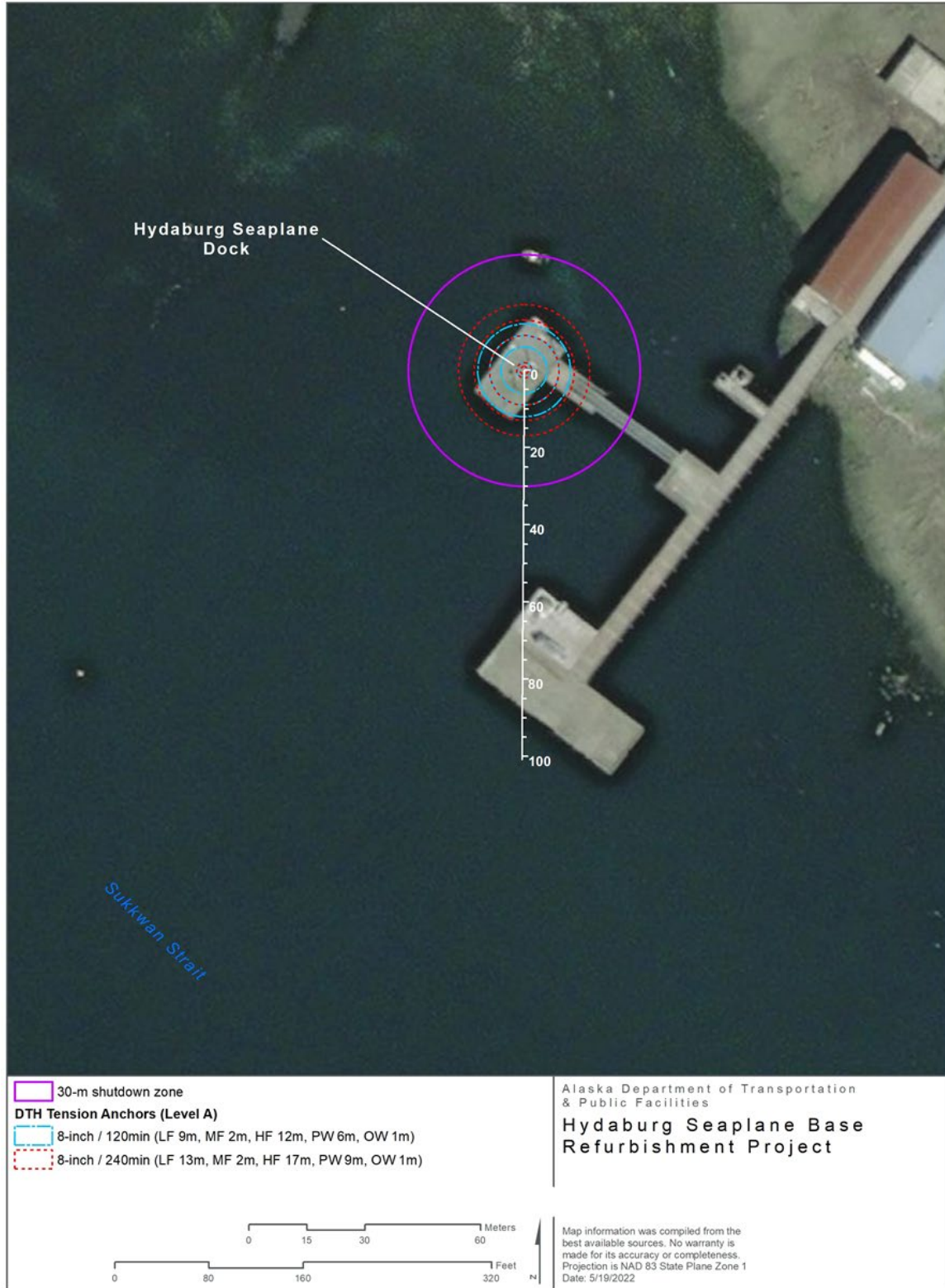
Figure 2-4. Level A Harassment Isopleths during Down-the-Hole Installation of Tension Anchors for 2 and 4 Hours
