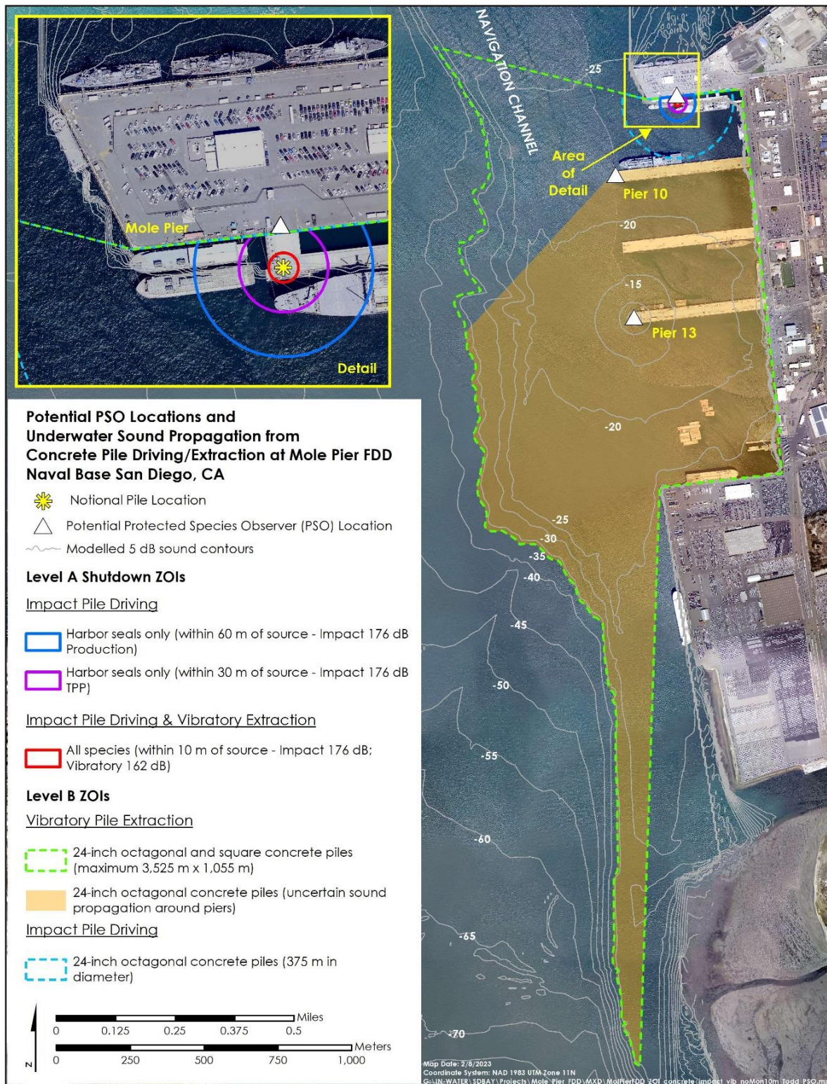
Figure 1-2. Monitoring/Shutdown Zones and Potential Monitor Locations for Proposed Impact and Vibratory Extraction/Installation of Concrete Piles.
