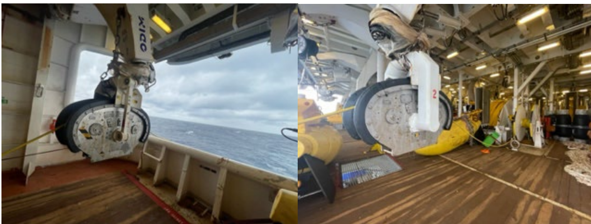
Figure 5-6. Cable guided through a fairlead block.
