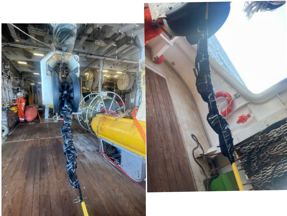
Figure 10-11. Weight added to the tow cable to increase depth.
