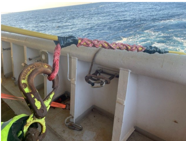
Figure 13. Chinese finger attached to the tow cable and the metallic hook
