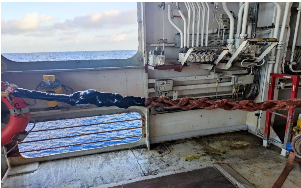
Figure 5. Chinese finger added to the tow cable to help secure it after deployed.
