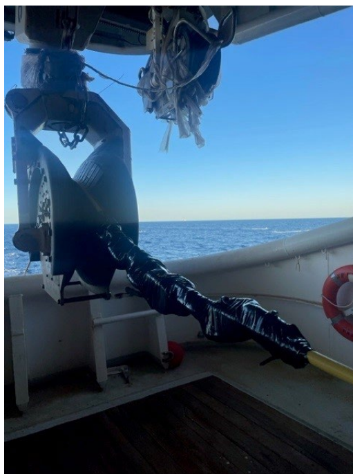
Figure 12. Cable guided through a fairlead block.
