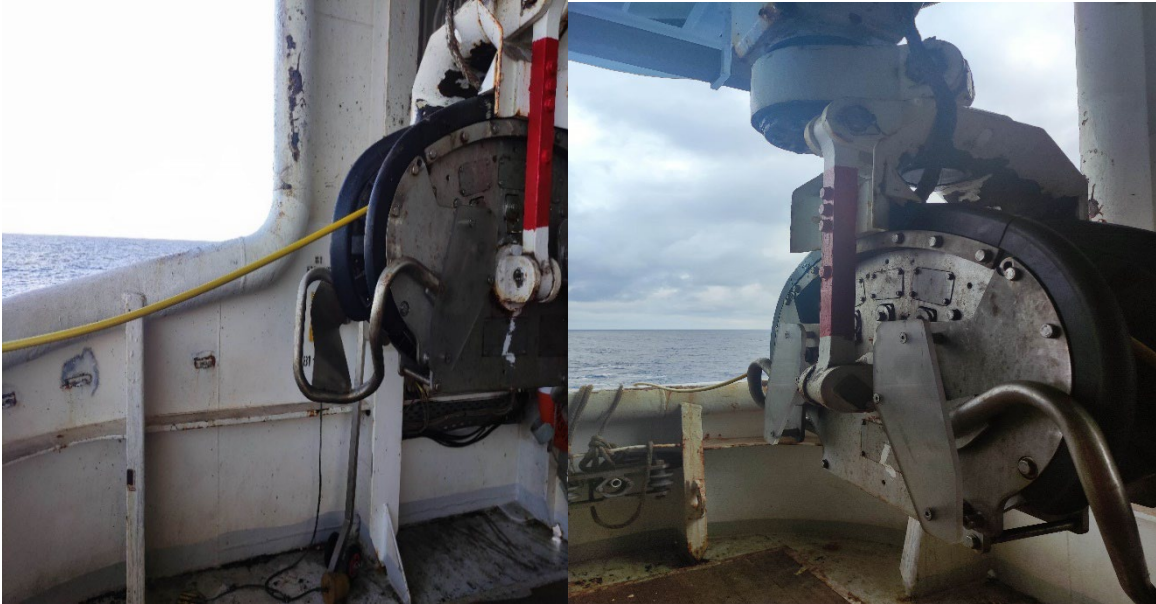
Figure 6. Cable guided through a fairlead block to the port stern of the vessel.
