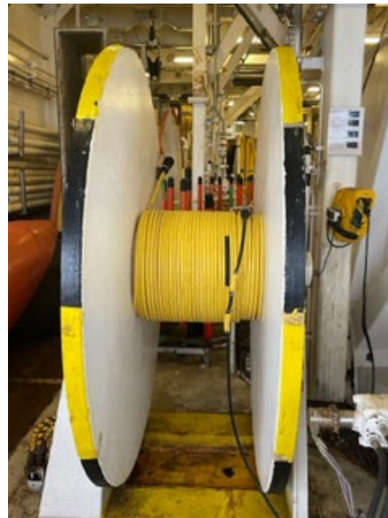
Figure 2. Hydrophone and tow cable on the hydraulic winch.
