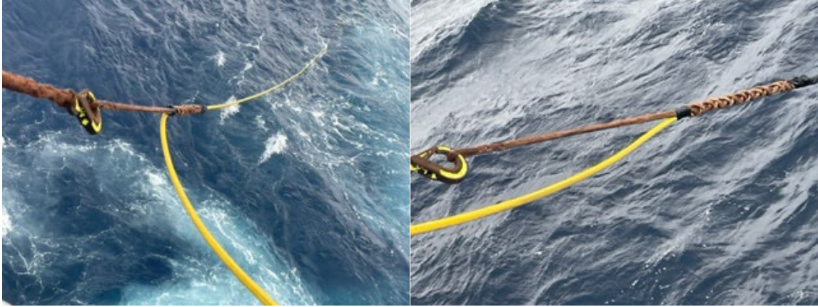
Figure 6-7. Chinese finger attached to the tow cable.
