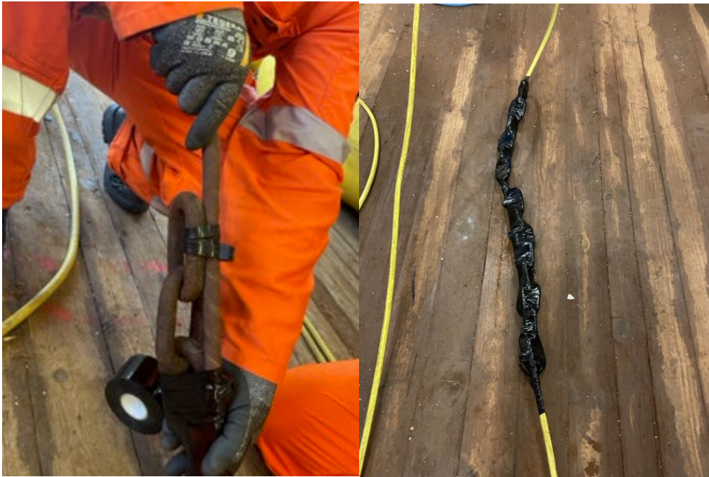
Figure 3-4. Weight added to the tow cable to increase depth.
