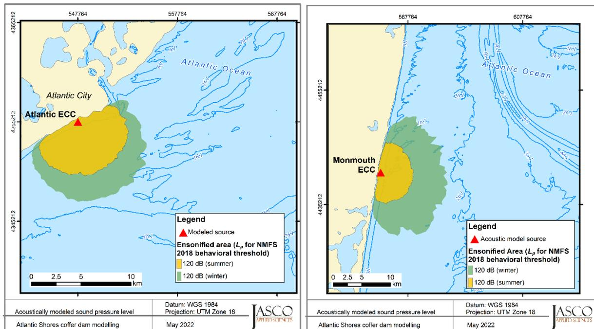
Figure 3. Modeled sound pressure level (SPL) at 120 dB re 1 µPa for two proposed cofferdam sites with sheet pile sources. The behavioral threshold for vibratory pile driving is SPL 120 dB re 1 µPa.
