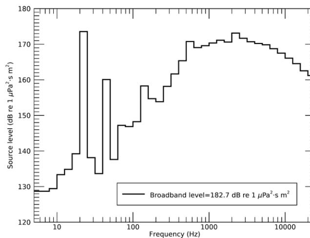
Figure 2. Decidecade-band spectral levels, at 10 m, for vibratory driving of sheet pile (Illingworth & Rodkin 2017).
