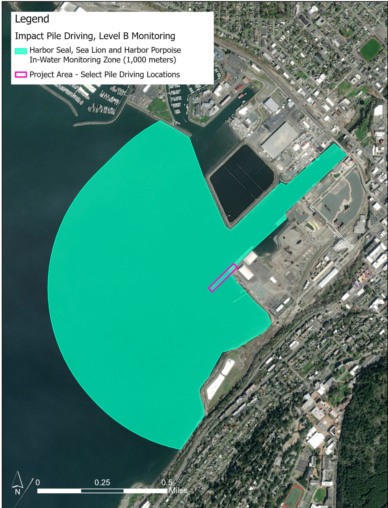
Figure 12. Impact Pile Driving, Level B Monitoring Zone
