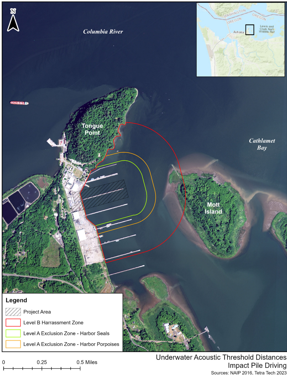
Figure 6-1. Underwater Acoustic Threshold Limits for Impact Pile Driving
