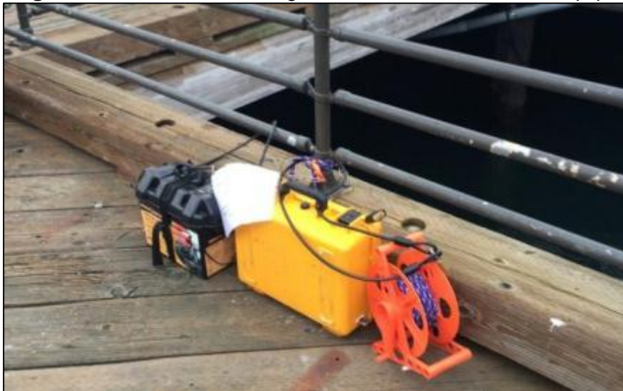
Figure 7.12 Near Shore Background Sound Measurement Equipment
