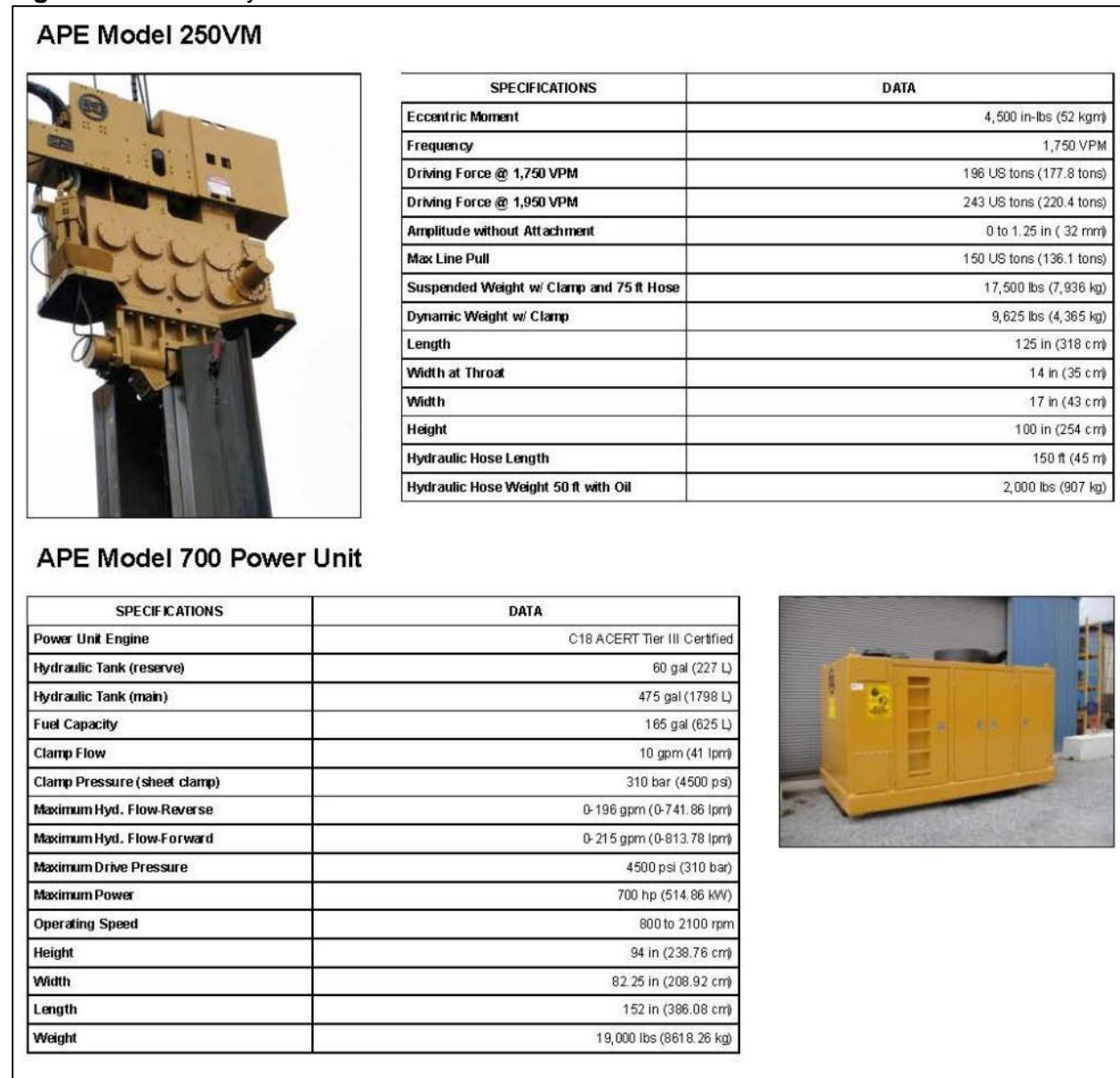
Figure 12.1 Vibratory Hammer Information
