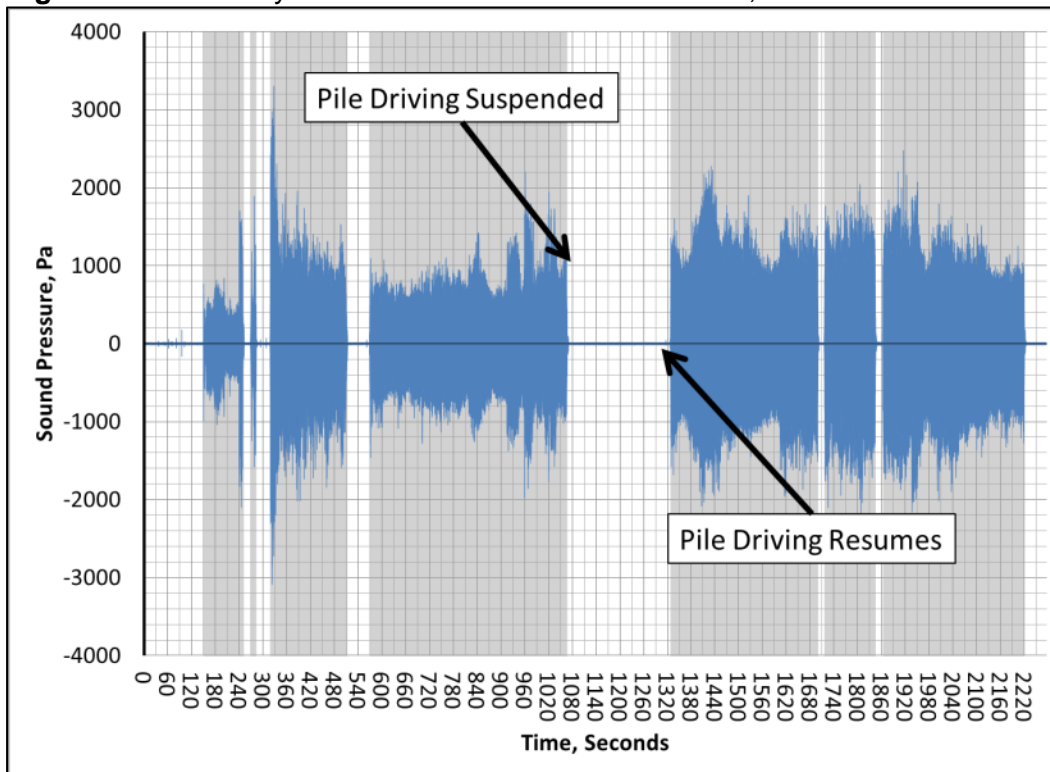
Figure 8.32 Vibratory Sheet Pile 5 Peak Sound Pressure, Pa
