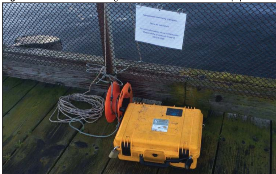
Figure 7.11 Near Shore Background Sound Measurement Equipment
