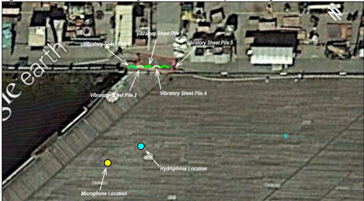
Figure 8.2 Sheet Pile and Monitoring Locations for Vibratory Pile Driving
