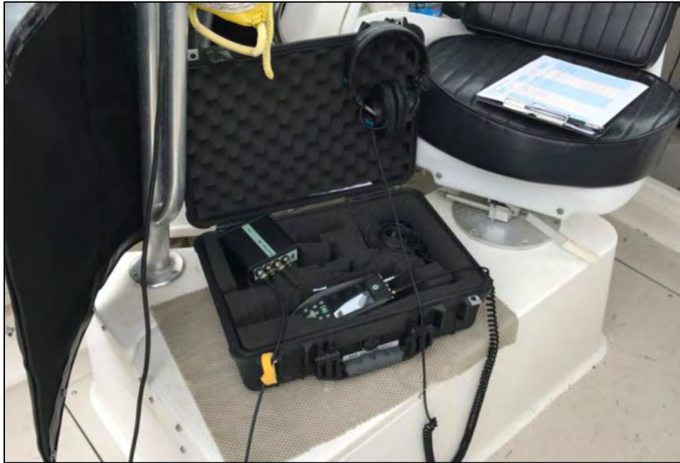
Figure 7.2 Far Field Background Sound Measurement Equipment
