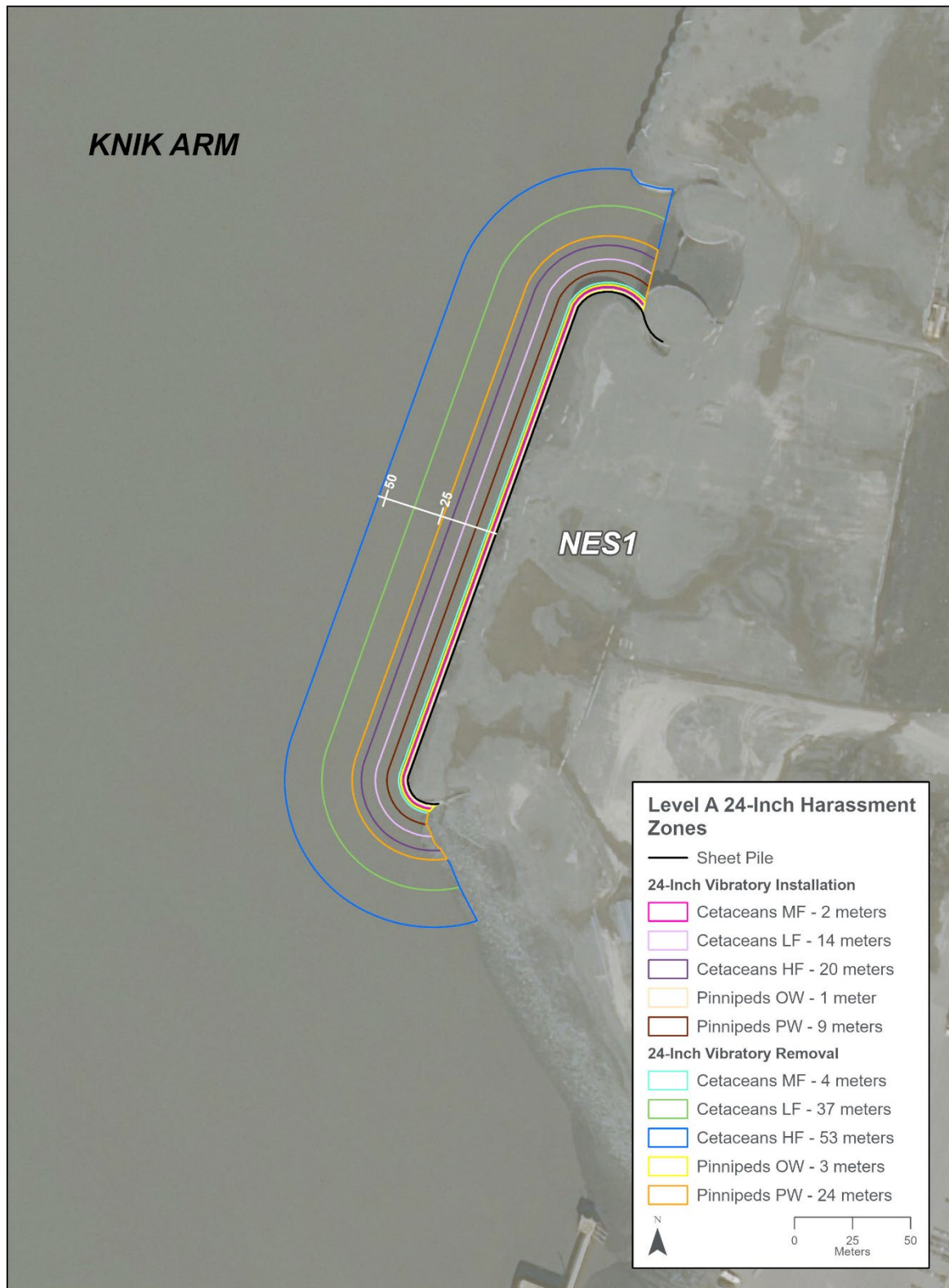
Figure 6-2. Level A Harassment Isopleths for Vibratory Installation and Removal of 24-Inch Piles
