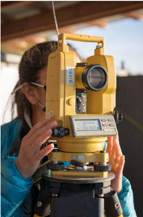
Photo 16. PSO using Topcon DT-205 digital theodolite (Photo Credit: Kristina Smolenski – The Photo Gecko)
