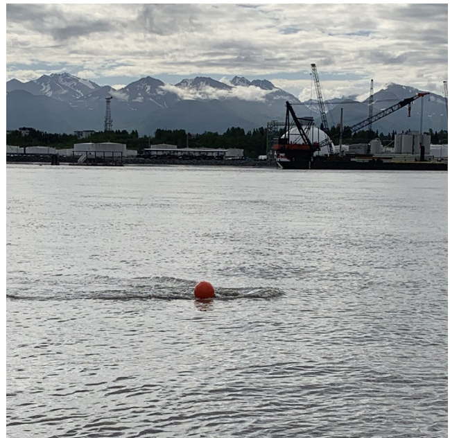
Mooring in current for hydrophone placed at approximately 800 meters from pile driving
