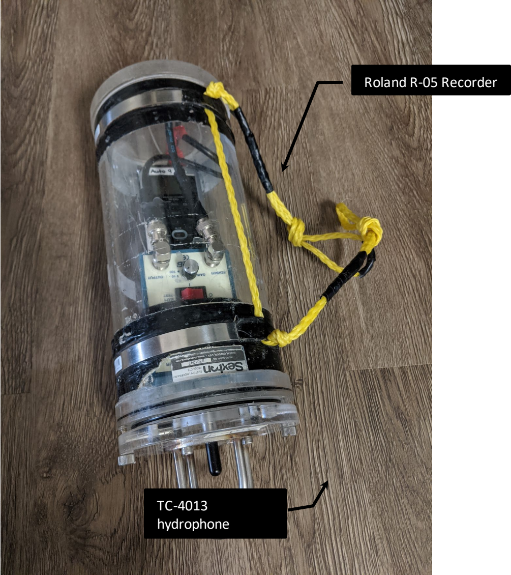
Figure 2-3. Autonomous units used at the close-in, SFD, and mooring positions
