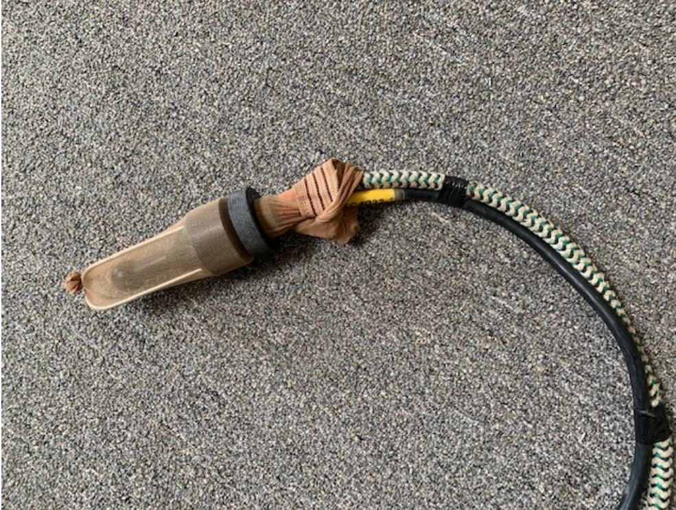
Figure 2-6. Example of hydrophone flow shield
