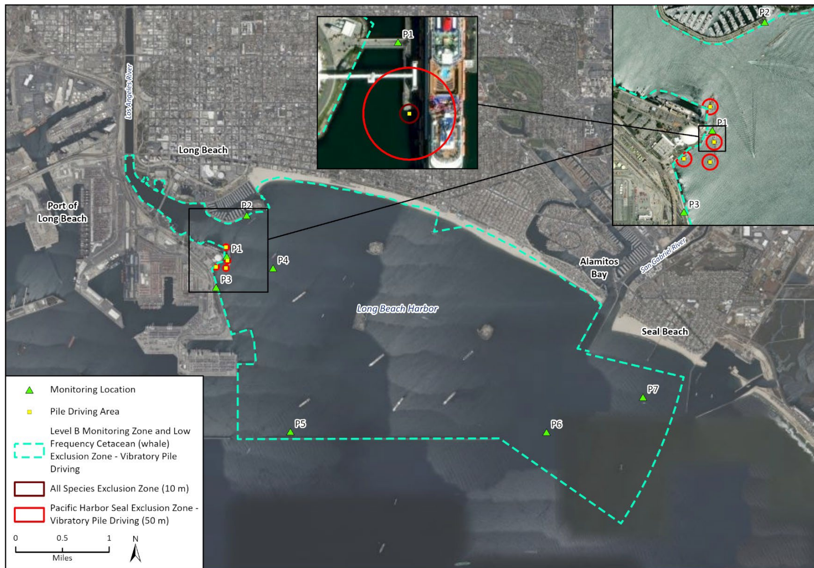
Figure 3 Monitoring and Exclusion Zones for Vibratory Pile Driving.
