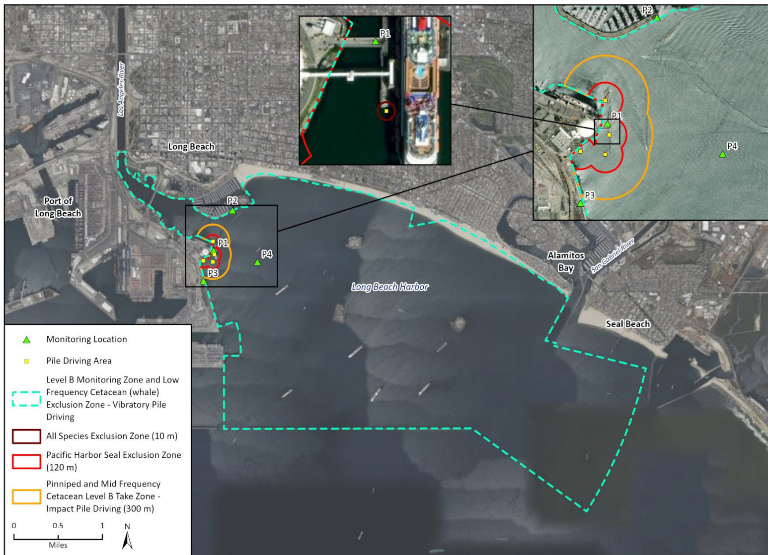
Figure 4 Monitoring and Exclusion Zones for Impact Pile Driving.
