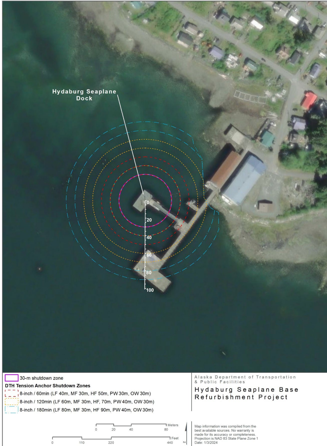
Figure 2-3. Representative Shutdown Zones during DTH Tension Anchor Installation
