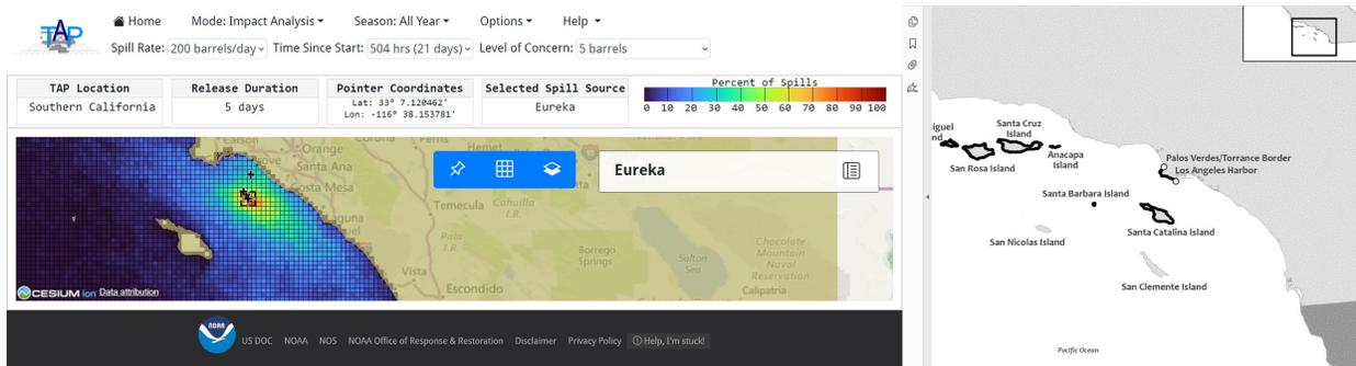
**Figure A-11. Modeled spill trajectory results for an accidental spill from Platform Eureka in the Beta Unit (left panel) and black abalone critical habitat, risk to Palos Verdes Peninsula, Santa Catalina and Santa Barbara Island (right panel).**
