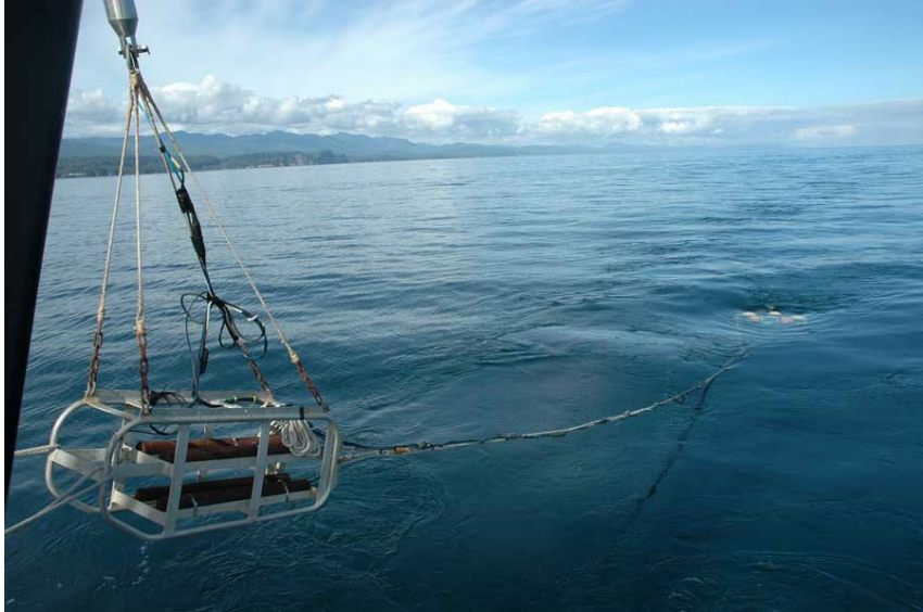
Figure A-28 TACOS video system during deployment
