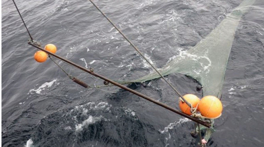
Figure A-8 Plumb staff beam trawl
