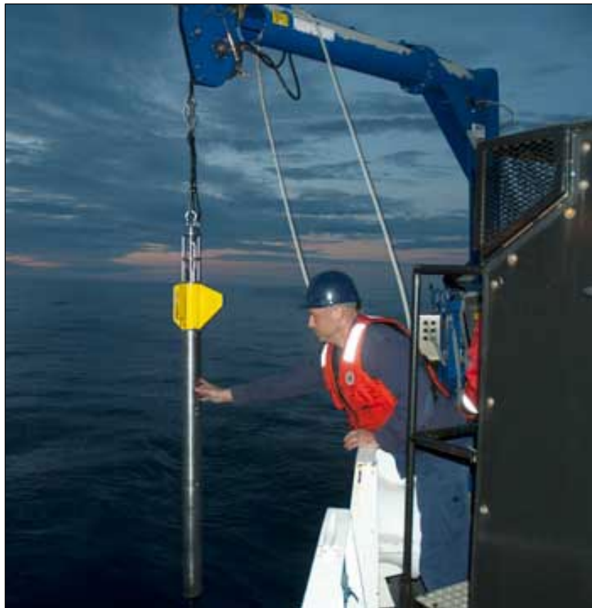
Figure A-23 Free Fall Cone Penetrometer
