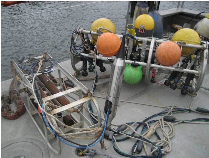
Figure A-27 TACOS video system with weighted sled
